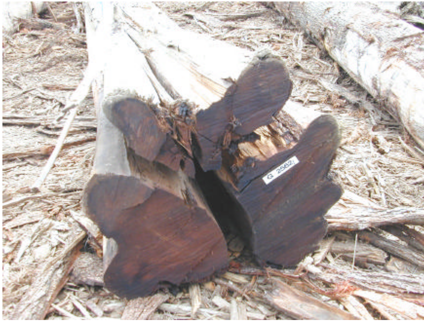
Plate 27: Quartering in a 'free' grown log which occurred during transport.
