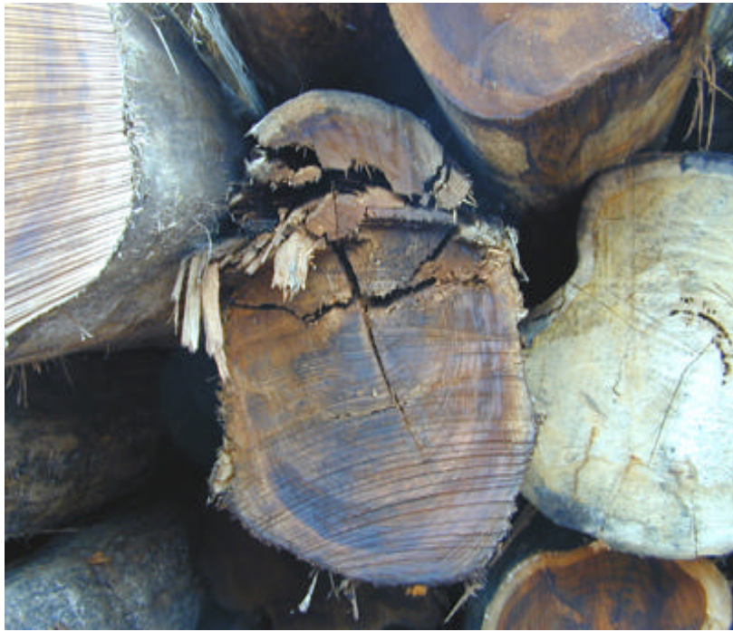
Plate 16: Capping visible at cut surface caused by forcing tree.
