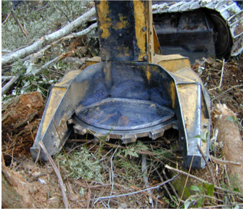
Plate 7: Disc saw utilised in Fixed Head.
