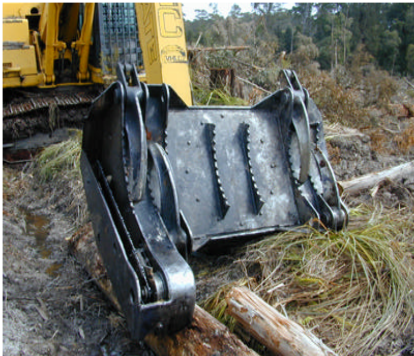
Plate 8: Chain saw utilised in rotatable Fixed Head.
