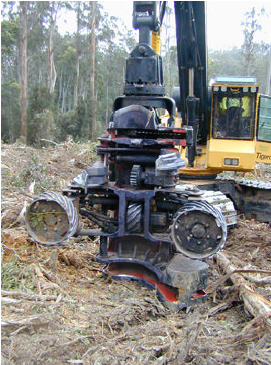
Plate 9: Live 'floppy' head showing grabs and feed rollers for debarking.
