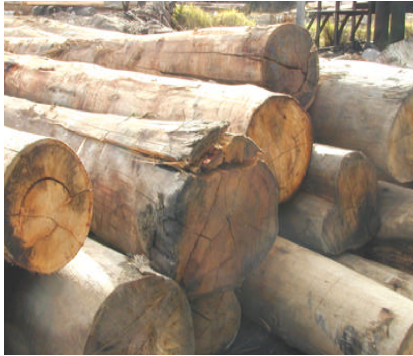
Plate 18: Slabbing and end-splitting caused by forces during felling.
