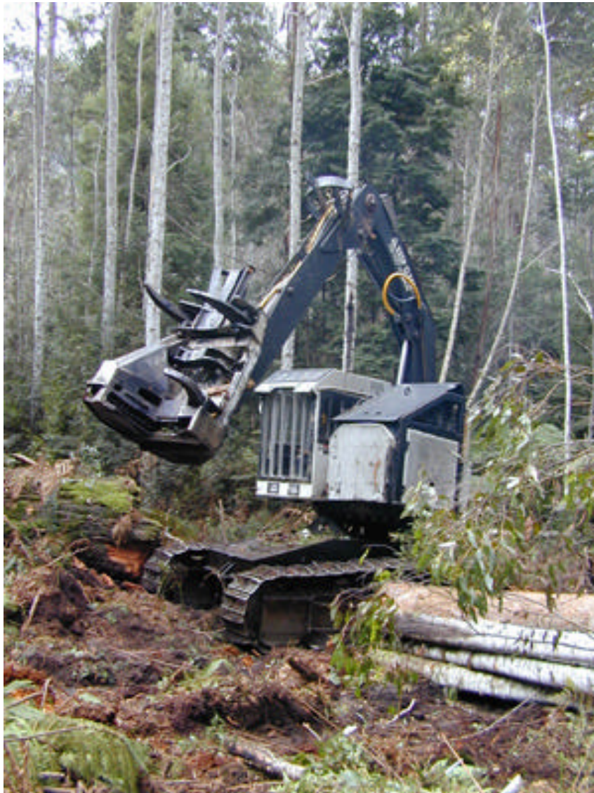
Plate 4: Purpose built carrier and fixed falling head.
