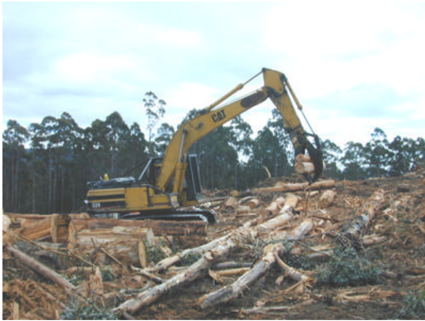
Plate 14: Crab grabs used for log sorting and loading.
