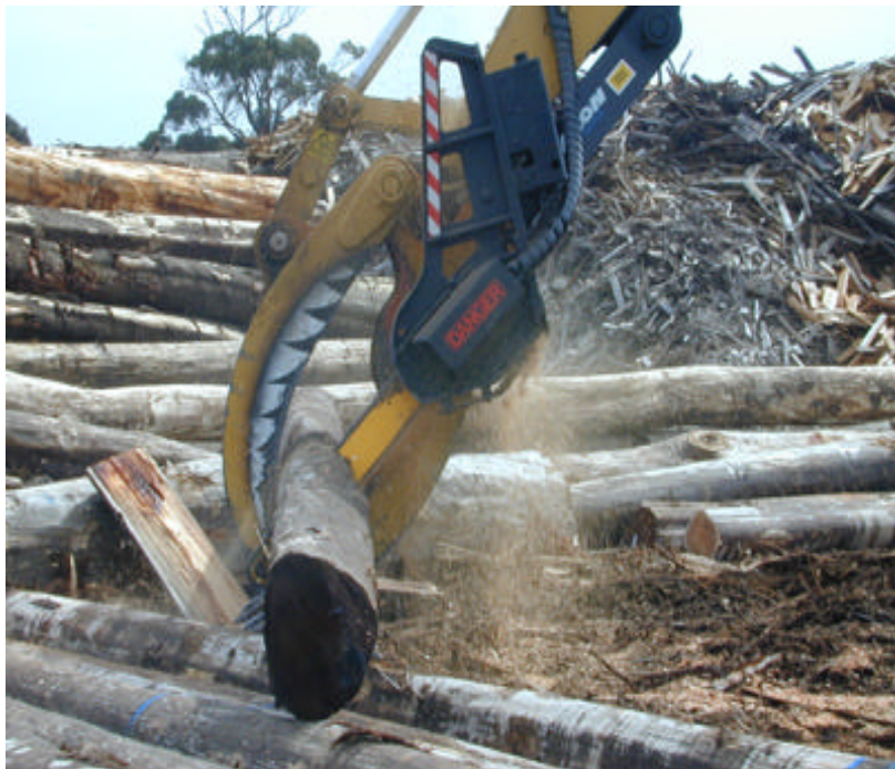
Plate 13: Cut-off saw for log presentation at landing.
