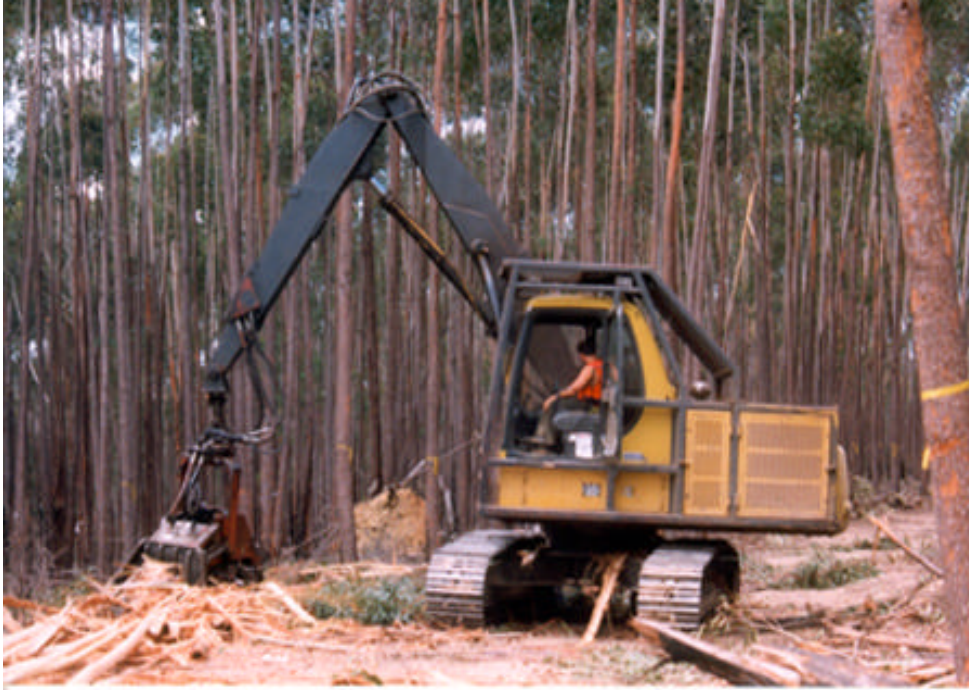
Plate 5: Excavator based ‘floppy’ or live felling head.
