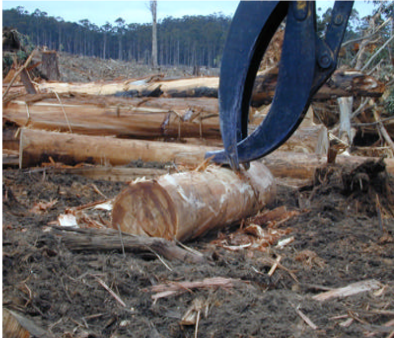
Plate 10: Debarking using crab grab attachment.
