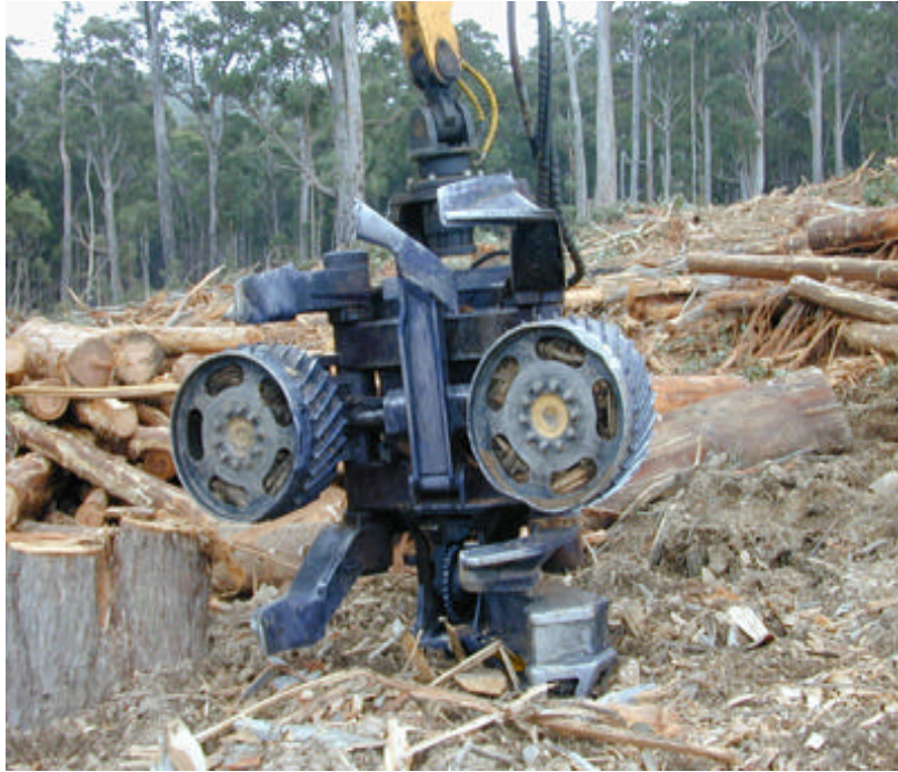
Plate 12: Debarking head with delimiting arms.
