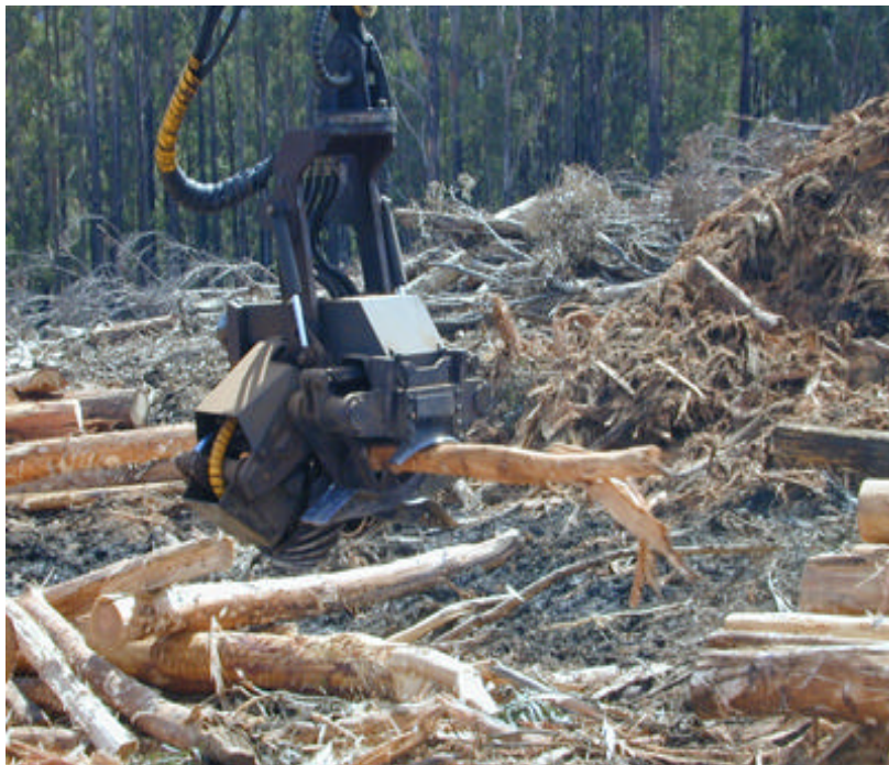
Plate 11: Debarking head used at landing.
