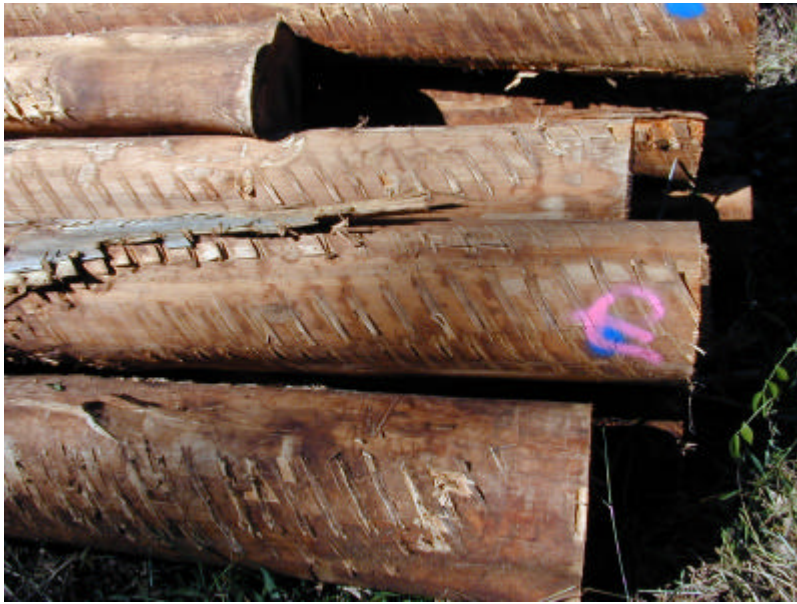
Plate 22: Machine marks and 'dog ears' caused by processing (debarking).
