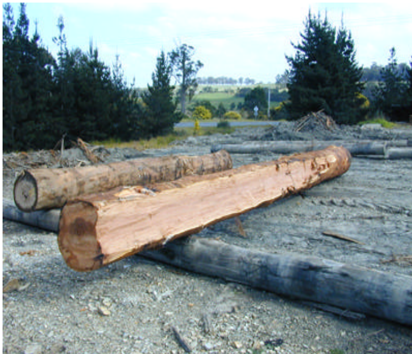
Plate 19: Slabbing in butt log through forcing the tree.
