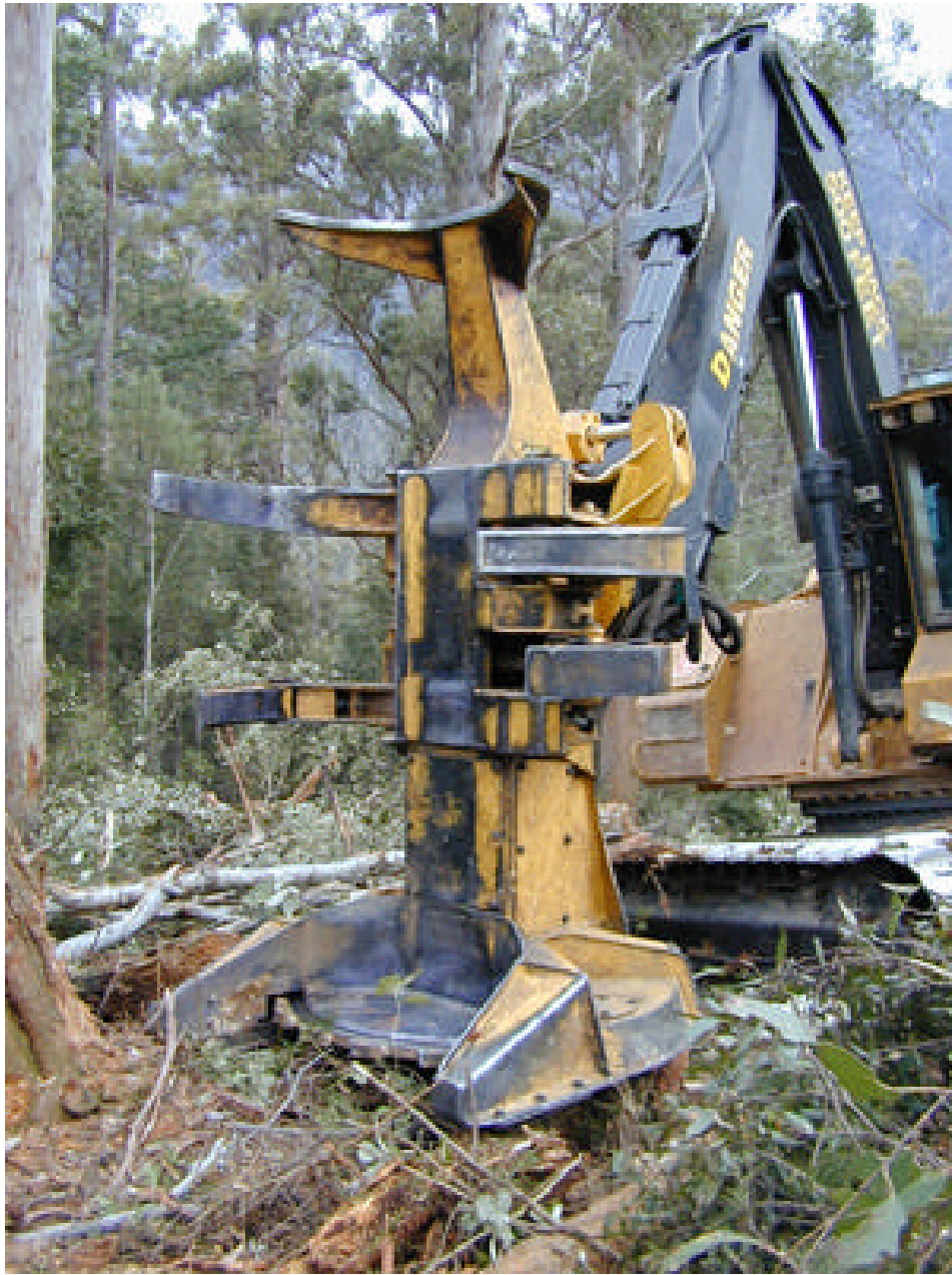
Plate 6: Fixed head used for directional falling.
