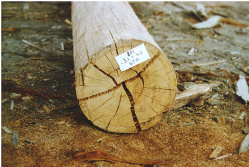
Plate 26: End splitting and shake in a small 'free' grown log.
