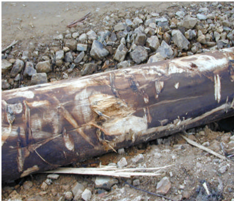
Plate 21: Shatter in a fallen log from striking an obstacle (stump?) which has translated into protrusions during debarking.
