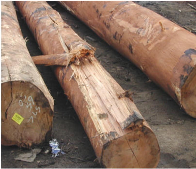
Plate 25: Slabbing caused by a single cut to unsupported log during bucking (subsequent handling has exacerbated the damage).
