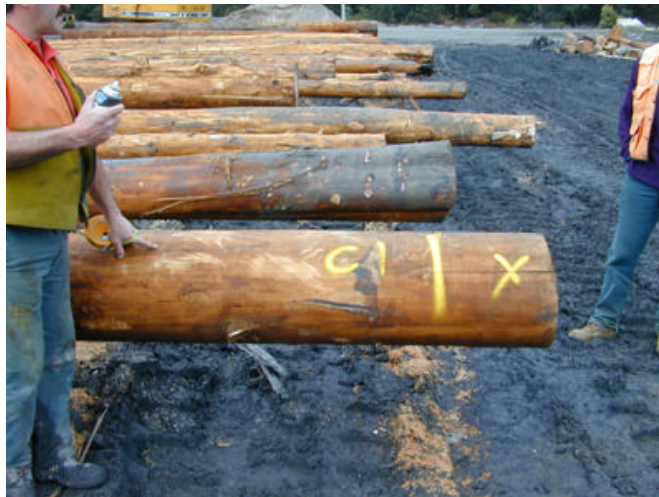
Plate 28: Yardsman identified lost volume (about to be docked) due to damage.
