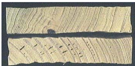
Figure 4. Corrugated (‘wash-boarding’) typical of collapse surface. Lower board shows internal checking in the earlywood of some growth rings
