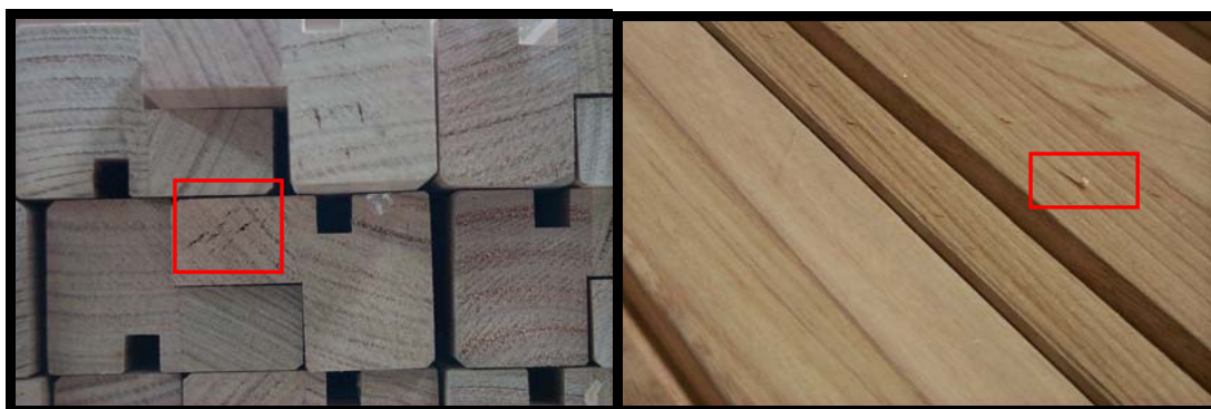
Figure 1. Internal checking in kiln dried Mountain ash window components (left) and lifting grain on dressed kiln dried Mountain ash (right).
