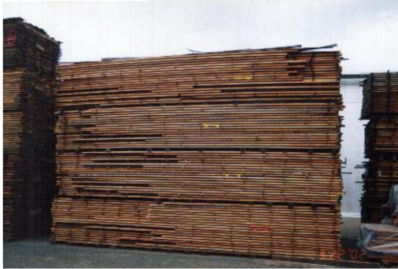
Figure 2.5 - Completed stack ready for air-drying
