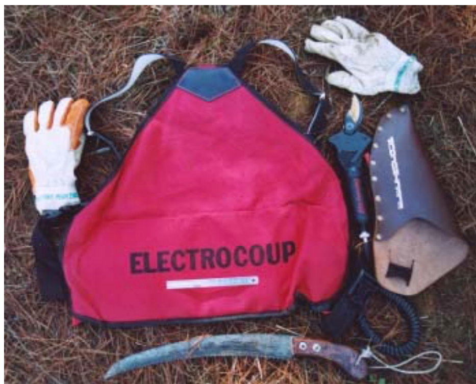
Figure 5. Photo of the Electrocoup hand piece, battery, safety gloves, holster and hand saw.
