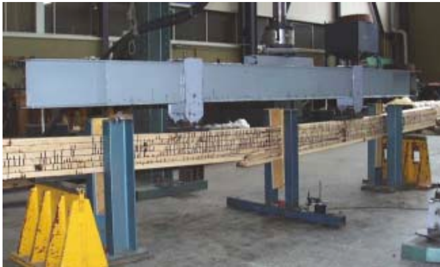
Figure 3 Arrangement used to measure MOR/MOE of glulam members
