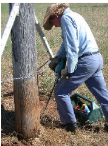
Figure 9. Several 500 mm long holes were drilled into poles 150 mm from ground level.
