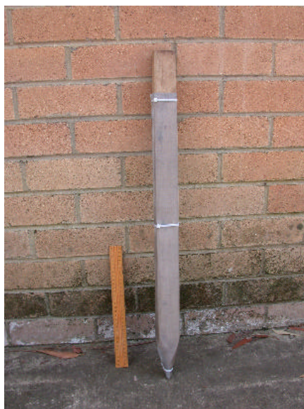
Figure 15. Post with stainless steel mesh barrier installed.
