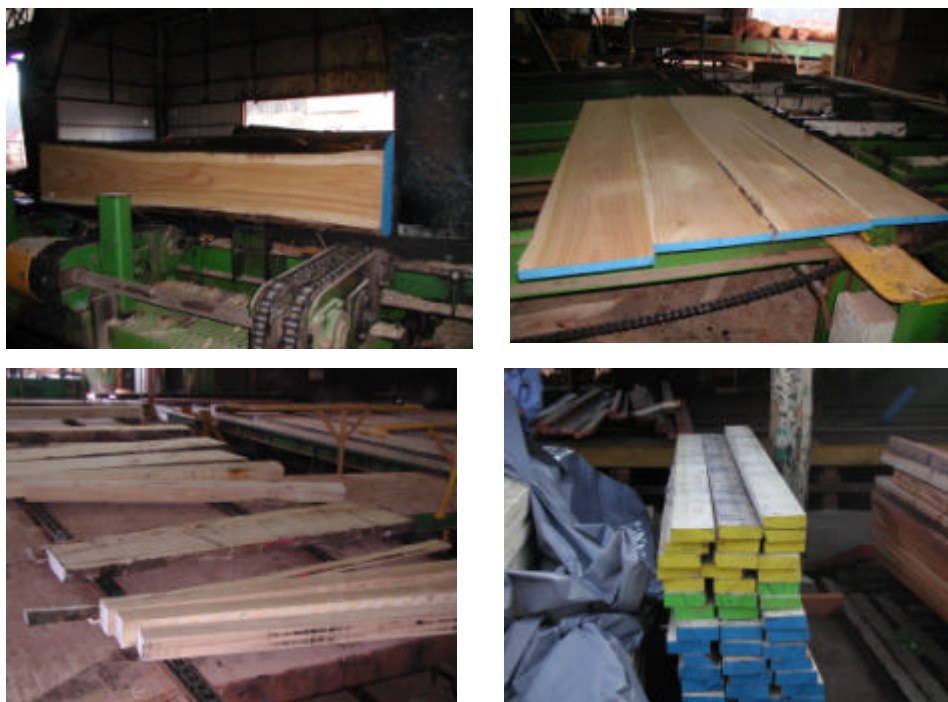
Figure 3. Back-sawing and quarter-sawing strategies used at the Auswest Timbers Pemberton mill (viewed from the small end); (a) back-sawing log break-down on the McKee twin saw; (b) quarter-sawing log break down on the twin saw; and, (c) quarter-sawing resawing strategy.
