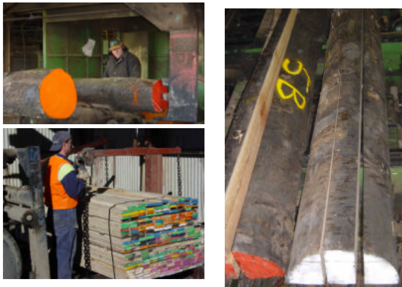
Figure 6. Sawing the unpruned E. globulus at Black Forest Timbers. Clockwise from top left; end dogging on the twin edger; quarter-sawn flitches for resawing; treating Lyctid susceptible sapwood.
