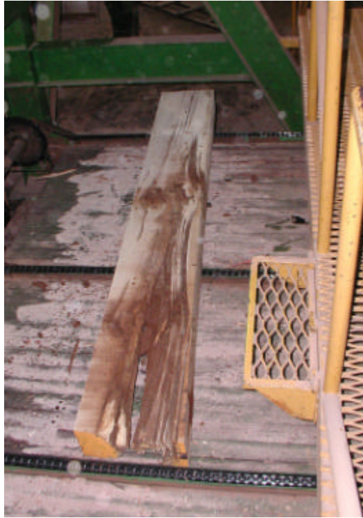
Figure 12. Termite damage in a cant that fell from the carriage at the completion of break down on the twin saw at the Auswest Timbers Pemberton mill.
