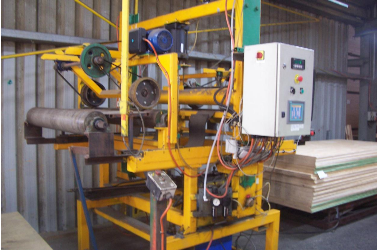
Figure 14: Plywood machine stress grader.
