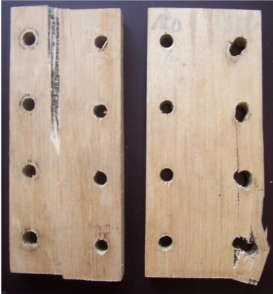
Figure 13: Plywood shear test specimens after test.
