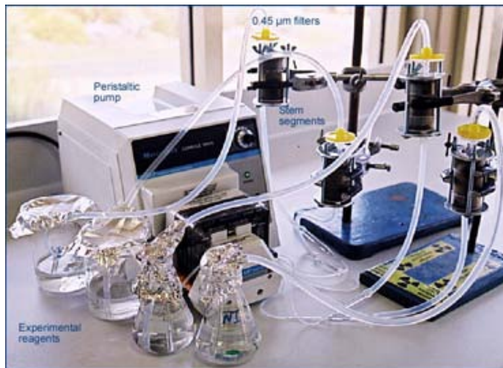
Figure 8 Components of the continuous flow in vitro system
