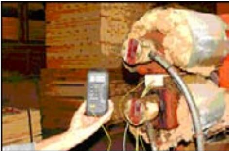
**Figure 1. Digital Temperature Meter and Thermocouples.**
