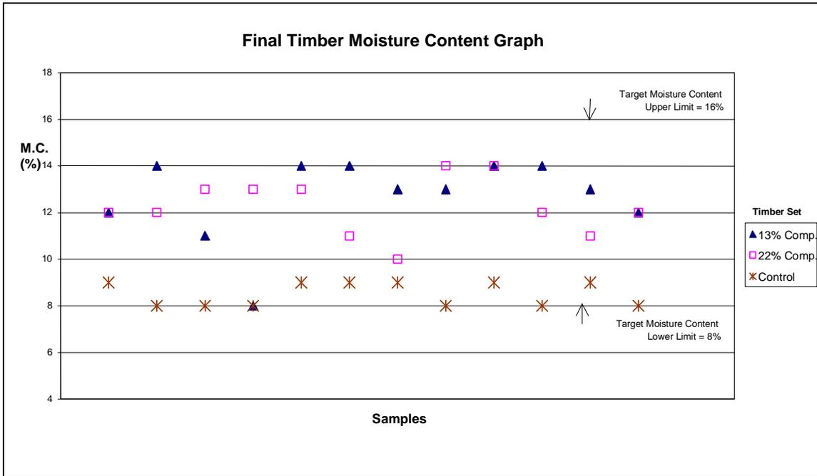
Figure 14. Final timber moisture content of timber samples.
