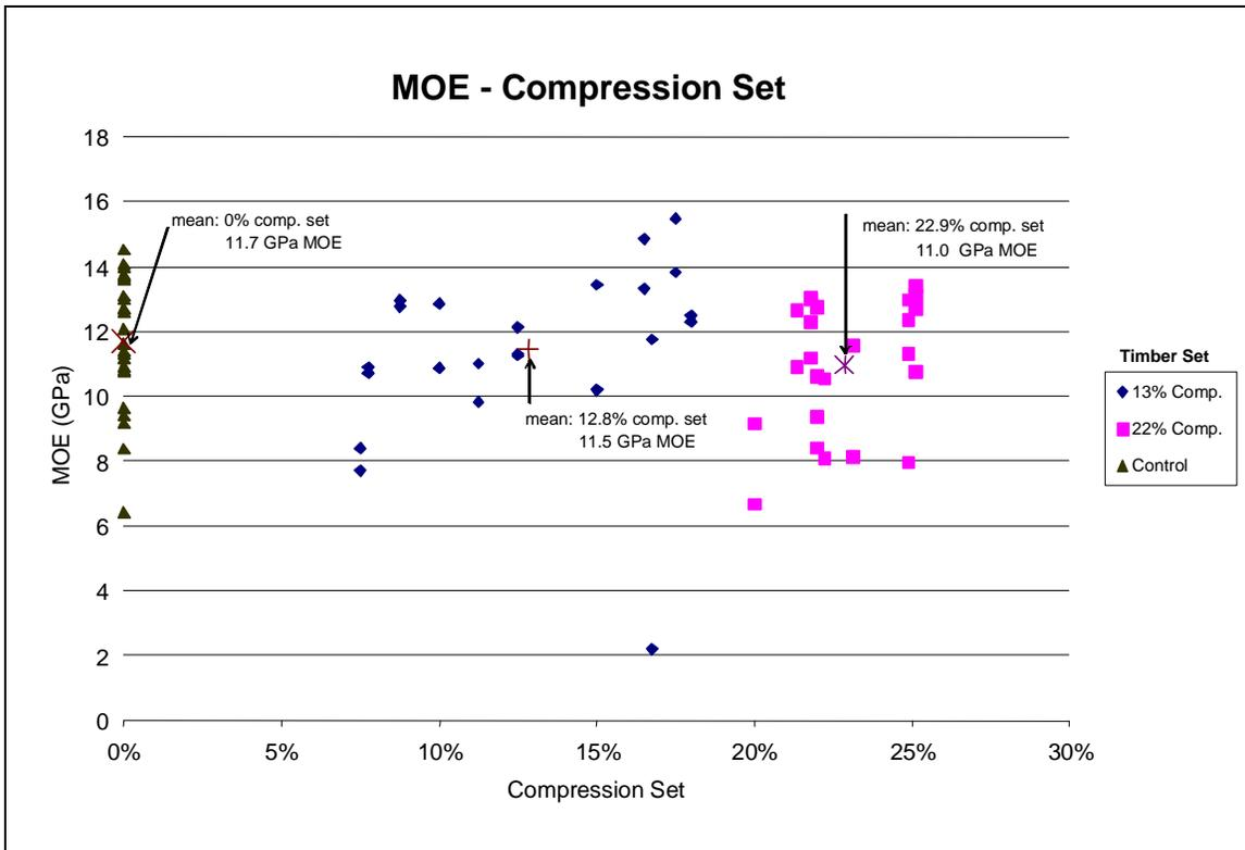
**Figure 18. MOE of the 620 mm long timber samples tested facewise compared to compression set, or the compression retained by the timber sample.**
