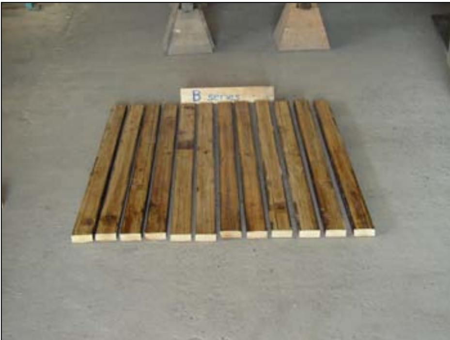
**Figure 13. B Series: 45 mm initial thickness timber representing 22 % nominal densification.**
