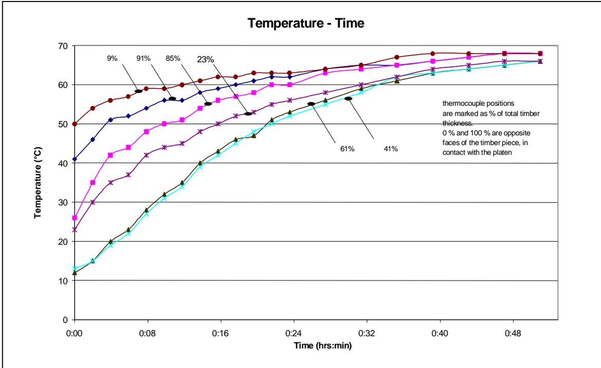
**Figure 2. Timber temperature response during the Experiment 1 pressing procedure at different distances from the platen contact face.**
