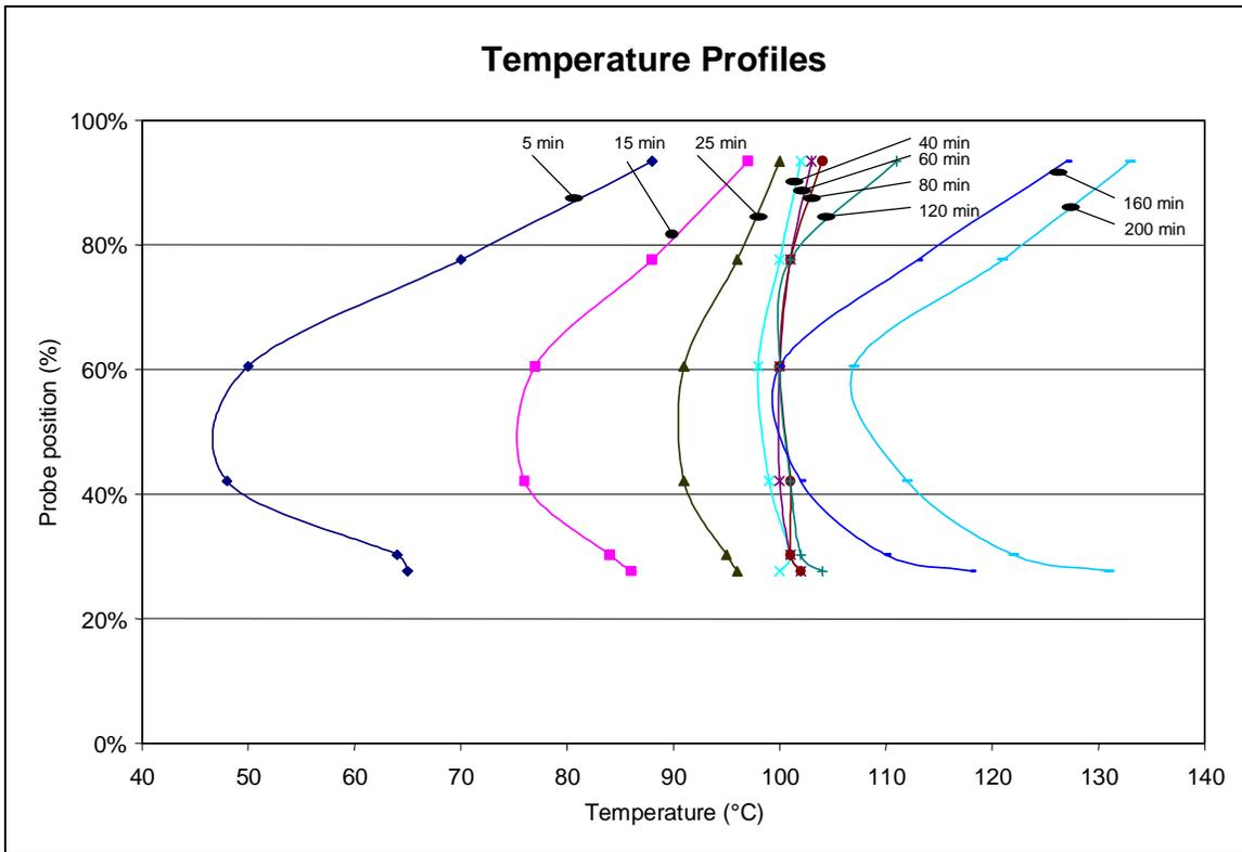
**Figure 6. Timber temperature response through the timber cross section at discrete time intervals during the Experiment 3 press procedure.**
