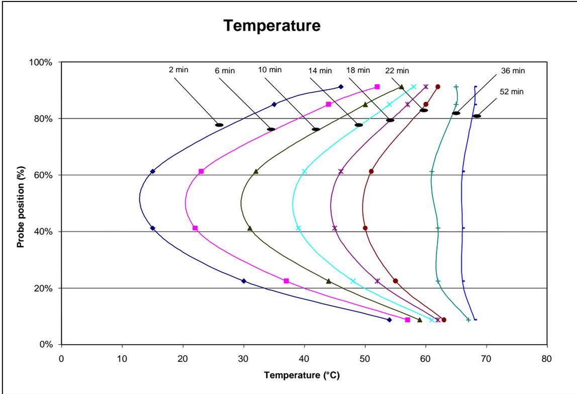
**Figure 3. Timber temperature response through the timber cross section at discrete time intervals during the Experiment 1 press procedure.**
