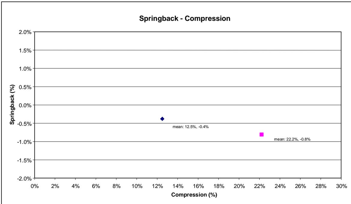
**Figure 16. Springback, or the recovery of the timber sample, compared to the total compression applied over the pressing procedure.**
