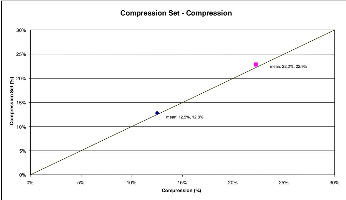
**Figure 15. Compression set, or compression retained by the timber sample, compared to the total compression applied over the pressing procedure.**
