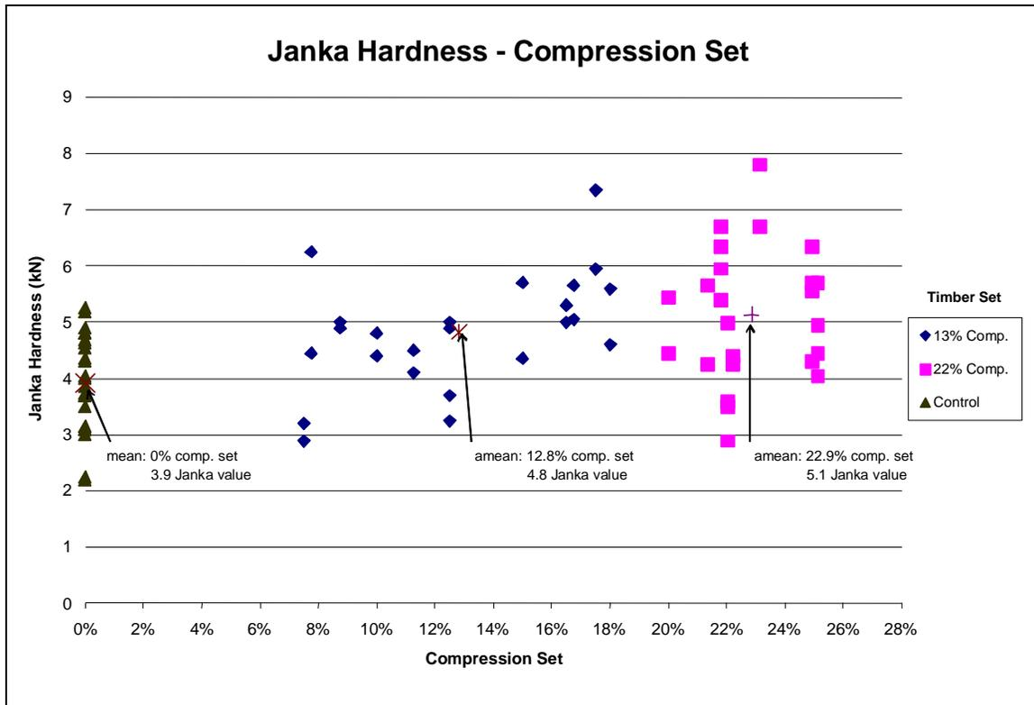
**Figure 20. Janka hardness for timber samples tested on the timber face in contact with the platen compared to compression set, or the compression retained by the timber sample.**
