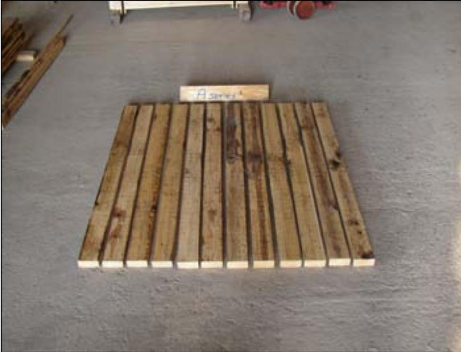
**Figure 12. A Series: 40 mm initial thickness timber representing 13 % nominal densification.**
