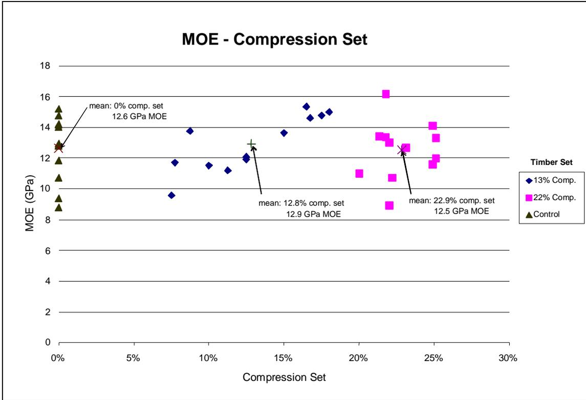
**Figure 17. MOE of the 1240 mm long timber samples tested edgewise compared to the compression set of the timber sample.**
