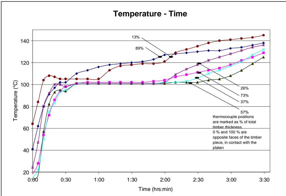
**Figure 7. Timber temperature response during the Experiment 4 pressing procedure at different distances from the platen contact face.**
