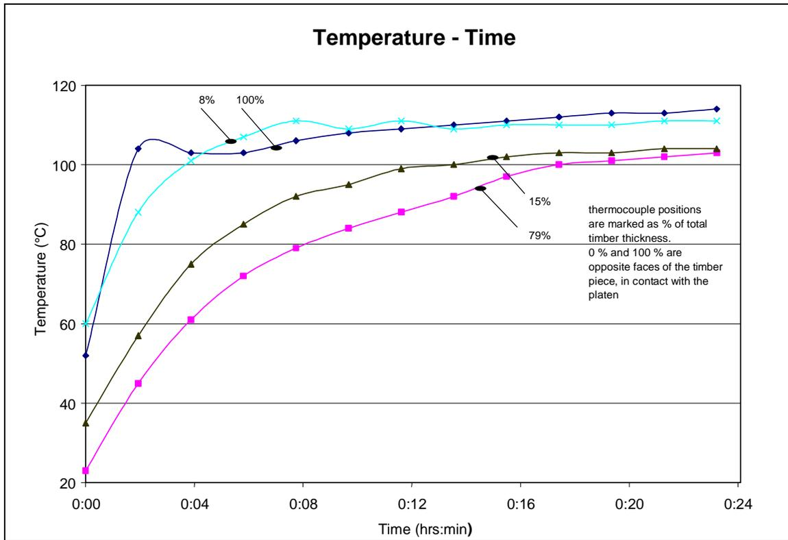
**Figure 4. Timber temperature response during the Experiment 2 pressing procedure at different distances from the platen contact face.**
