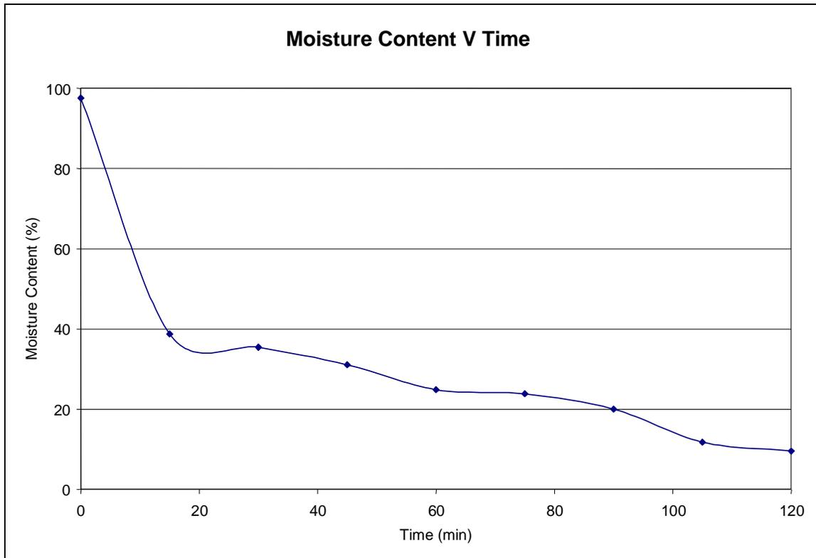
**Figure 9. Variation of timber moisture content through a typical pressing procedure.**
