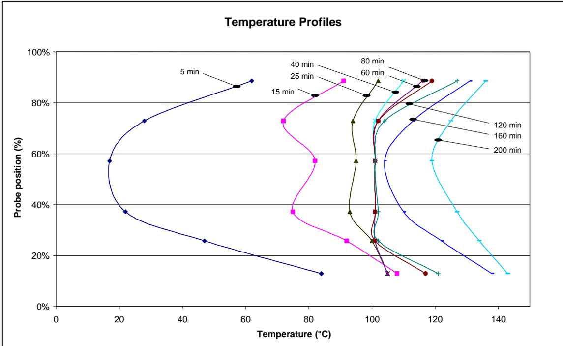
**Figure 8. Timber temperature response through the timber cross section at discrete time intervals during the Experiment 4 press procedure.**
