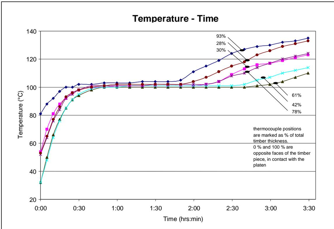
**Figure 5. Timber temperature response during the Experiment 3 pressing procedure at different distances from the platen contact face.**
