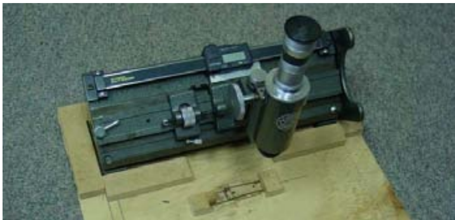
Figure 2.1.2. Apparatus for monitoring shrinkage of slices.
