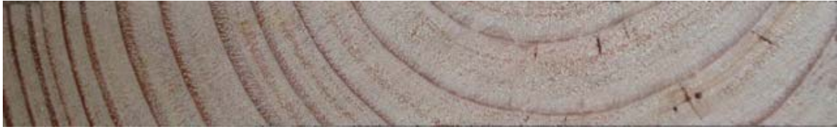
Figure 4.3.11. Victorian Ash board showing internal checking near heart only.
