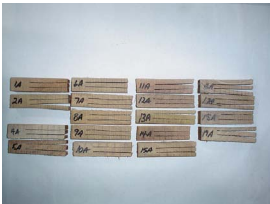
Plate 3. Stress prong test results immediately after cutting in Experiment 1
