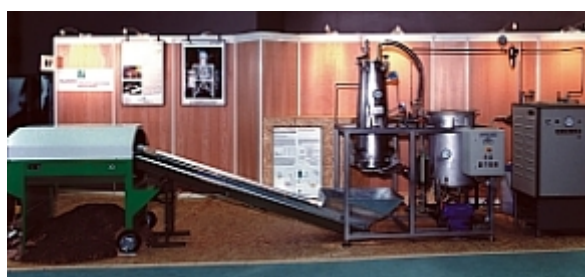
Figure 8.1. Picture of a pilot scale version of the WKI process.
