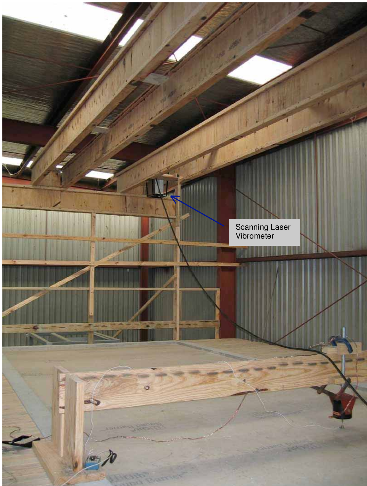
Figure 7-3. Overview of the shaker and the scanning laser vibrometer for measurement of floor vibration response. The scanning laser vibrometer is mounted on a gantry made from I-beams 2.6m above the floor. There are two gantries to enable the whole upper surface of the floor to be scanned.
