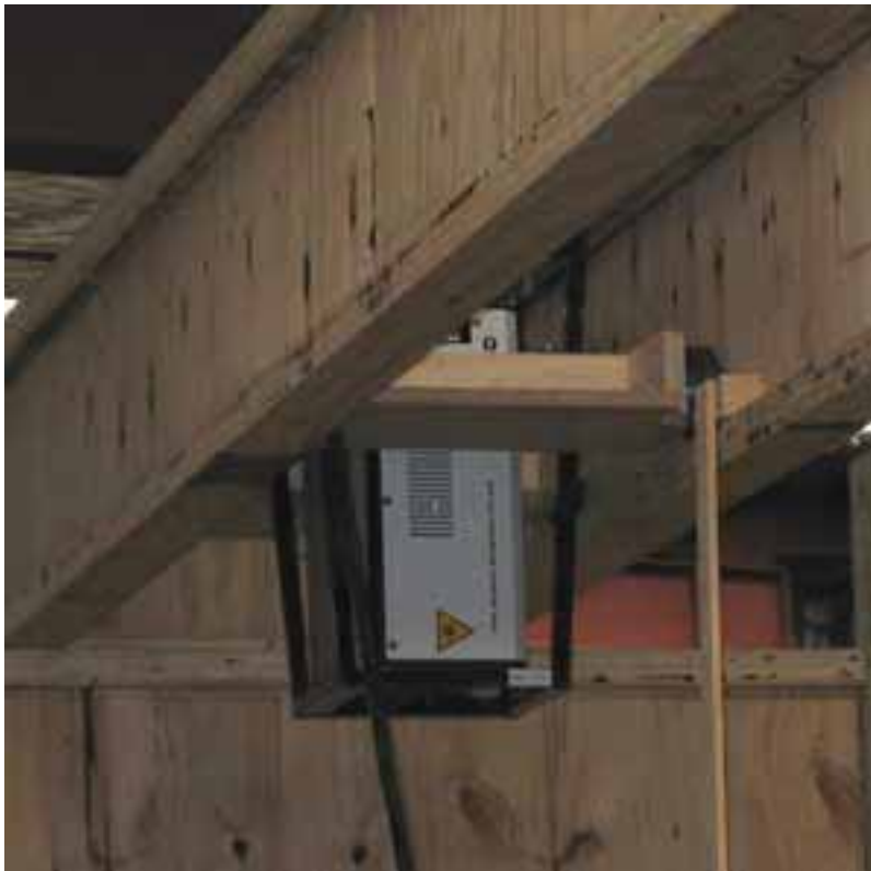
Figure 7-4. Close-up of the scanning laser vibrometer as supported in the gantry. The laser vibrometer is supported in a trolley, which can roll along the flanges of the I-beams, enabling the laser vibrometer to be moved to different sections of the floor.
