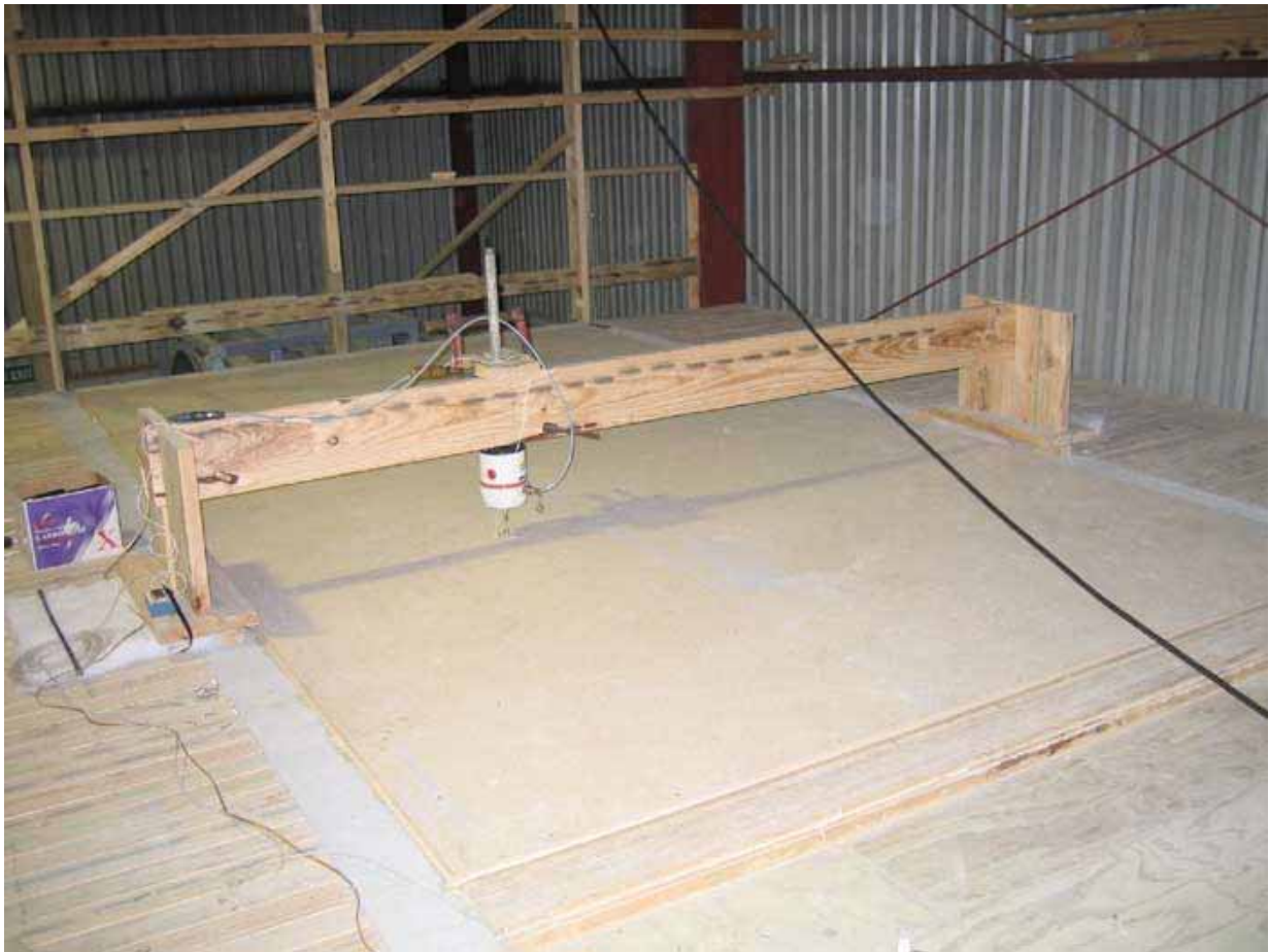
Figure 7-1. View of the shaker attached to a floor to send vibrations into the floor.
