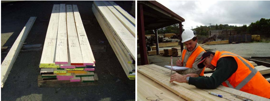
Figure 14. Board identification code on back-sawn boards and measurement of dimensions and spring and bow immediately after sawing
