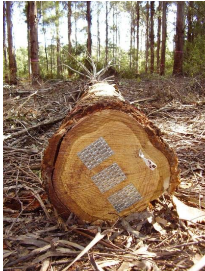
Figure 5. The felling cut after application of end-sealing compound with the gang nails and identity tag applied immediately after felling
