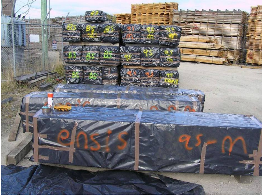
Figure 15. Boards packed and ready for transport to Launceston for drying at the University of Tasmania kilns and at NST Timbers in Mowbray
