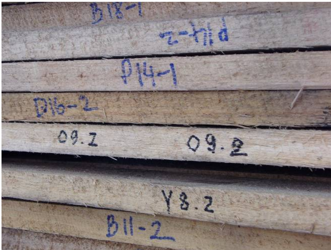
Figure 19. Board identification code transferred from the face to edges of boards
