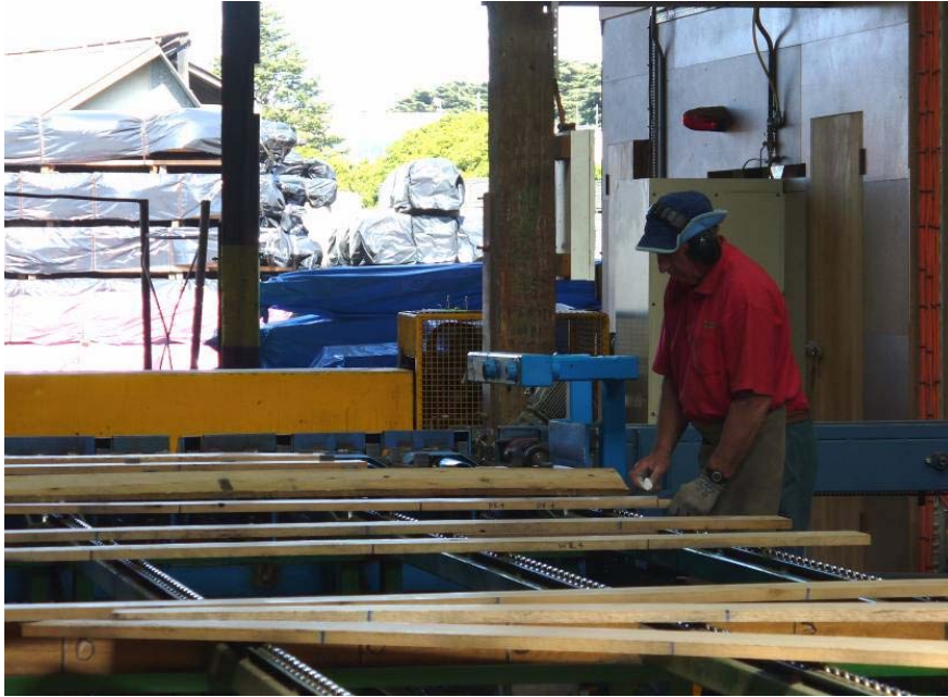
Figure 22. McKay Timbers staff grading boards
