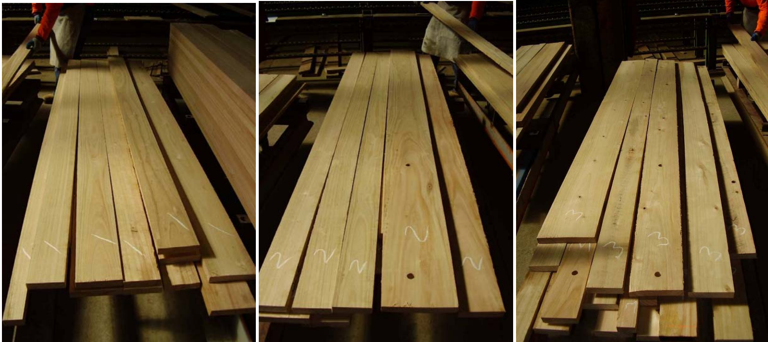
Figure 25. Select grade back-sawn boards (left), Standard grade back-sawn boards (centre) and Utility grade back-sawn boards (right)
