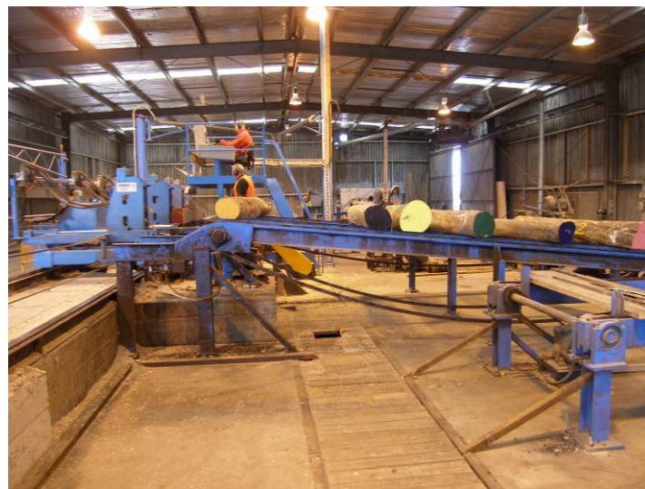
Figure 10. Back-sawing logs on the second break-down saw
