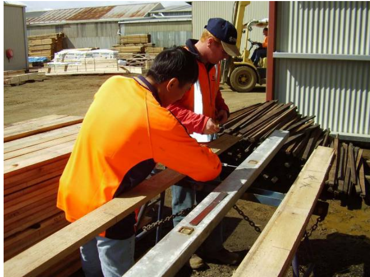
Figure 20. Measuring spring, bow, cupping, product dimensions and end split severity on the intensively measured boards before planning
