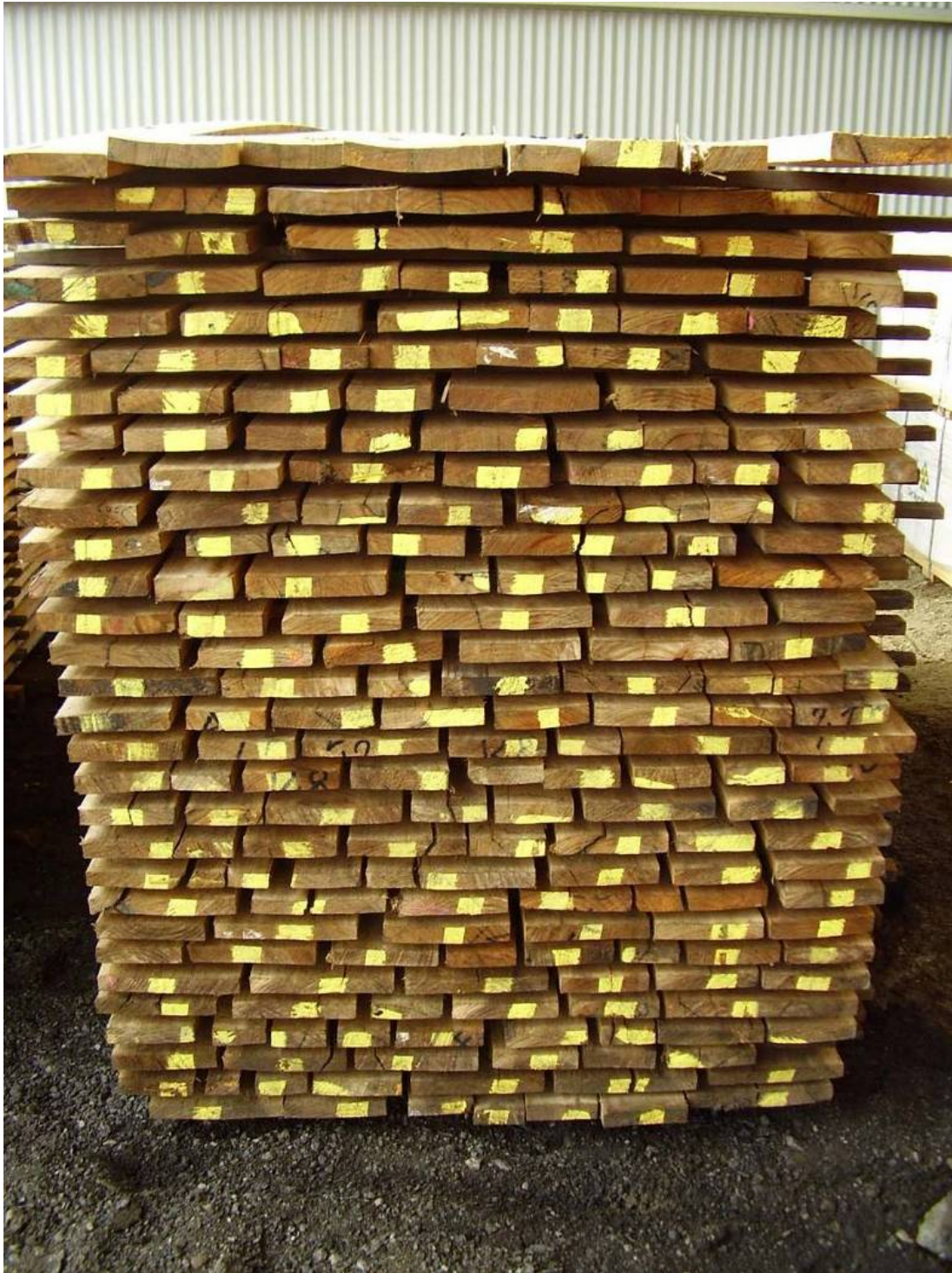
Figure 17. Dried back-sawn boards
