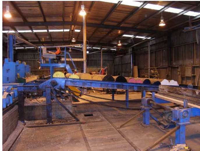
Figure 9. Quarter-sawing logs on the second break-down saw
