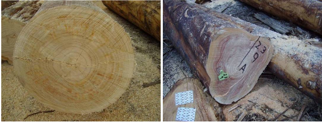
Figure 6. Log end splitting immediately after removal of discs (top) and transfer of log identity code to the freshly sawn face after collection of discs
