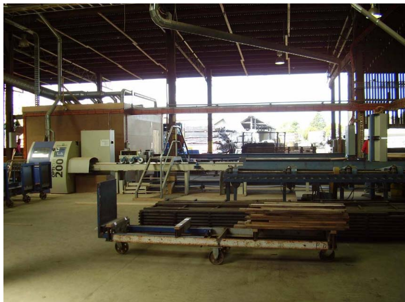
Figure 21. Opticut 200 planer used to skip dress boards on the face and back
