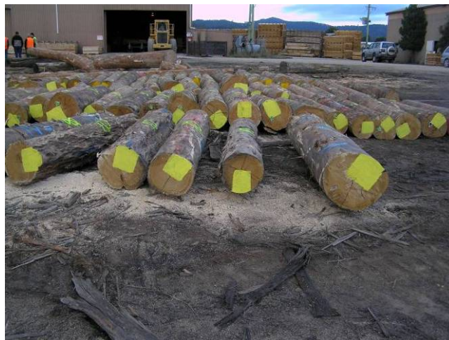
Figure 8. Colour codes on the log large end (top), and position of centre cant boards on back-sawn logs (centre) and the centre cant on quarter-sawn logs
