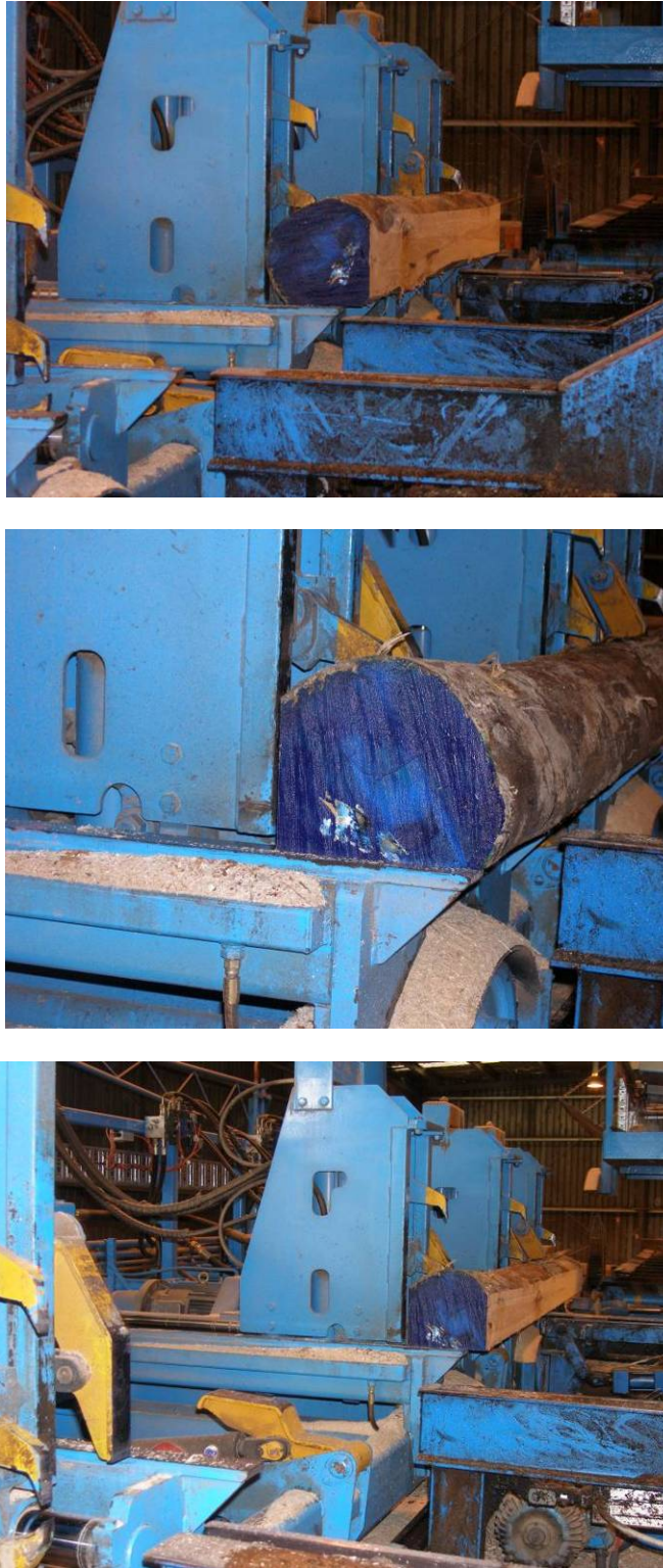
Figure 12. Log rotation sequence used for back-sawing. Note the end dog is unused in the 2.7 m logs
