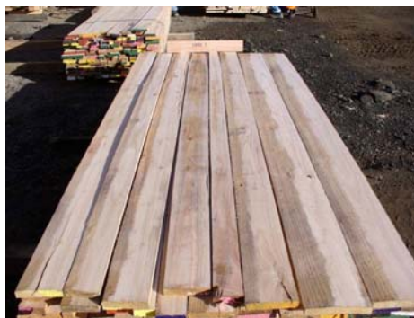
Figure 28. Undersized back-sawn and quarter-sawn boards down-graded to utility grade
