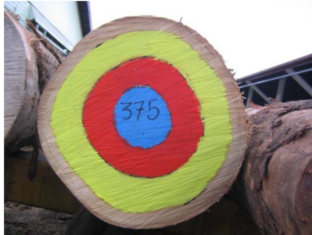
Figure 1 Typical allocation of inner (blue), intermediate (red) and outer (yellow) heartwood zones.
