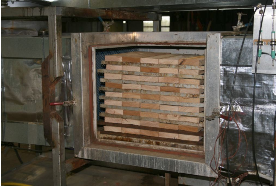
Plate 2 - Conventional kiln stack
