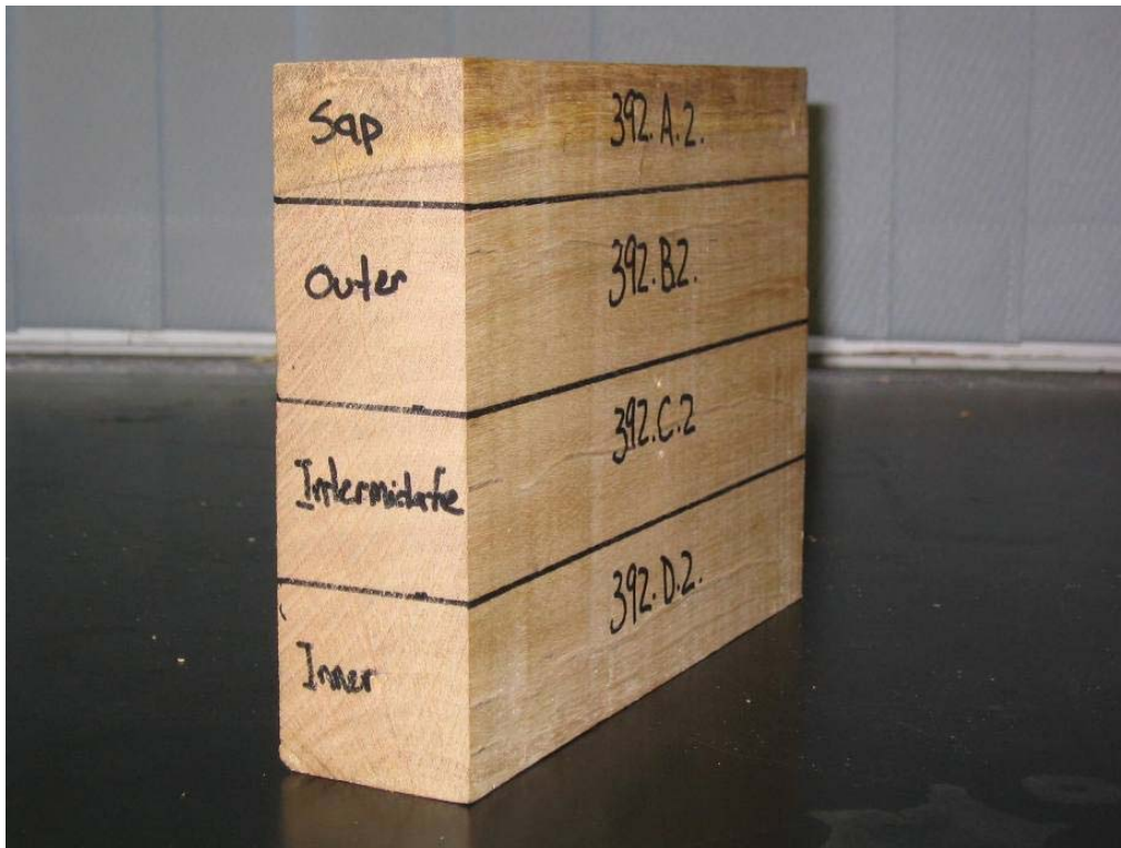
Plate 4. Hardness sample preparation enabled testing to be conducted on the inner, intermediate and outer heartwood and sapwood zones.
