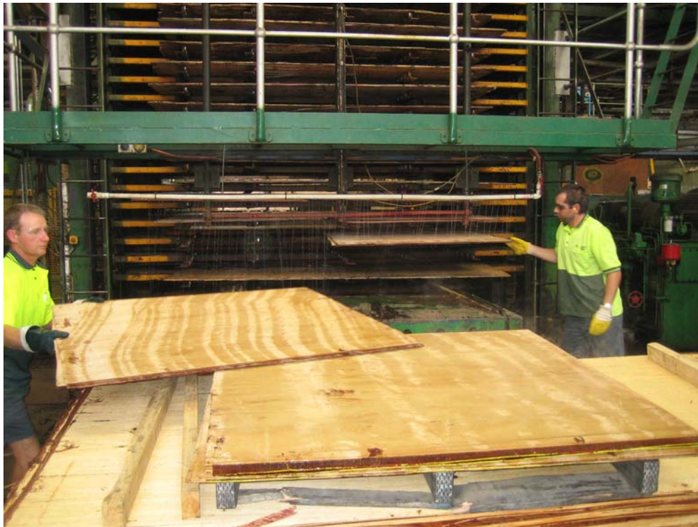
Plate 4. Manufactured plywood being removed from the hot press at Boral Hancock.
