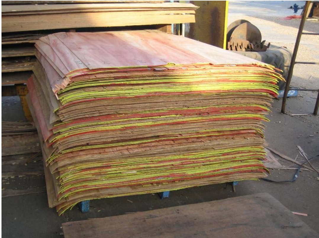
Plate 3. Veneer produced from peeling trials conducted at Big River Timbers.
