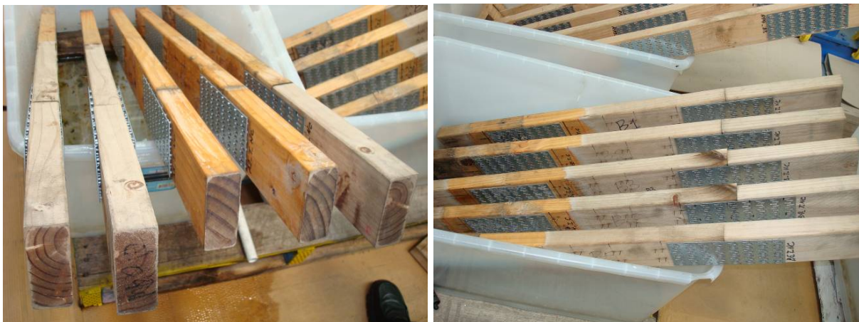
Figure 3.2 – Test specimens: left are plain finished with 5 joints non-coated and 5 coated with WB5000; right are reed finished with 5 joints non-coated and 5 coated with 660 Seal n Peel
