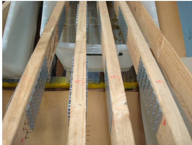
Figure 3.14 – Backout on quarter-sawn Radiata pine specimens
