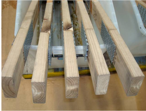
Figure 3.9 – Backout of non-coated joints in specimens B (reed finished).
