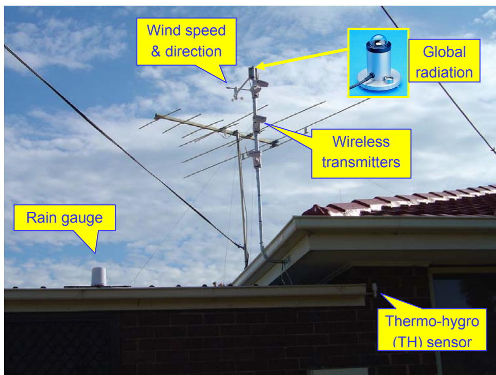
Figure 5.10 - Monitoring system for outdoor climate parameters, including air temperature & humidity, wind direction & speed, rain intensity and solar radiation
