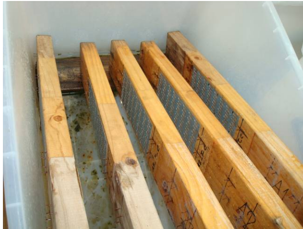
Figure 3.10 – Joints coated with 'Seal and Peel' WB5000. No backout observed.
