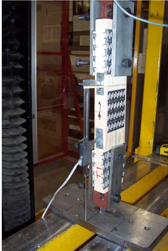
Figure 4.2 – Setup for short term capacity test
