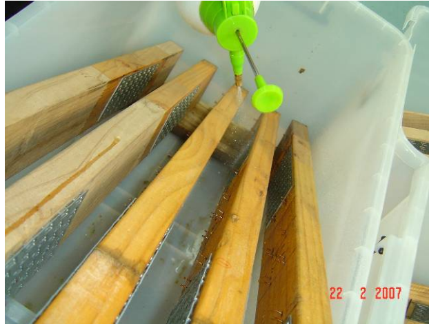
Figure 3.5 – Spraying water with a pre-pressurised spray bottle
