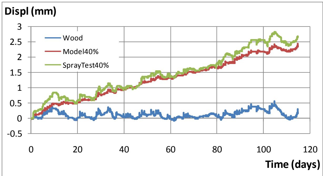
Figure 3.22 – Comparison of model prediction and spray test result for loading level of 40%.
