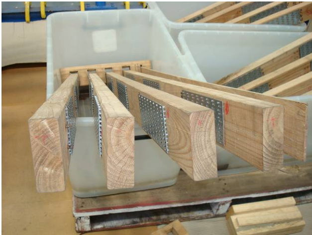
Figure 3.13 – Backout on back-sawn Radiata pine specimens
