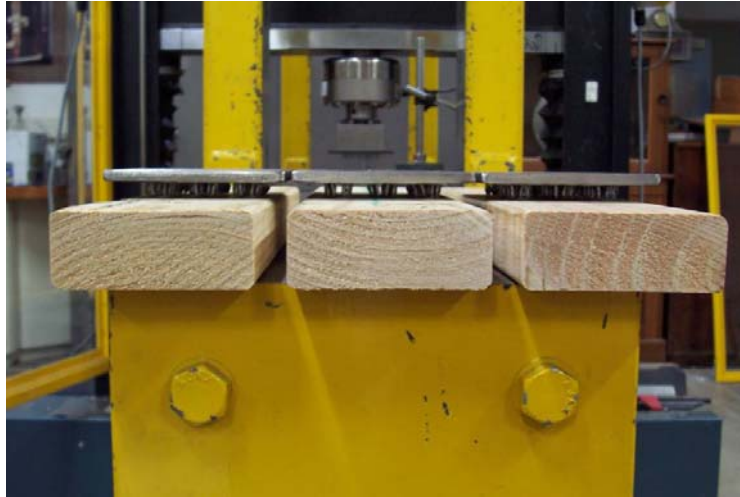
Figure 3.33 – Orientations of nailplate to timber – barkside (left), pithside (centre) and quartersawn (right)
