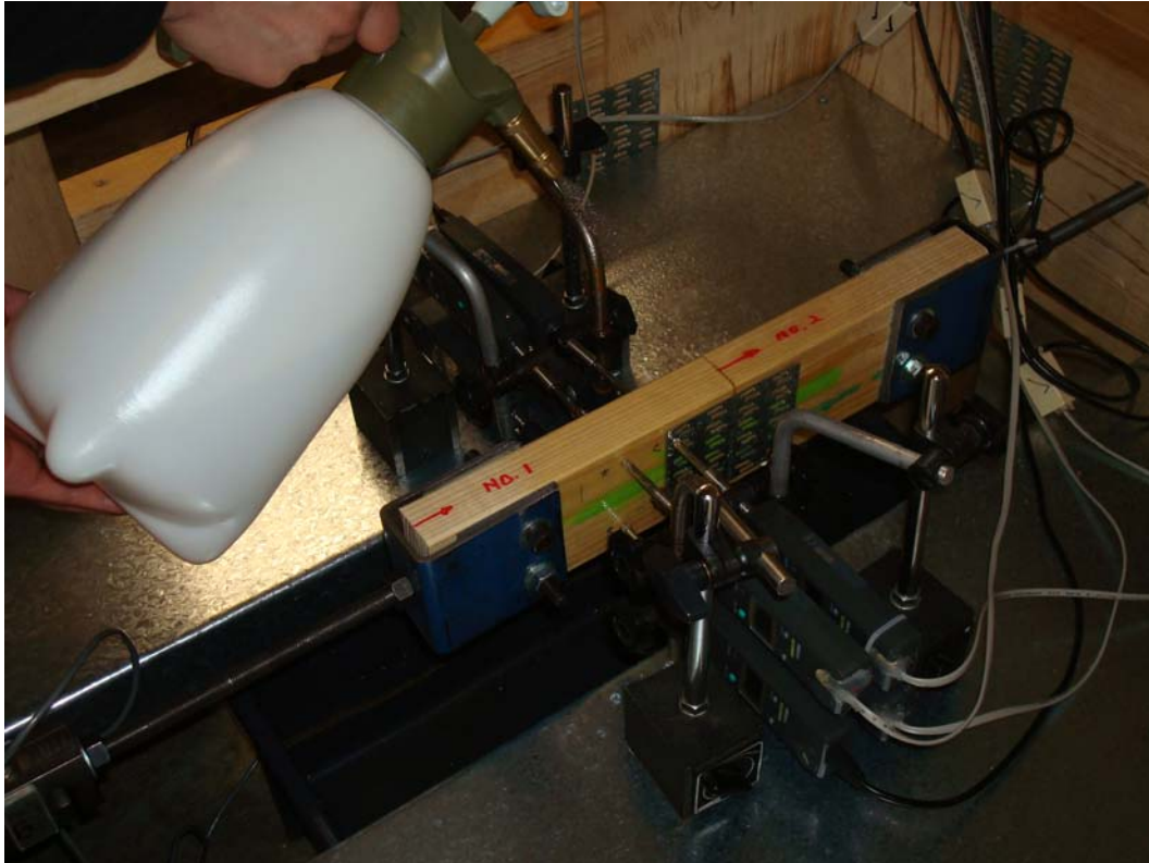
Figure 3.16 – Wetting of specimens using a pressurised spray bottle
