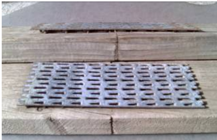
Figure 2.2 – Backout of nailplates exposed to the weather for 20 years
