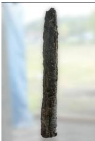
Figure 8 FireTard 120 CCA-treated spotted gum specimen four hours after testing at 60 kW/m 2 and being subjected to a 2 m/s wind
