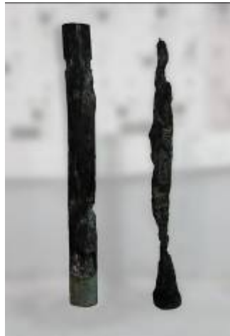
Figure 13 CCA-treated spotted gum specimens 24 hours after testing at 60 \text{ kW/m}^2 without subsequent 2 m/s wind exposure (L) and with subsequent 2 m/s wind exposure (R)
