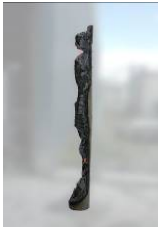
Figure 4 CCA-treated spotted gum specimen four hours after testing at 60 kW/m 2 and being subjected to a 2 m/s wind
