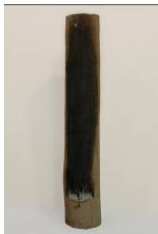
Figure 21 FireGuard CCA-treated radiata pine specimen four hours after AS 1530.8.1 test start
