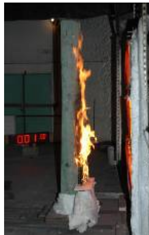
Figure 3 CCA-treated spotted gum specimen one minute after start of AS 1530.8.1 test
