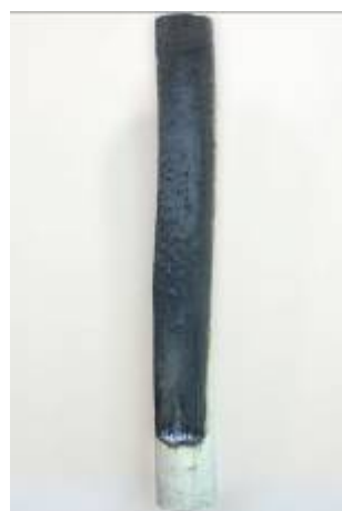
Figure 17 Chartek 7 CCA-treated spotted gum specimen four hours after AS 1530.8.1 test start
