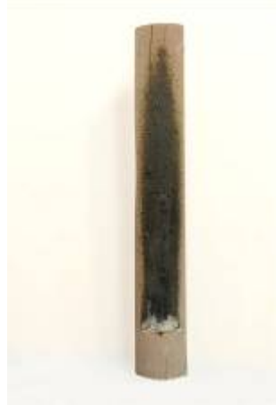
Figure 18 FireGuard CCA-treated spotted gum specimen four hours after AS 1530.8.1 test start
