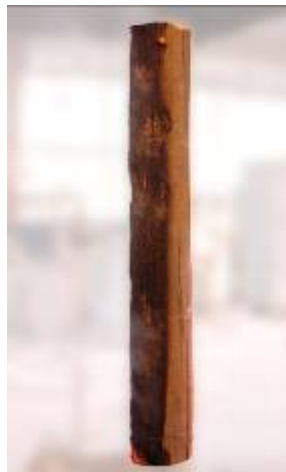
Figure 19 FireTard 120 CCA-treated spotted gum specimen four hours after AS 1530.8.1 test start
