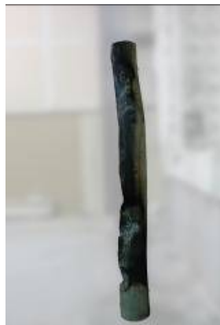
Figure 12 CCA-treated spotted gum specimen 24 hours after testing at 60 kW/m 2 without being subjected to a 2 m/s wind exposure
