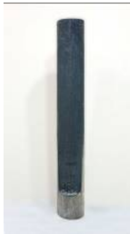
Figure 15 Creosote-treated spotted gum specimen four hours after AS 1530.8.1 test start
