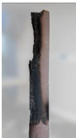
Figure 7 FireGuard CCA-treated spotted gum specimen four hours after testing at 60 \text{ kW/m}^2 and being subjected to a 2 m/s wind
