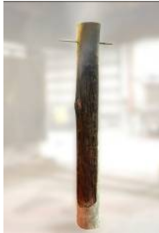
Figure 16 CCA-treated spotted gum specimen four hours after AS 1530.8.1 test start
