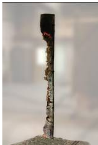
Figure 23 CCA-treated spotted gum specimen 24 hours after AS 1530.8.1 test start
