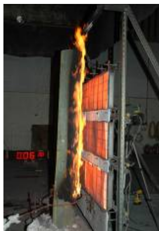
Figure 2 CCA-treated spotted gum specimen six minutes after ENA pole fire test start
