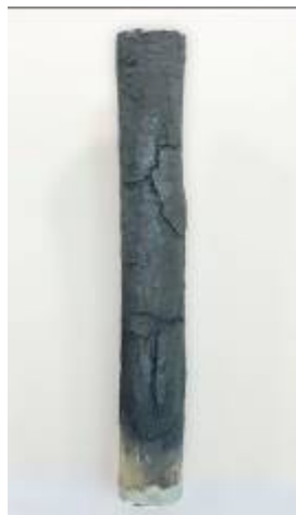
Figure 6 Chartek 7 CCA-treated spotted gum specimen four hours after testing at 60 kW/m 2 and being subjected to a 2 m/s wind
