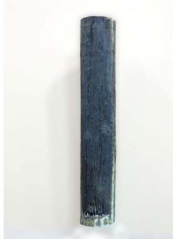
Figure 22 FRX CCA-treated radiata pine specimen four hours after AS 1530.8.1 test start
