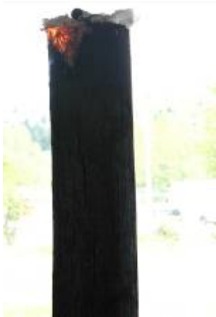
Figure 9 Combustion at top of FRX CCA-treated spotted gum specimen one hour after testing at 60 kW/m 2 and being subjected to a 2 m/s wind
