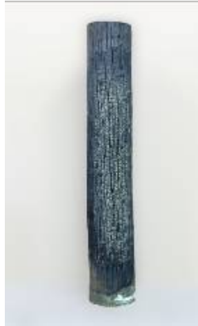
Figure 11 FRX CCA-treated radiata pine specimen four hours after testing at 60 kW/m 2 and being subjected to a 2 m/s wind
