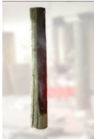
Figure 20 FRX CCA-treated spotted gum specimen four hours after AS 1530.8.1 test start
