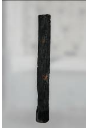
Figure 5 CCA-treated radiata pine specimen four hours after testing at 60 kW/m 2 without a subsequent 2 m/s wind exposure
