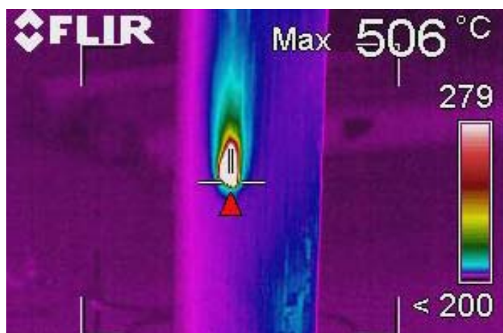
Figure 26 Infrared image of glowing combustion in CCA-treated spotted gum
