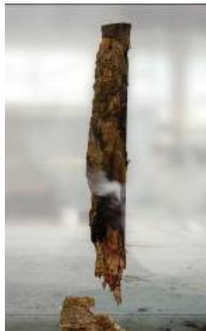
Figure 24 FireTard 120 CCA-treated spotted gum specimen 24 hours after AS 1530.8.1 test start
