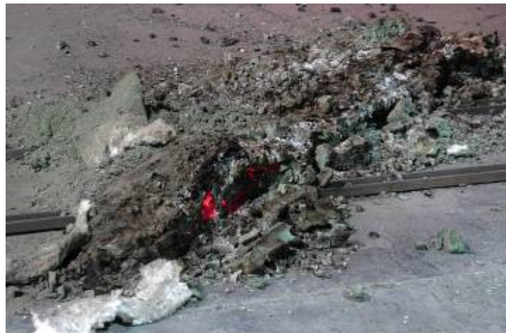
Figure 14 CCA-treated radiata pine specimen 24 hours after testing at 60 \text{ kW/m}^2 without subsequent 2 m/s wind exposure
