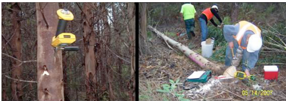
Figure 3. Acoustic velocity measurements were taken from opposing diameters from each tree. Log values were taken using the HM 200 on felled stems
