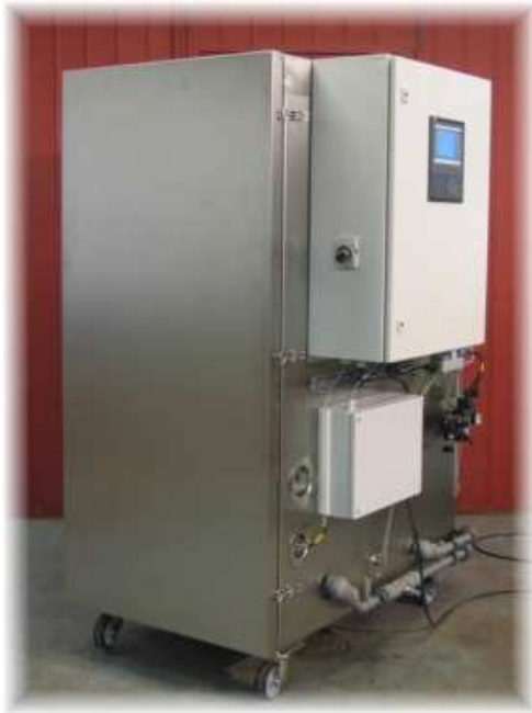
Figure 2.1: Example of a 1m 3 test chamber.
