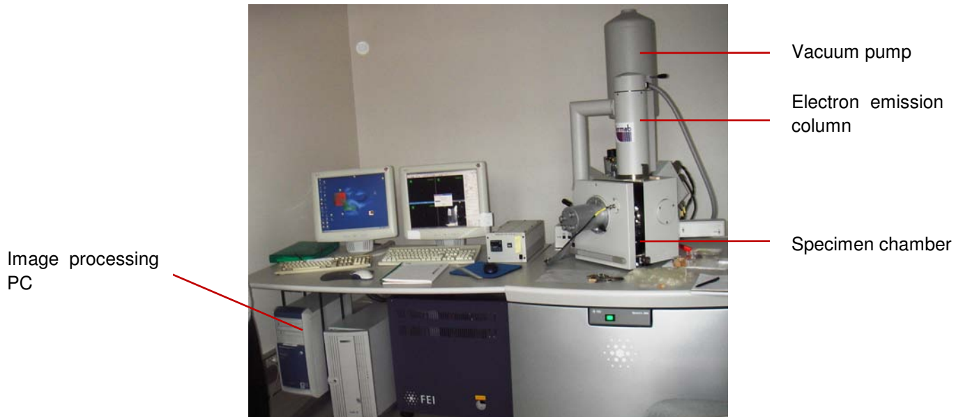
Figure 7. FEI Quanta 200 3D environmental electron scanning microscope.
