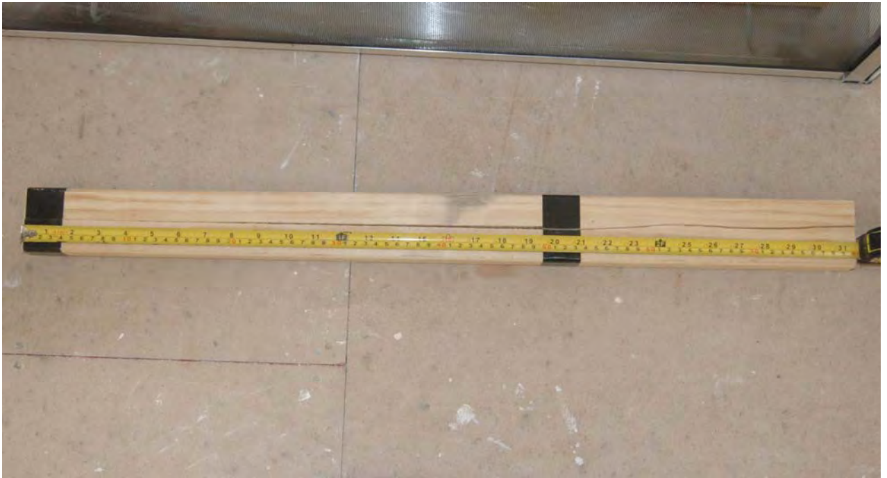
Figure 2: Typical split-beam (trial 1 design) showing tape binding with the left part being the sawn groove and the right part the split section (Photo: RJ Cunningham)
