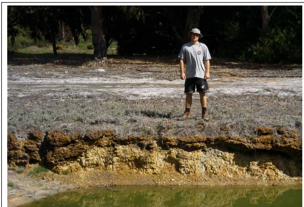
Figure 1. Partially exposed soil profile at Wellstead showing shallow gravelly sand and laterite over a clay subsoil.
