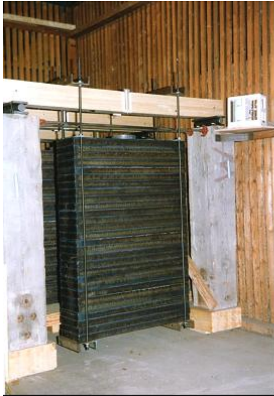
Figure 13. Photograph of the creep deformation tests that have been underway at FMPA for the last 13 years.
