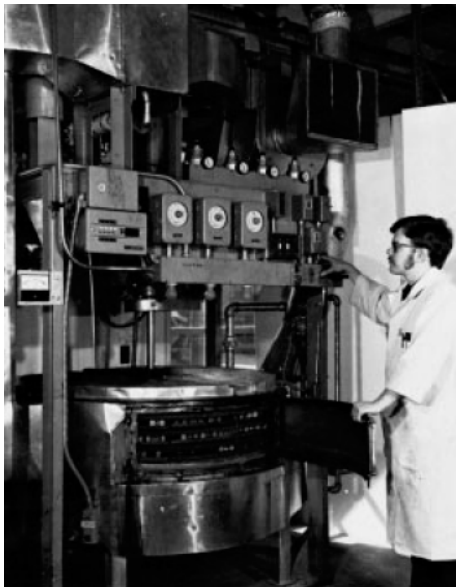
Figure 21. Schematic (a) and photograph (b) of the Automatic Boil test instrument as described in ASTM 4343.
