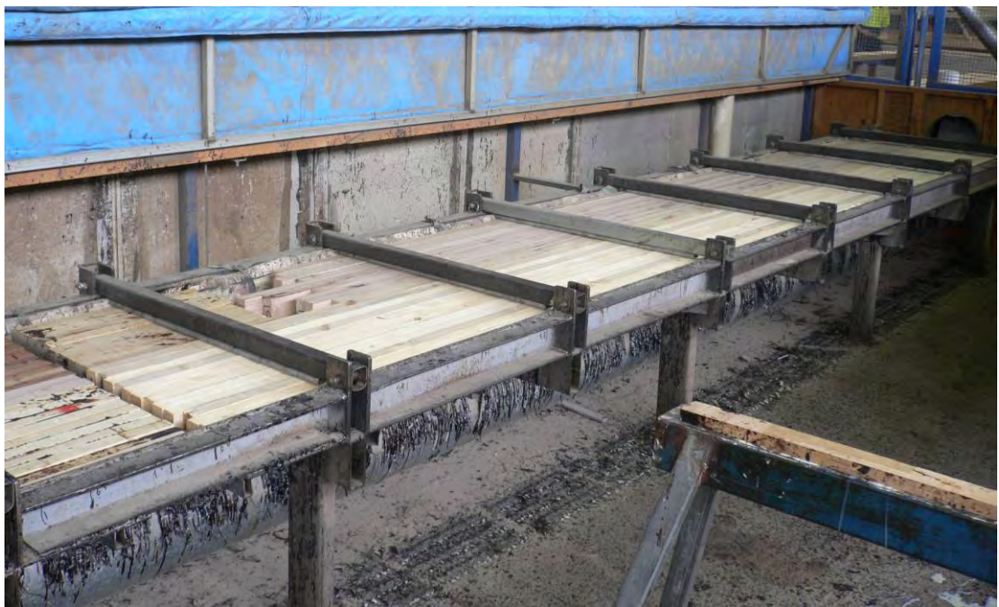
Figure 2. The press at Warrnambool Timber used to manufacture the test beams ( top ) before and ( bottom ) during pressing.
