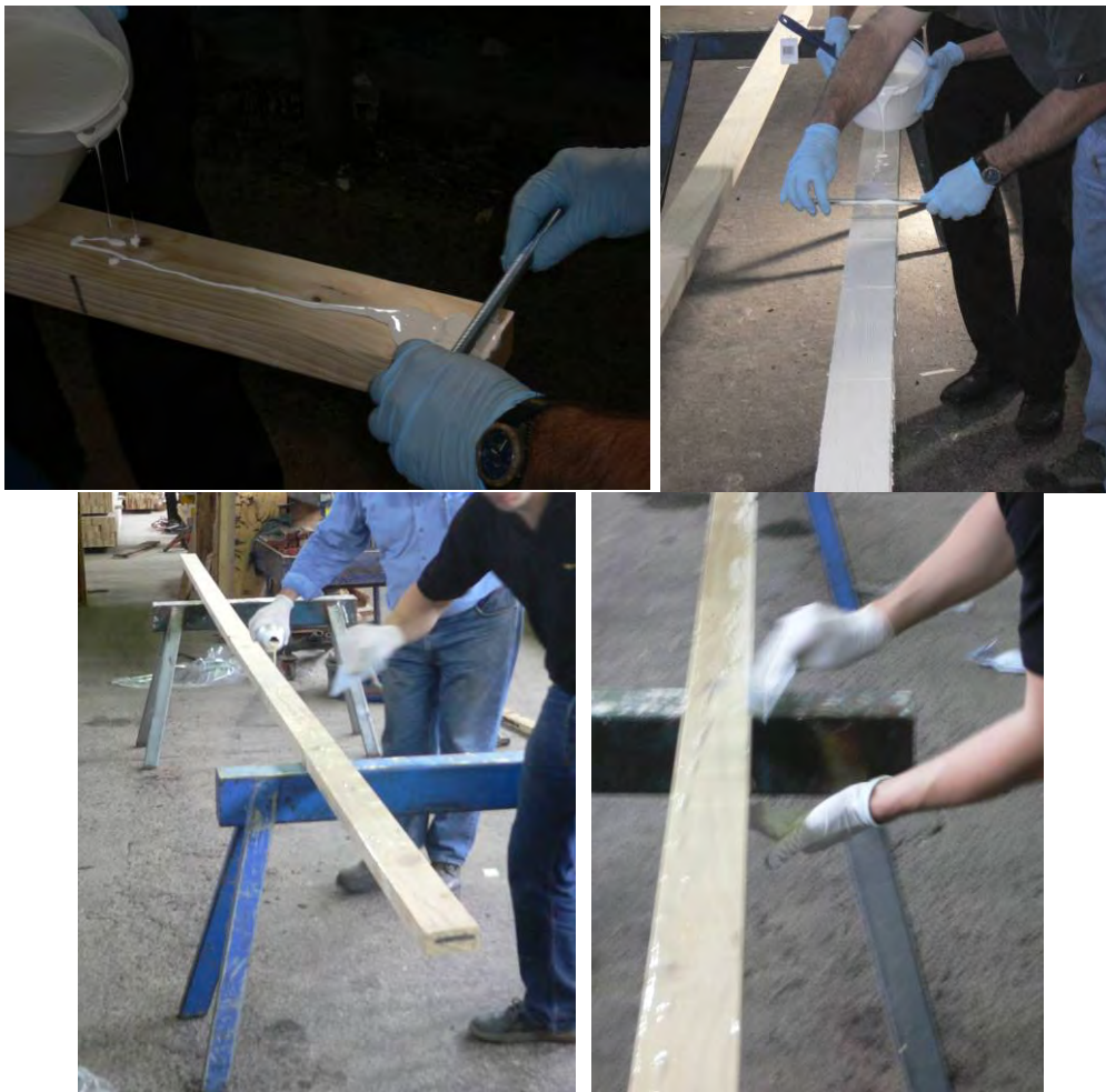
Figure 1. Application of the IBAs was achieved by using a coating rod ( top ) or an adhesive comb ( bottom )
