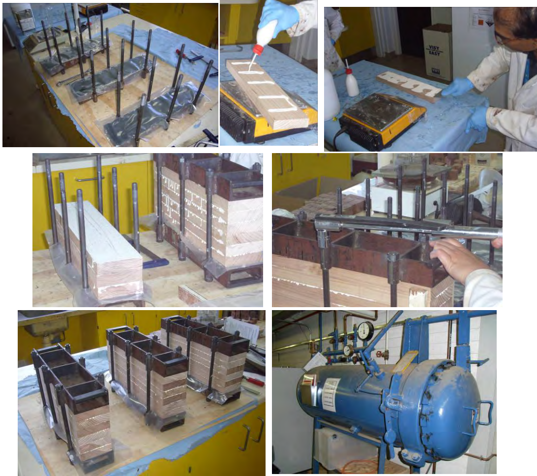
Figure 78. Preparing the bonded assemblies for the delamination test. ( top left ) the clamps used for manufacture; ( top middle ) applying the adhesive; ( top right ) spreading the adhesive; ( middle left ) assembling the glued lamellae in the clamps; ( middle right ) tightening the clamps to the correct pressure and ( bottom left ) the three bonded assemblies in the clamps; ( bottom right ) the vacuum-pressure vessel used for the water soak.
