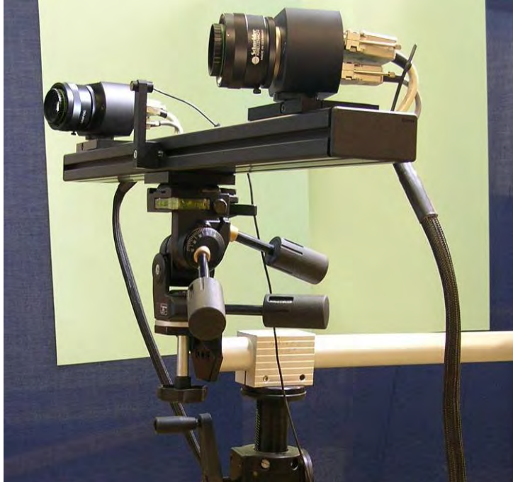
Figure 85. Aramis system digital cameras used to capture digital images.
