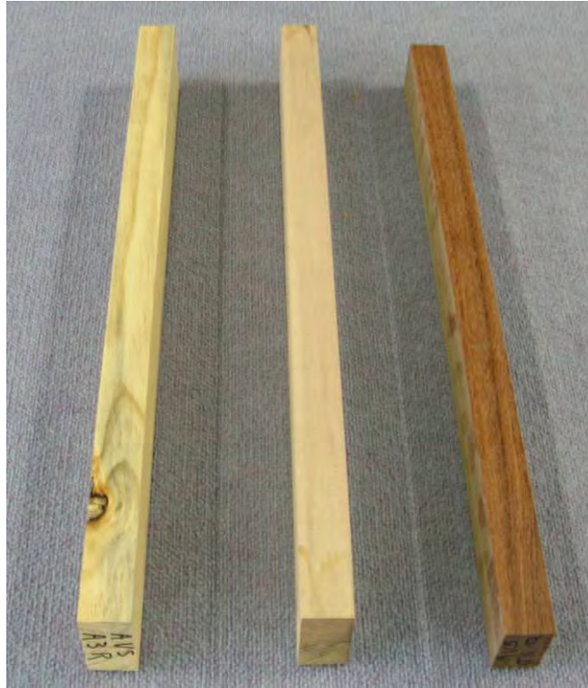
Figure 3. Radiata Pine ( left ), Victorian Ash ( middle ) and Spotted Gum ( right ) test beams for the exposure study
