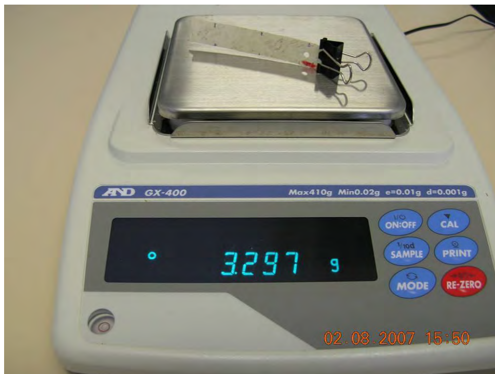
Figure 90. Specimen under observation to observe weight changes.
