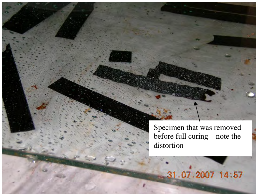
Figure 87. Thin films of PRF held between two glass sheets.
