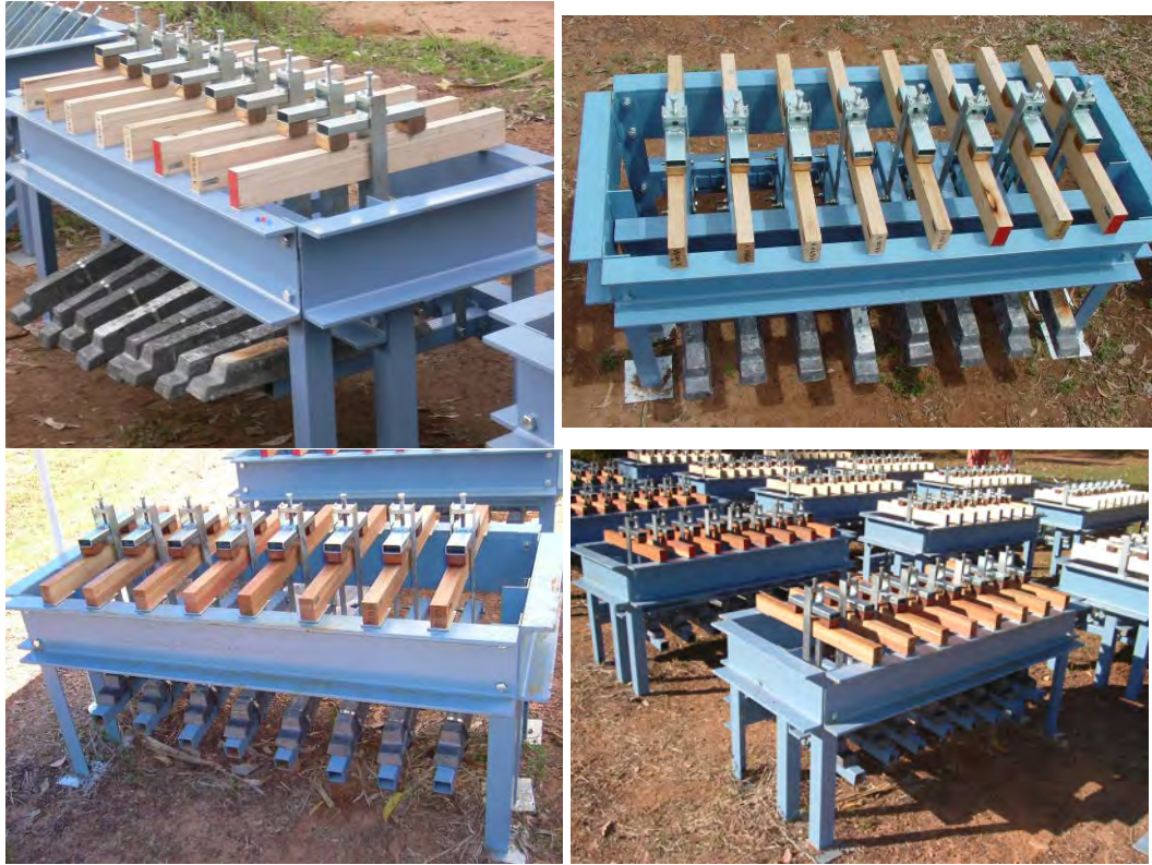
Figure 74. Pictures of the test rigs for the loaded beams at the outdoor exposure site, Darwin.
