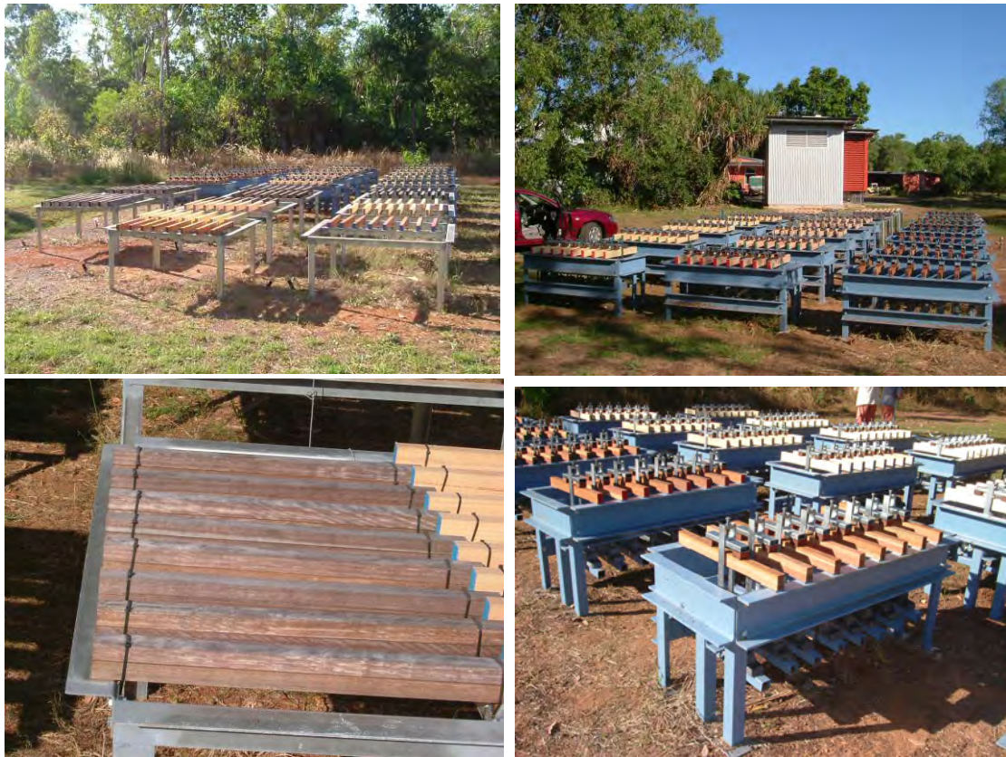
Figure 4. The samples at the exposure site in Darwin; ( top left ) Looking north-west at the samples with the unloaded beams in the foreground; ( top right ) Looking south-east at the samples showing the loaded samples in the foreground; ( bottom left ) A close-up of some of the unloaded samples; ( bottom right ) A close-up of the loaded samples in the test rigs.
