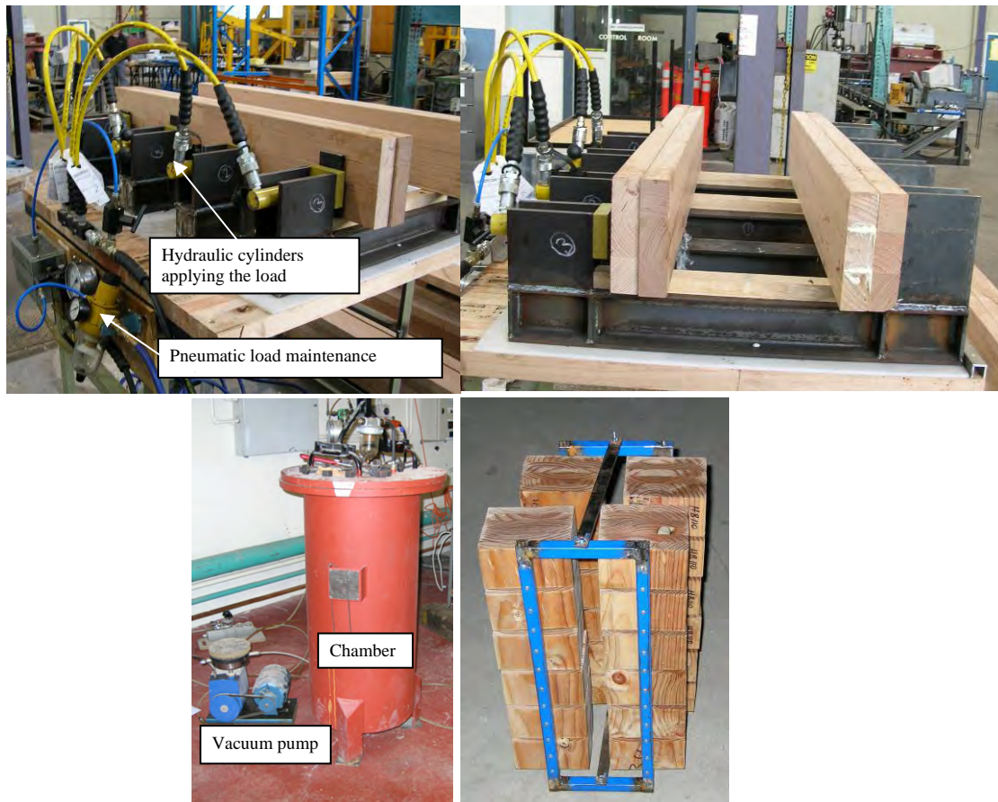
Figure 80.. (top left) Cramping rig used to make test specimens for cyclic delamination tests. The hydraulic cylinders have their load maintained by a pneumatic system. (top right) End view of cramping system showing the caul boards used to evenly distribute the cramping pressure. (bottom left) Test chamber used to apply vacuum and pressure to condition specimens. (bottom right) System used to separate specimens for cyclic delamination test. Screw fastening does not extend below outer laminate.
