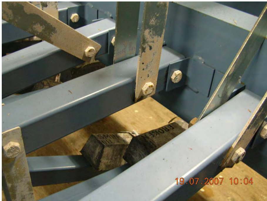
Figure 73. Double cantilever loading mechanism.
