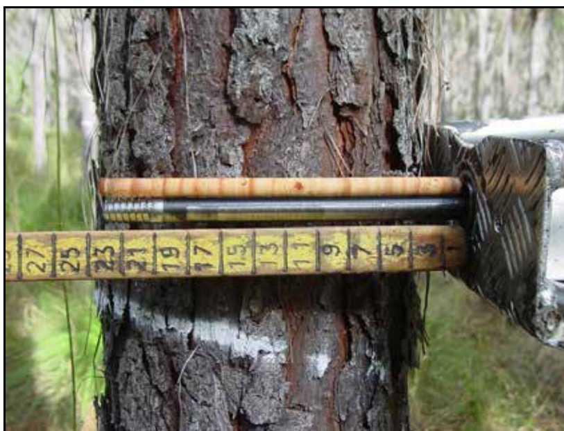
Plate 5. Wood core collected from 350 GYM to assess basic density and spiral grain.
