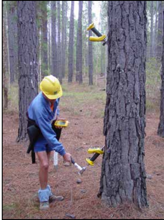
Plate 1. Measuring standing tree acoustic velocity using a FibreGen ® ST300 tool.
