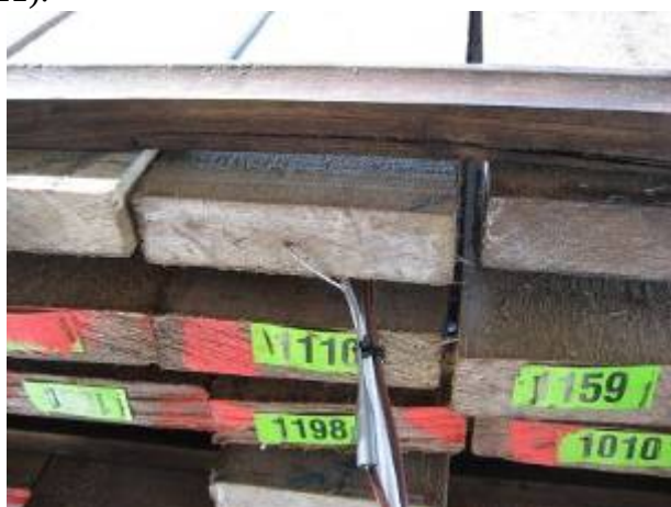
Plate 11. Thermocouple inserted into the end of a test board
