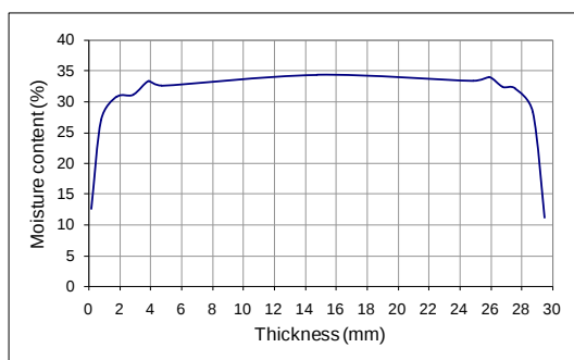
Figure 74. Measured initial moisture content gradient of spotted gum sample board immediately prior to vacuum kiln drying
