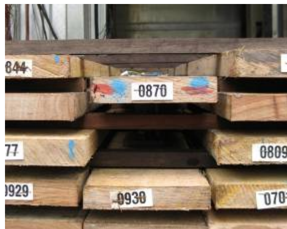
Plate 9. Test board/ load cell arrangement
