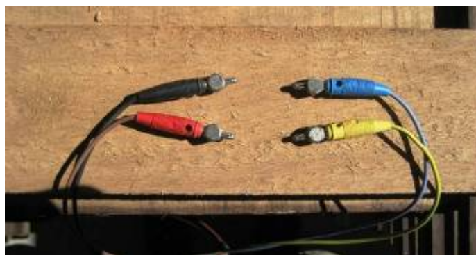
Plate 3. MC resistance probes inserted into a test board
