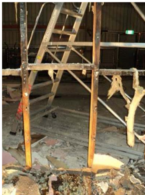
Figure 12 Showing condition of studs post fire test
