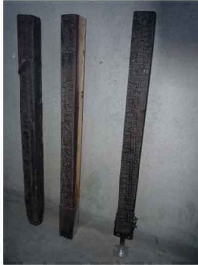
Figure 4 Results from various post configurations being exposed to radiant heat and timber crib
