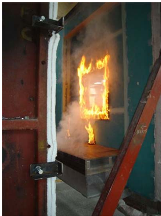
Figure 5 WRC window and hardwood deck facade test being exposed to radiant panel
