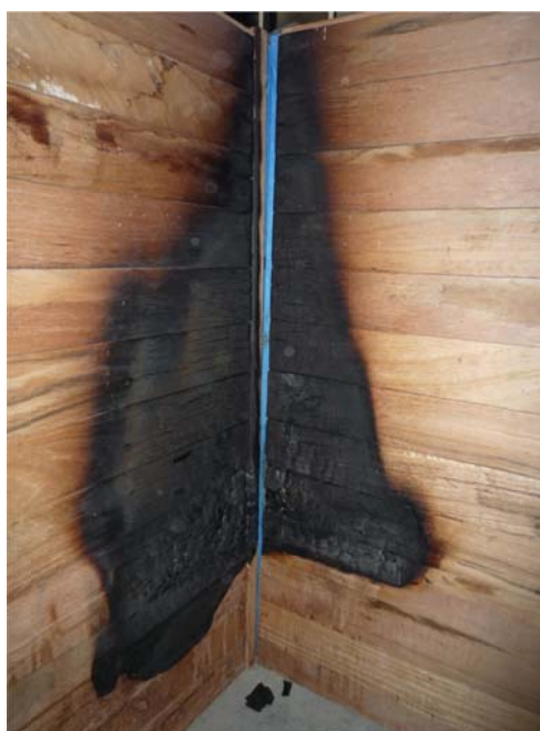
Figure 2 Hardwood cladding after exposure to timber crib screen test
