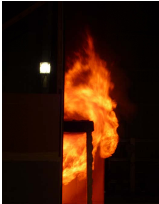
Figure 15 Flames coming out of room and wrapping around 600 mm projection
