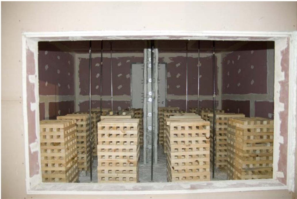
Figure 8– Photo of cribs in fire room. Steel column is visible in centre of room.
