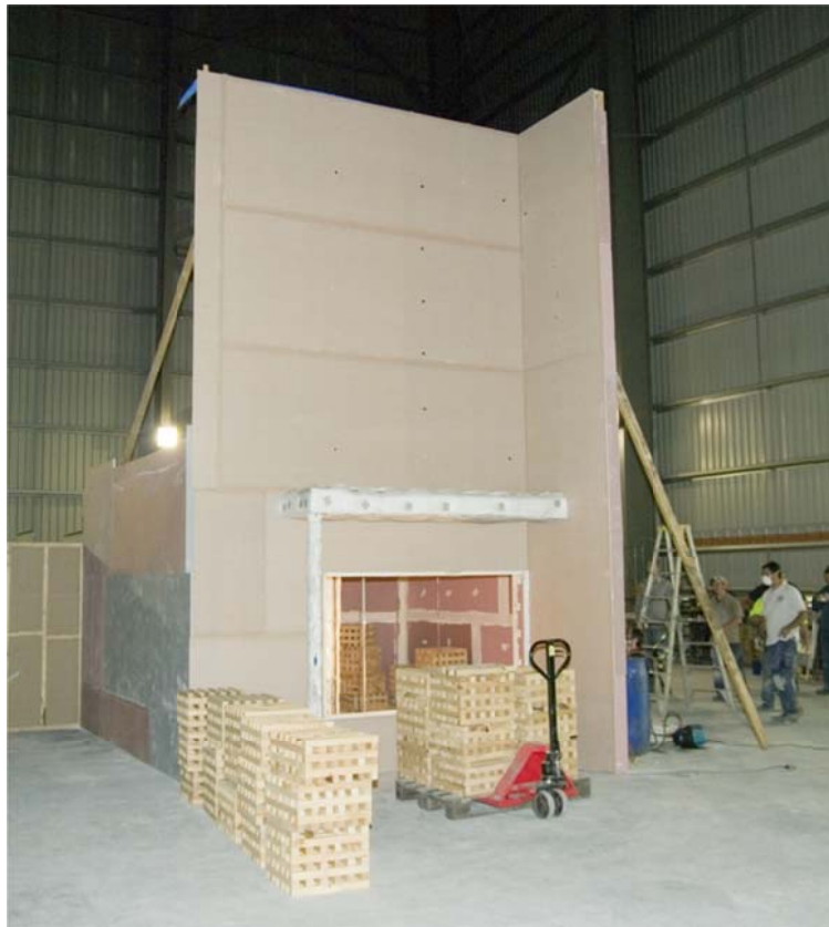
Figure 7 Completed Test Specimen with timber cribs in foreground
