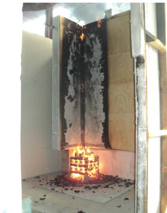
Figure 13 Intermediate test of fire retardant plywood without radiant heat load applied
