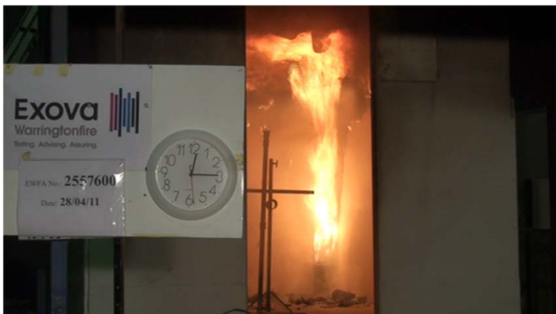
Figure 17 ISO room test - western red cedar linings
