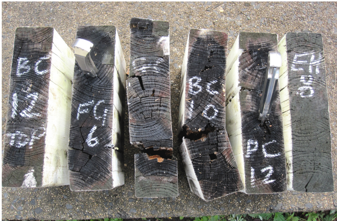
Figure 19. Top ends of azole-treated test specimens exposed vertically for 3.2 years at Innisfail. BC12 = P. radiata treated ( 40 \text{ l/m}^3 ) after gluing with deep decay in 5 laminates rating 0; FG6 = P. elliotii treated ( 43 \text{ l/m}^3 ) after gluing and sealed with CuN with deep decay in 5 laminates rating 0; GC8 = P. elliotii treated ( 56 \text{ l/m}^3 ) before gluing with deep decay in 7 laminates rating 0; BC10 = P. radiata treated ( 40 \text{ l/m}^3 ) after gluing with deep decay in 8 laminates rating 0; DC12 = P. radiata treated ( 69 \text{ l/m}^3 ) after gluing with 6 laminates rating 0; EH8 = P. elliotii treated ( 35\text{-}40 \text{ l/m}^3 ) before gluing with moderate decay in 1 laminate rating 5.
