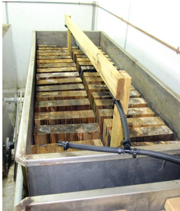
Figure 18. Trough containing glulam test specimens after 3.1 years in the AFS.
