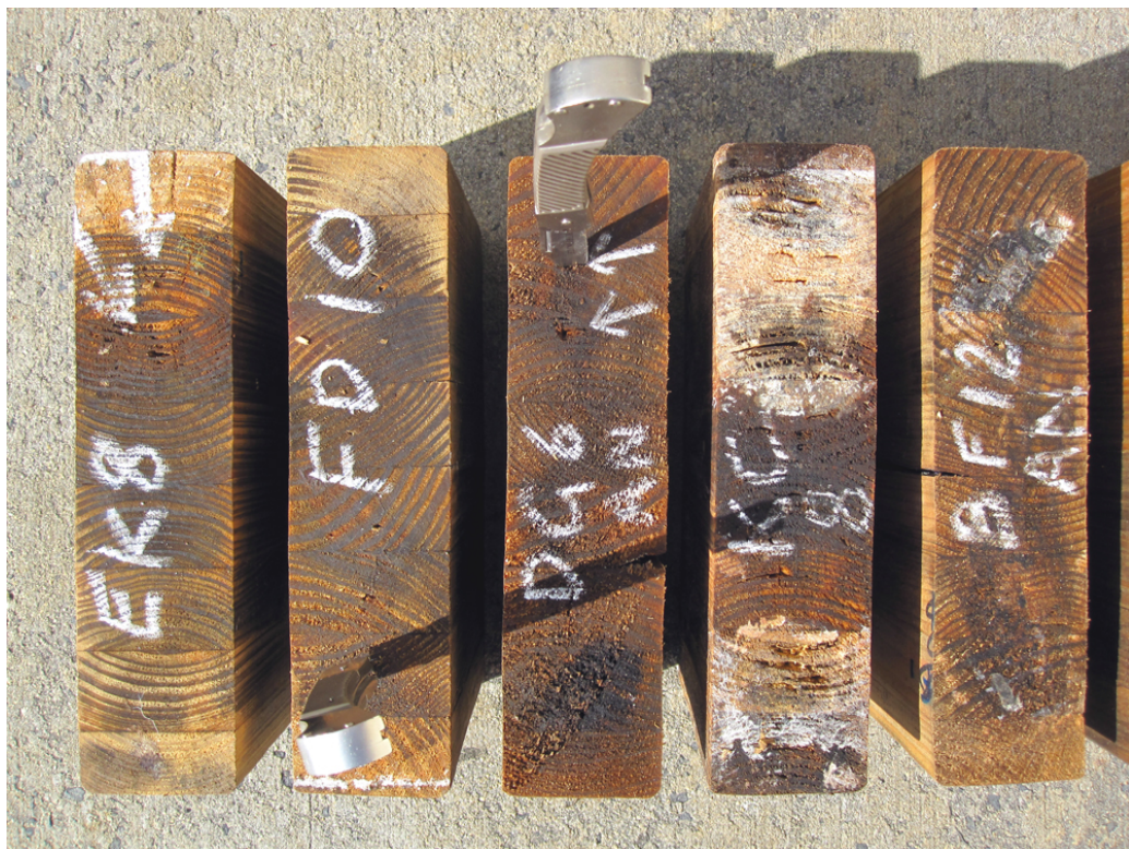
Figure 21. Top ends of specimens exposed vertically for 3.1 years in the AFS. EK8 = P. elliotii treated (35-40 l/m 3 ) before gluing and sealed with ZnN with 16-19 mm brown rot in 2 laminates rating 3; FD10 = P. elliotii treated (43 l/m 3 ) after gluing and sealed with ZnN with 5-65 mm brown rot in 3 laminates rating 0 (failed); DG6 = P. radiata treated (69 l/m 3 ) after gluing with 17 mm brown rot in 2 laminates rating 4; KC8 = untreated P. elliotii with 18-44 mm decay in all laminates rating 0; BF12 = P. radiata treated (40 l/m 3 ) after gluing with 5-22 mm brown rot in 6 laminates rating 0.
