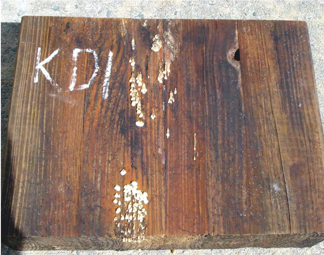
Figure 16. KD1 = untreated P. elliotii exposed vertically for 2.1 years in the AFS, showing bell-shaped fruiting bodies over 2 laminates.
