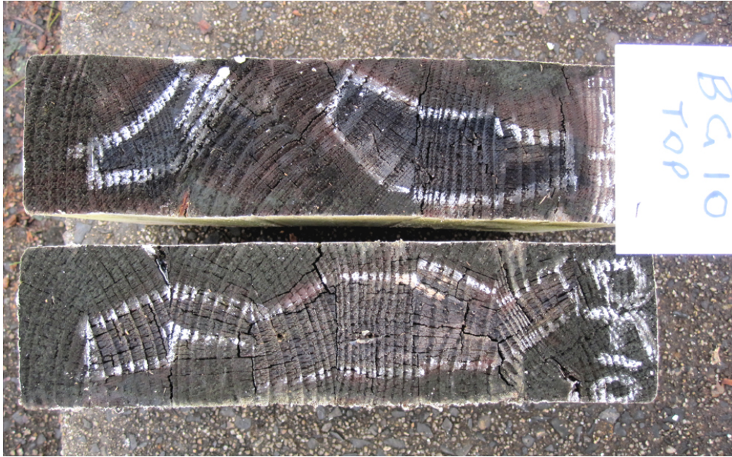
Figure 20. Top ends of azole-treated test specimens exposed vertically for 3.2 years at Innisfail. BG10 = P. radiata treated (40 l/m 3 ) after gluing and sealed with ZnN; DF10 = P. radiata treated (69 l/m 3 ) after gluing. Chalk marks show outline of decayed or discoloured regions where preservative penetration may have been lacking.
