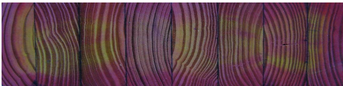
Figure 27. Original image of JE5 after spot testing with PAN indicator.
