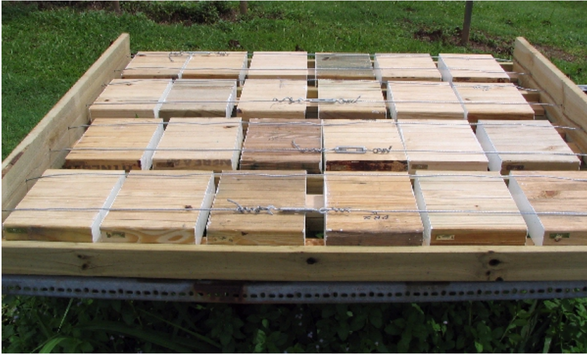
Figure 3. Another frame of test specimens laying flat and exposed at Innisfail.
