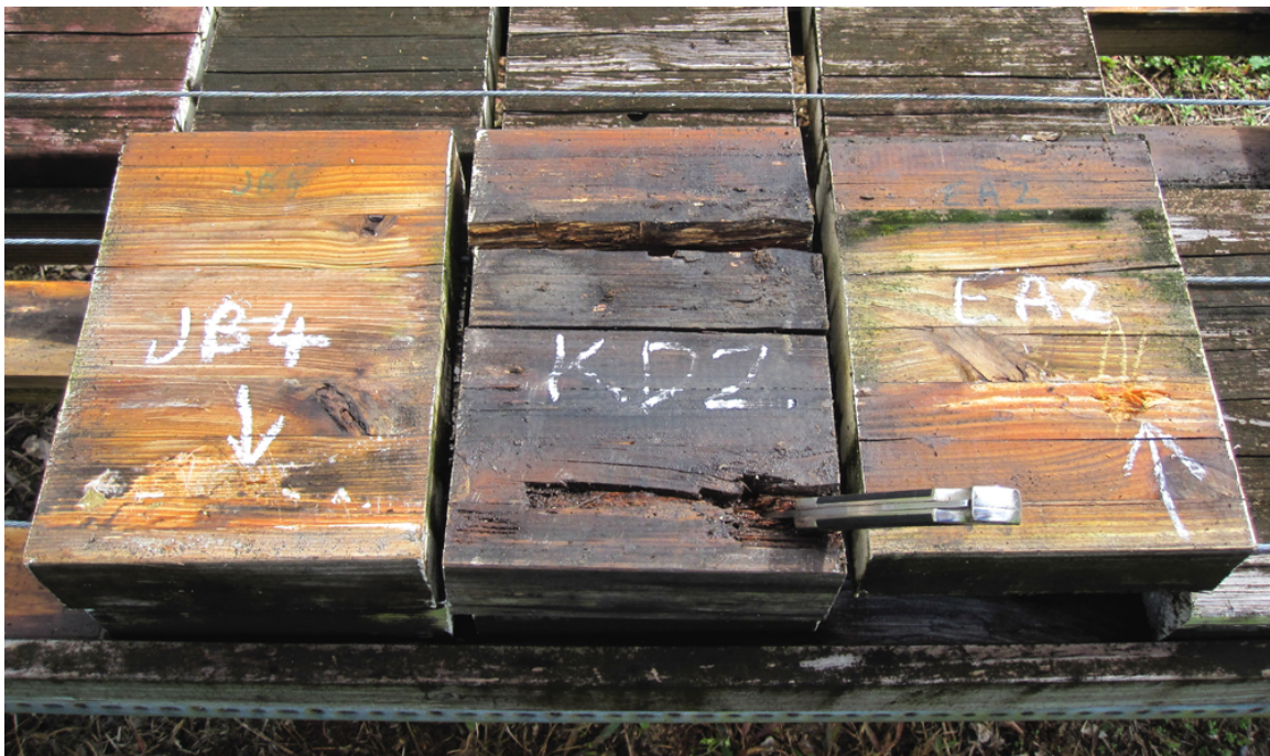
Figure 11. Underside of test specimens after 3.2 years at Innisfail. JB4 = TBTN-treated ( 37 \text{ l/m}^3 ) P. elliotii with light decay rating 7; KD2 = top side of untreated P. elliotii fully brown rotted rating 0; EA2 = P. elliotii treated ( 35\text{-}40 \text{ l/m}^3 ) before gluing with light-moderate decay rating 6.
