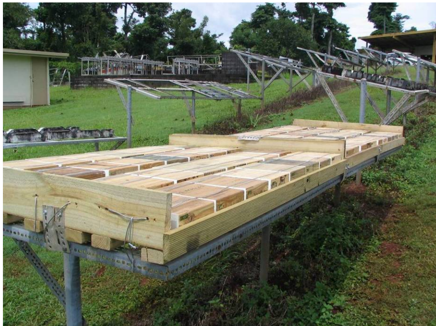
Figure 33. A test frame newly installed at Innisfail. Test specimens rest upon untreated pine strips (hidden) which were nailed upon 70 x 35 mm CCA-treated pine bearers (visible at one end of frame).
