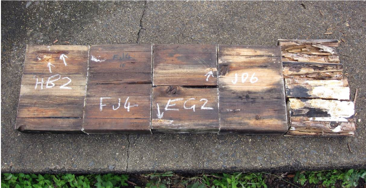
Figure 10. Underside of test specimens after 3.2 years at Innisfail. HB4 = P. elliotii treated ( 82 \text{ l/m}^3 ) after gluing with light-moderate decay rating 6; FJ4 = P. elliotii treated ( 43 \text{ l/m}^3 ) after gluing without decay rating 8; EG2 = P. elliotii treated ( 35\text{-}40 \text{ l/m}^3 ) before gluing with light decay rating 7; JD6 = TBTN-treated ( 37 \text{ l/m}^3 ) P. elliotii without decay rating 8; KA3 = untreated P. elliotii fully brown rotted rating 0.
