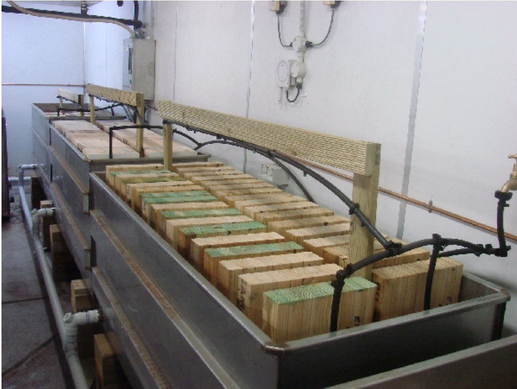
Figure 1. Three tanks in the AFS containing rows and layers of glulam test specimens, with irrigation and drainage system. Green ends are test specimens brushed with CuN end seal.
