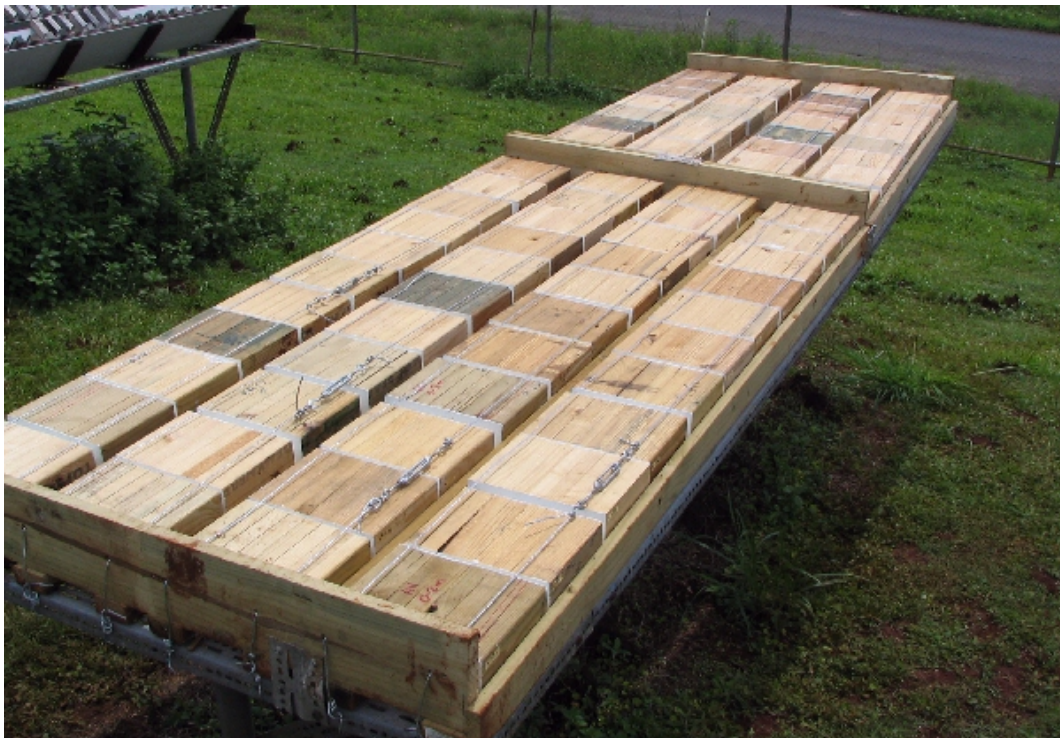
Figure 2. Two frames of test specimens laying flat (horizontally) and exposed at Innisfail. Top wires aid retention of test specimens during cyclones. Test specimens sealed with epoxy on their ends.
