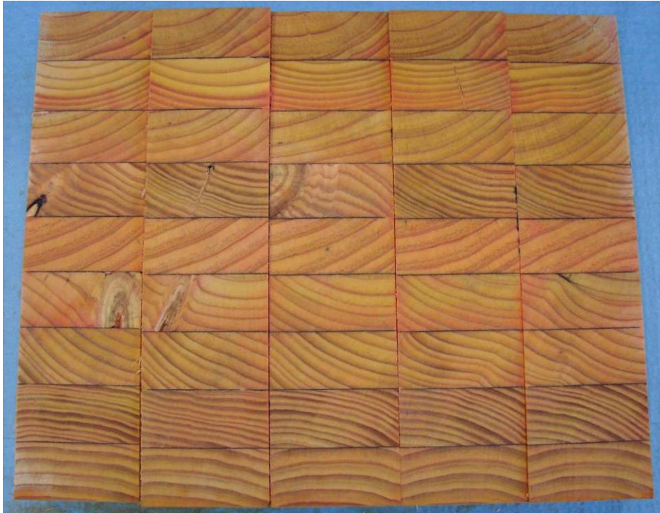
Figure 7: Azole-treated (before gluing) P. radiata beam AJ, showing PAN stained wafers AJ3, AJ5, AJ7, AJ9, AJ11 (left to right) removed from between test specimens (which were AJ2, AJ4, AJ6, AJ8, AJ10, AJ12). Showing limited success (mean of 15% penetration) as spot test for zinc (red coloured regions).
