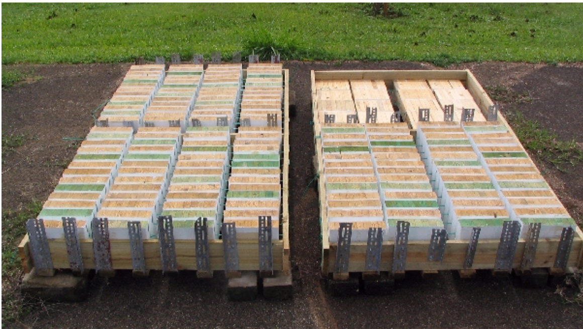
Figure 4. Vertical test specimens at Innisfail, and a small set of flat laying test specimens (in top right frame). Note that the sides of the vertical specimens at Innisfail were painted. Specimens with green ends had been resealed with CuN.
