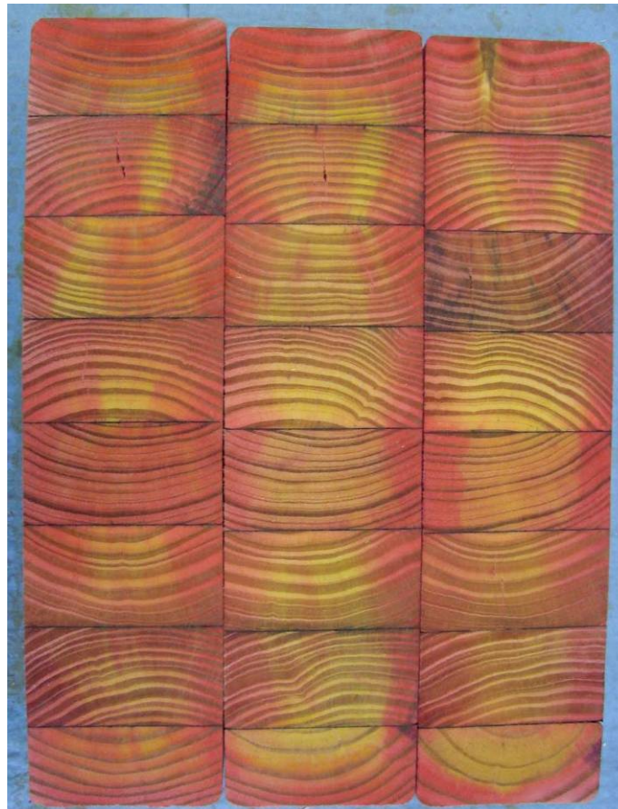
Figure 6: TBTN-treated P. radiata beam JE, showing PAN stained wafers JE3, JE5, JE7 (left to right) removed from between test specimens (which were JE2, JE4, JE6, JE8). Showing good spot test for tin (red coloured regions).
