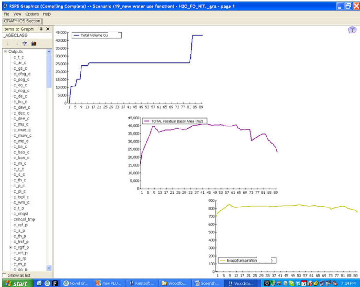
Figure 19. FEM screenshot showing volume cut ( \text{m}^3/\text{yr} ), standing basal area ( \text{m}^2 ) and evapotranspiration ( \text{mm}/\text{yr} ) for each year of a 90-year simulation where objective is to have non-declining total volume cut and smoothed evapotranspiration ( \pm 10\% ) scenario for 1532 ha of E. nitens plantation in the Florentine Valley
