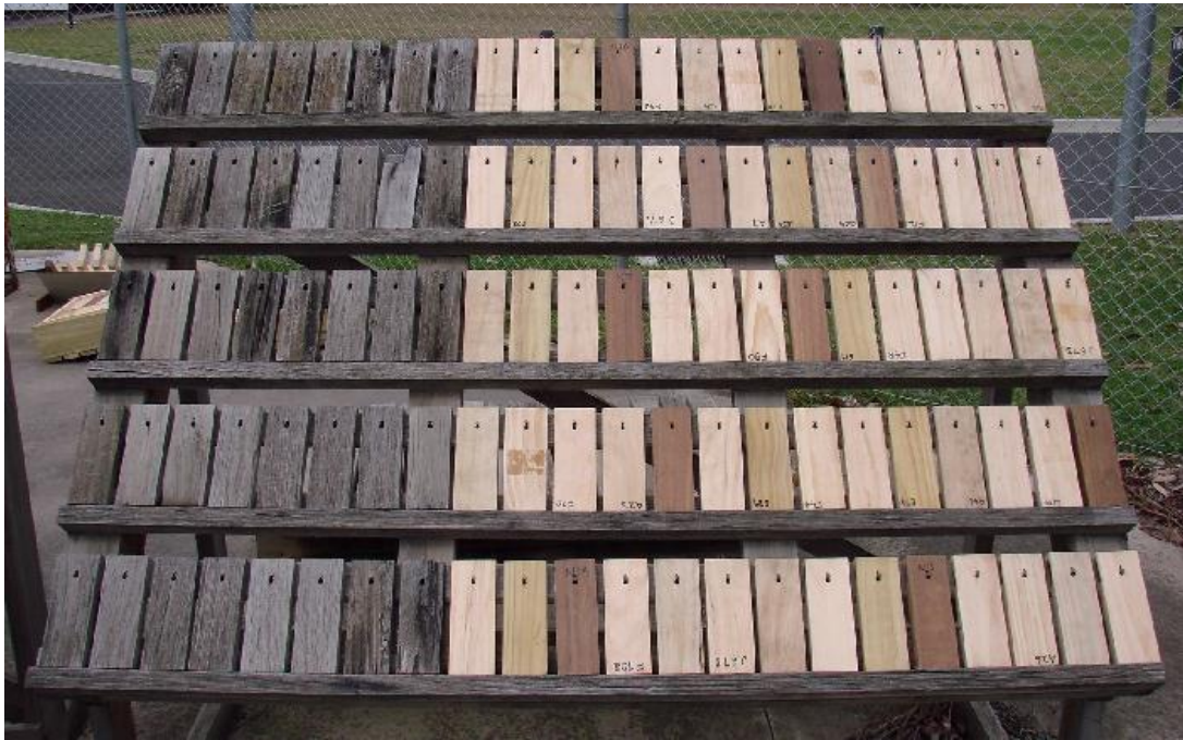
Figure 4. Flat panel test installed of A-list specimens at Clayton, on existing ten year old frame.
