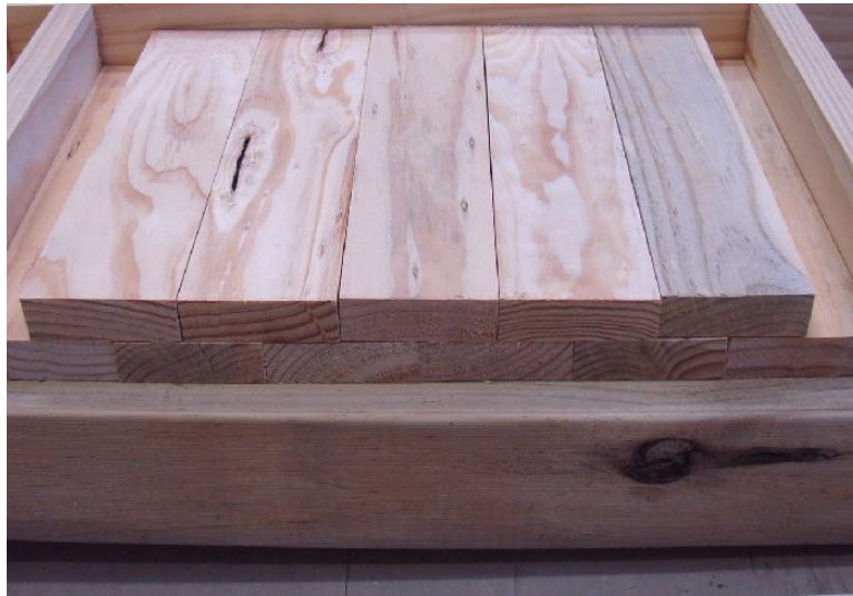
Figure 33. Mock up of double layer test, showing 11 specimens (10 test specimens, and one spare).
