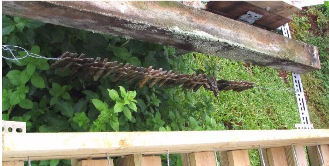
Figure 40. Clothes peg test after three months at Innisfail.
