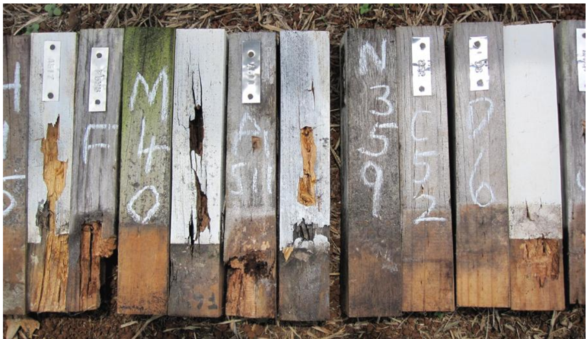
Figure 49. Embedded test at Innisfail after four years, frame H. Left to right = H15 CCA (H3) rating 8, A517 water painted rating 0, F586 TBTN rating 0, M40 azoles (H3) rating 8, F650 TBTN painted rating 0, A511 water rating 0, J778 HFK painted rating 0, N359 C. maculata rating 8, C52 CuCr ('H3') rating 8, D6 ACQ (H3) rating 8, G547 CCA painted rating 6.
