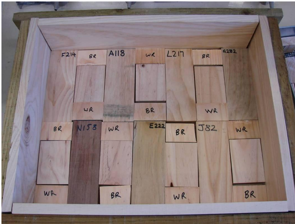
Figure 27. Bottom layer of test specimens and pre-inoculated blocks for Clayton AFS rot box. WR = white rot and BR = Brown rot.
