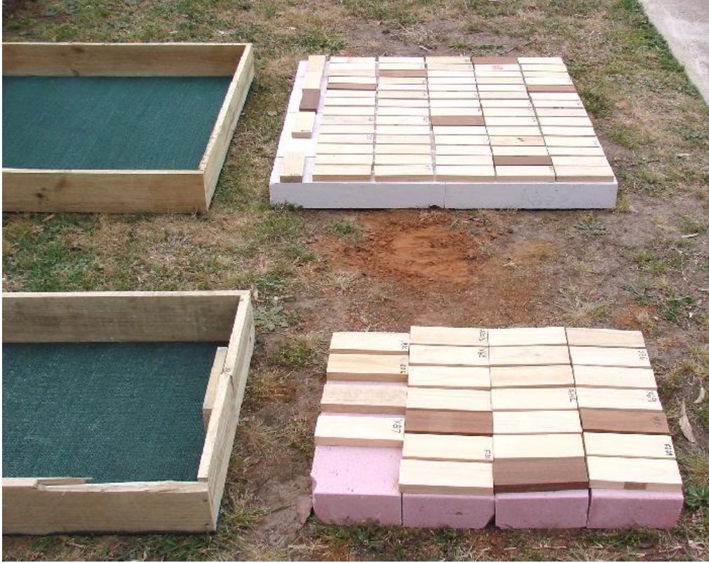
Figure 30. Ground proximity test installed at Clayton (shade cloth covers removed).
