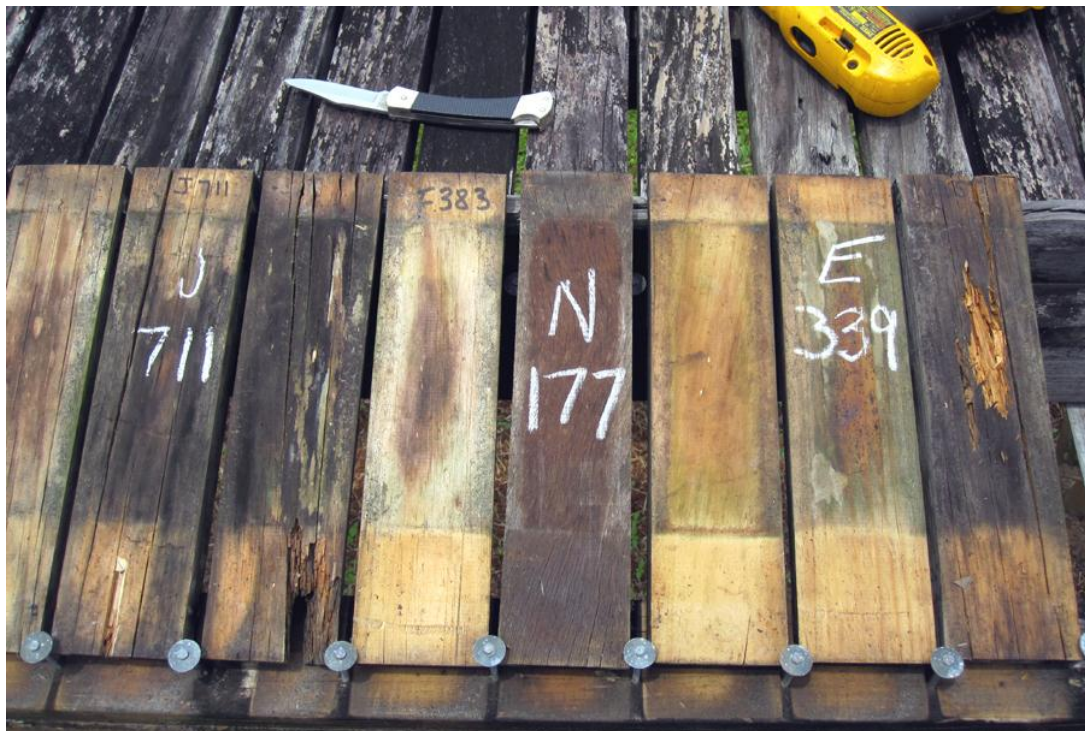
Figure 47. Raised deck at Innisfail after four years, underside. Left to right = F343 TBTN rating 8, J711 HFK rating 1, A229 water rating 0, F383 TBTN rating 8, N177 C. maculata rating 8, G395 CCA rating 8, E339 ACQ rating 8, L357 azoles rating 0.
