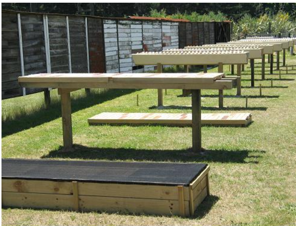
Figure 1. General view at Rotorua of double layer, decking and embedded tests upon installation.
