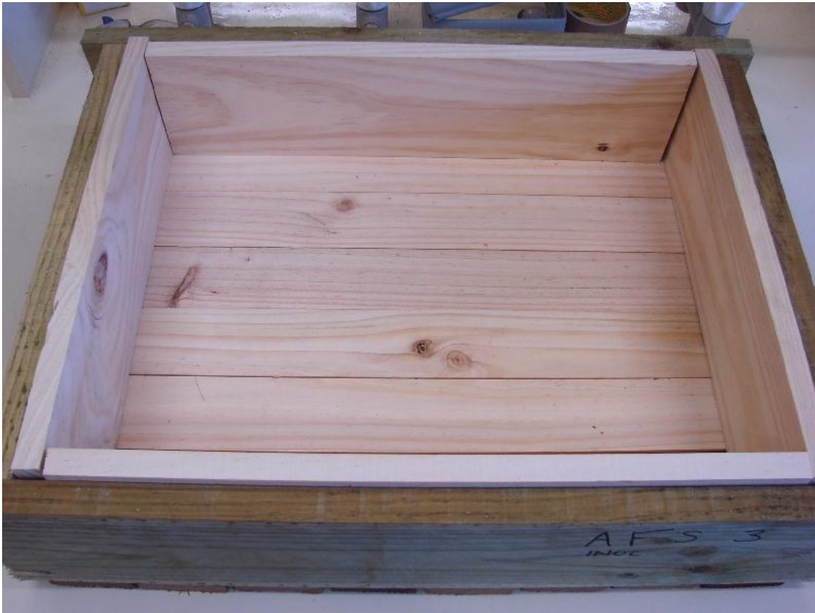
Figure 22. Rot box lined with untreated P. radiata , prior to placement of test specimens.
