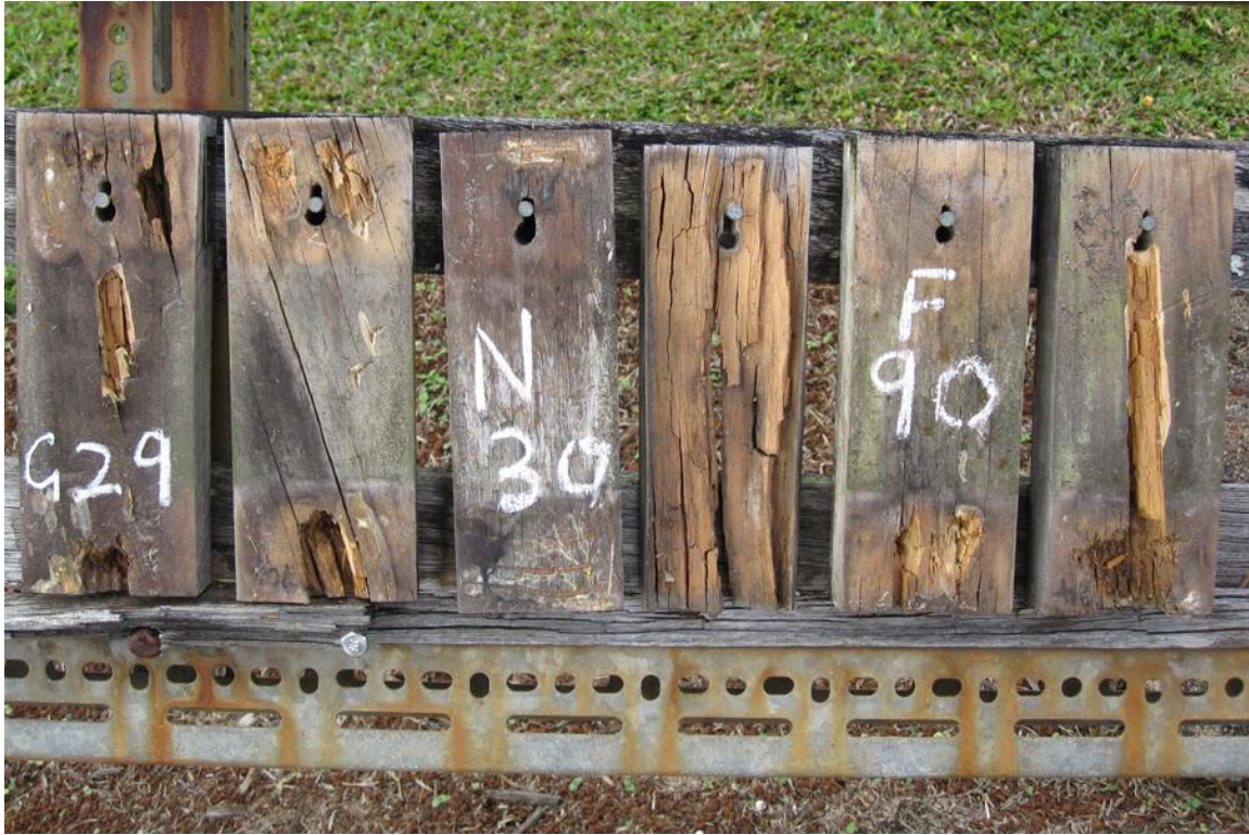
Figure 44. Flat panel test on old frame at Innisfail after four years, underside. Left to right = G29 CCA rating 0, L701 azoles rating 0, N30 C. maculata rating 8, J633 HFK rating 0, F90 TBTN rating 3, E24 ACQ rating 0.
