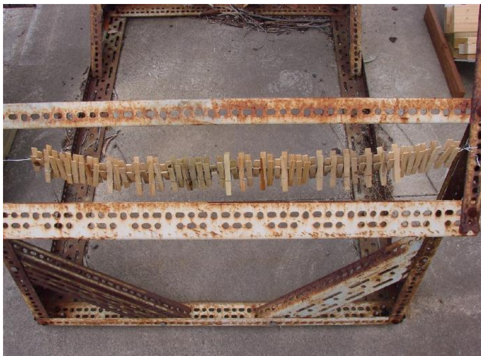
Figure 41. Clothes peg test installed at Clayton.
