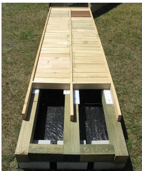
Figure 36. Double layer test installed at Rotorua (plastic strips nailed on bearers removed soon after installation, to be similar to the Innisfail frame).
