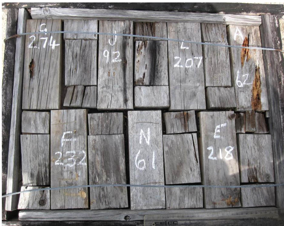
Figure 53. Inoculated rot box No. 14 at Innisfail after four years, top row, inoculated feeder bait blocks alternate with test specimens. Left to right = G274 CCA rating 4, J92 HFK rating 0, L207 azoles rating 7, A62 water rating 0, F232 TBTN rating 5, N61 C. maculata rating 7, E218 ACQ rating 6.
