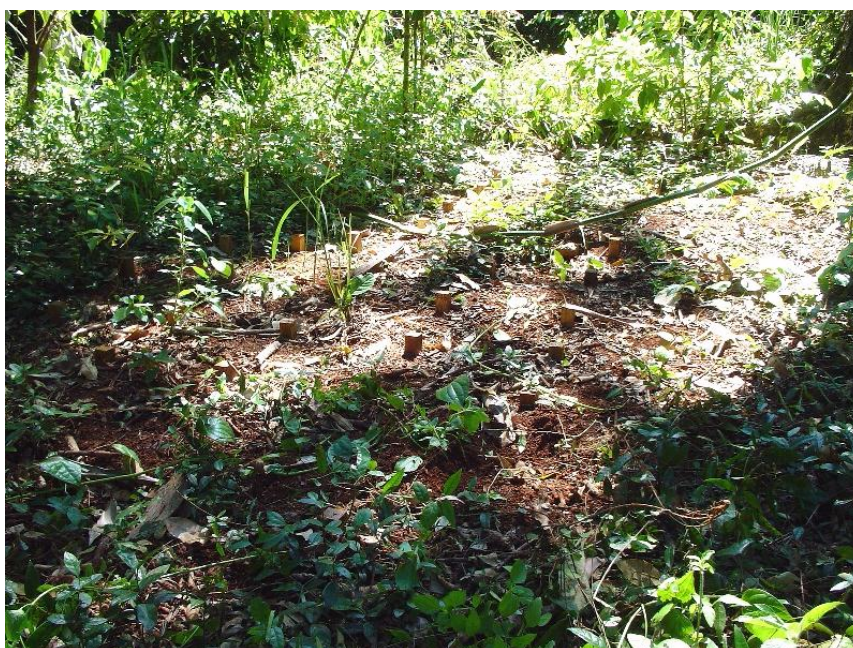
Figure 38. In-ground stakes in rainforest clearing at Innisfail, six months after installation.
