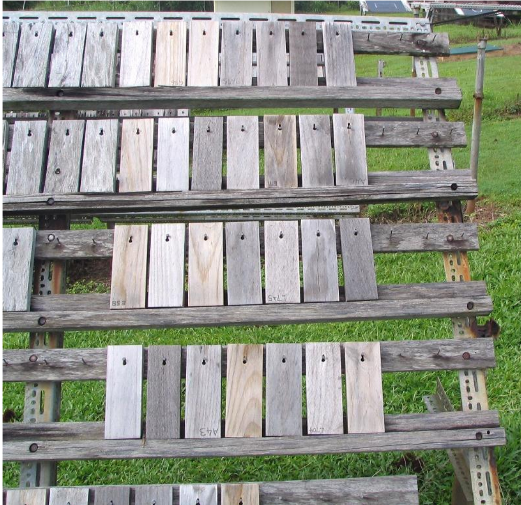
Figure 3. Flat panel test installed at Innisfail on 'old frame'. The seven columns of test specimens on the right side of the frame are the test specimens for this project.
