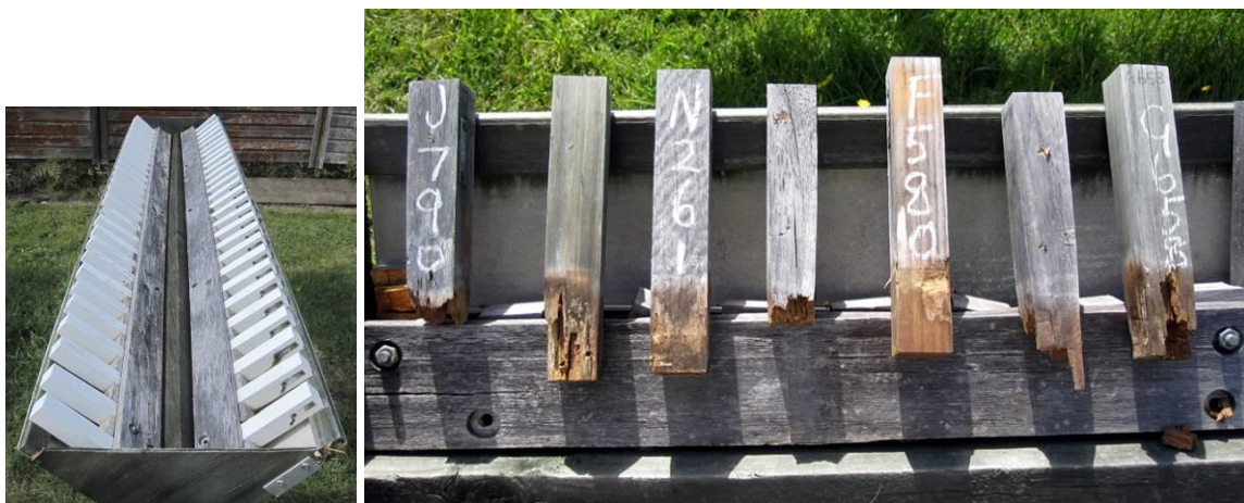
Figure 51. Embedded tests at Rotorua after four years. Left photo, painted specimens. Right photo, frame No. 5 in AFS (not inoculated), left to right J790 HFK rating 0, E631 ACQ rating 0, N261 C. maculata rating 7, L630 azoles rating 0, F530 TBTN rating 7, A496 water rating 0, G659 CCA rating 0.
