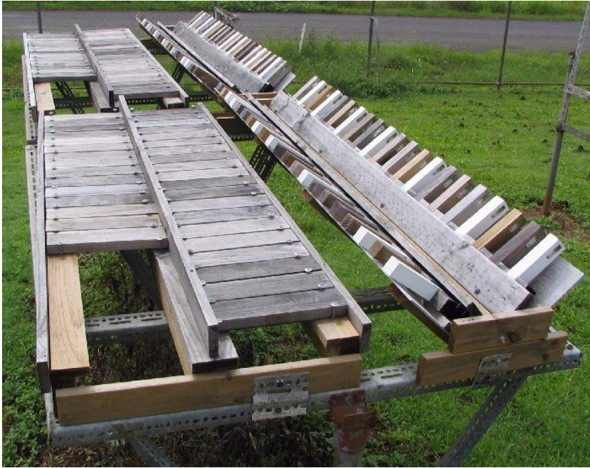
Figure 12. Raised decking trial (on left), and embedded test (on right) after three months at Innisfail.
