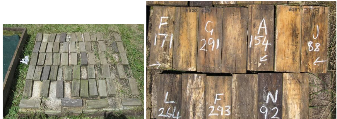
Figure 56. Ground proximity test at Clayton after four years. Left to right underside = F171 TBTN rating 7, E320 ACQ rating 7, G291 CCA rating 8, L790 azoles rating 8, A154 water rating 7, E287 ACQ rating 8, J88 HFK rating 4.
