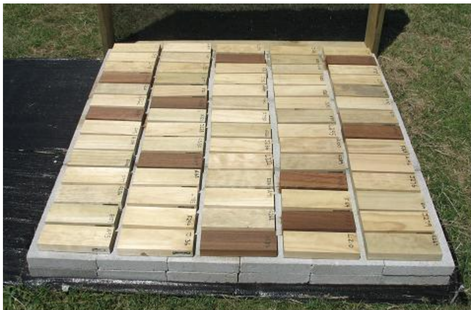
Figure 32. Ground proximity test at Rotorua, with shade-cloth frame removed.
