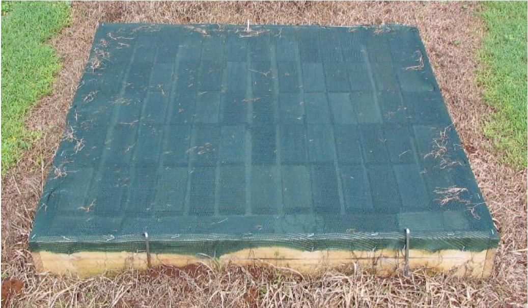
Figure 31. Ground proximity test after three months at Innisfail.
