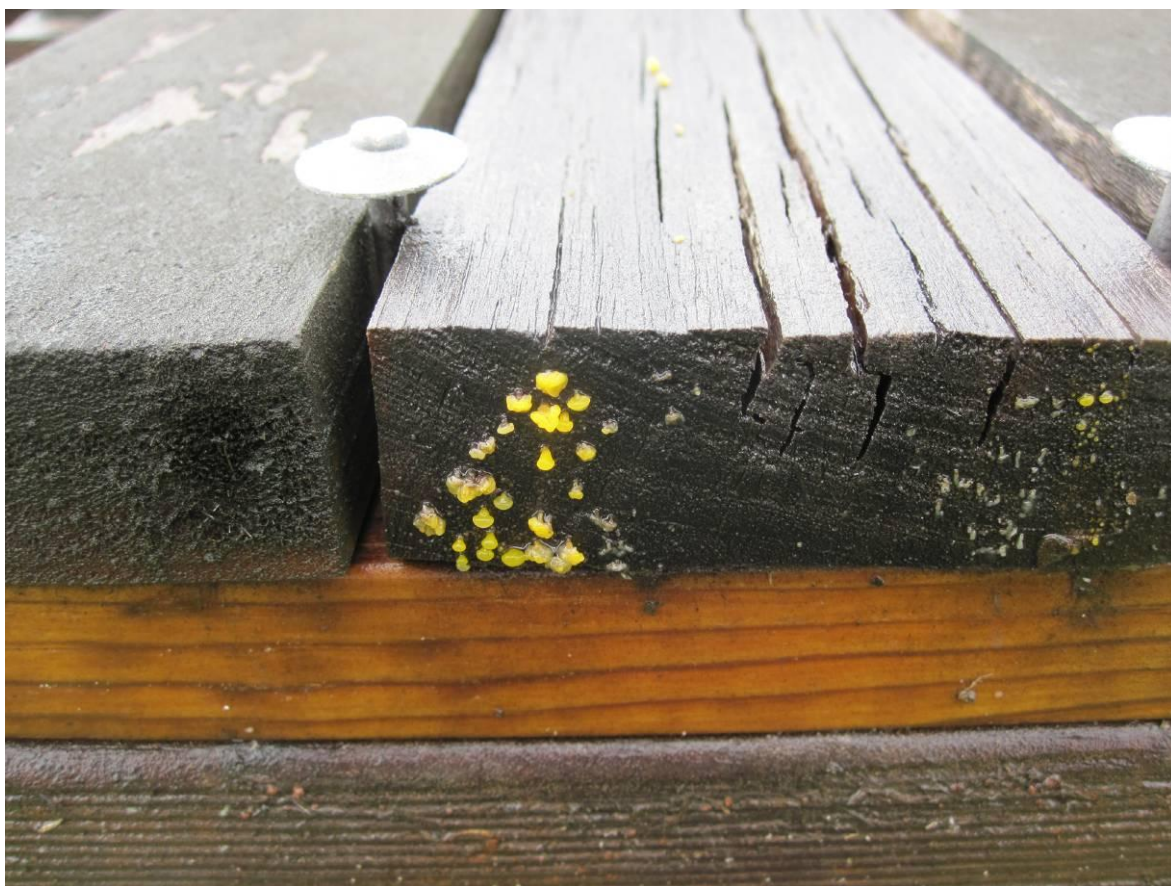
Figure 67. Fruiting bodies of the brown rotting fungus ( Heterotextus sp.) responsible for extensive decay in quarter azole-treated P. radiata test specimens in the raised deck test at Innisfail after three years.
