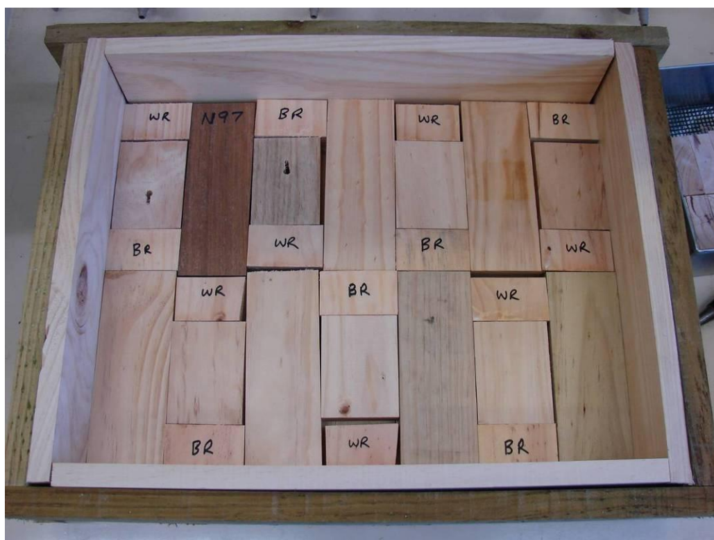
Figure 28. Second bottom layer of test specimens and pre-inoculated blocks for the Clayton AFS rot box, alternating with the bottom layer. WR = white rot and BR = Brown rot.
