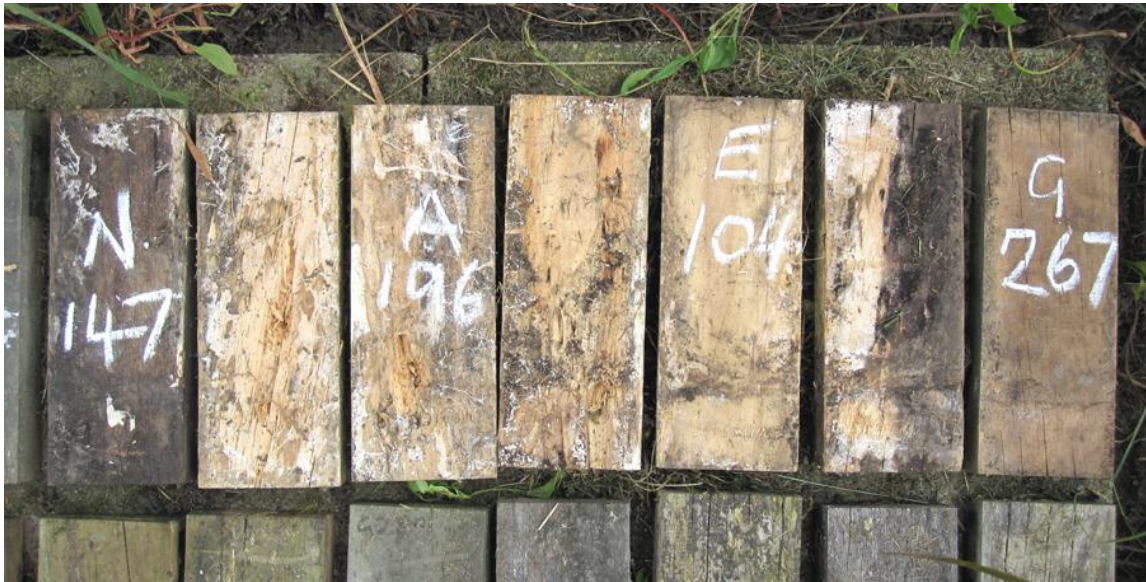
Figure 57. Ground proximity test at Rotorua after four years, underside. Left to right = N147 C. maculata rating 7, F263 TBTN rating 2, A196 water rating 2, J276 HKF rating 1, E104 ACQ rating 7, J279 HFK rating 6, G267 CCA rating 8.
