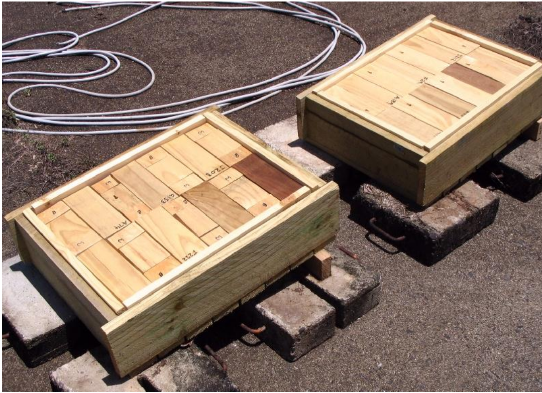
Figure 24. Rot boxes installed at Innisfail. Left box is pre-inoculated.
