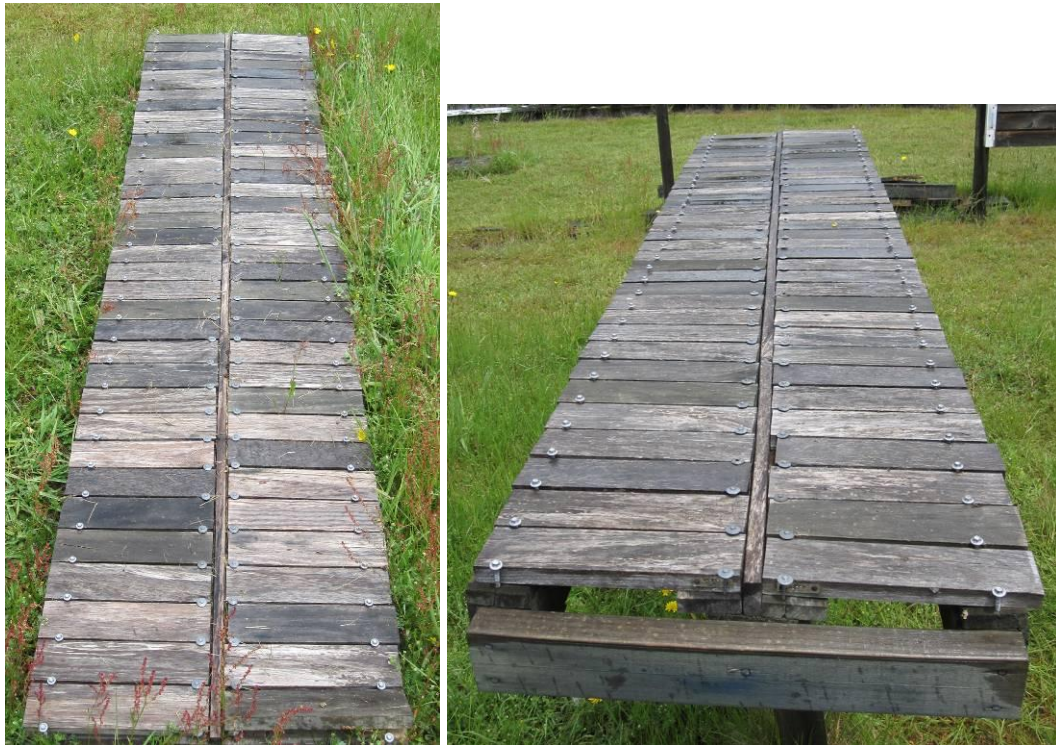
Figure 45. Decking tests at Rotorua after four years. Left, deck-on-grass. Right, raised deck.
