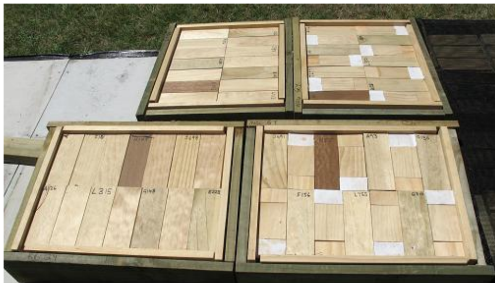
Figure 26. Rot boxes installed at Rotorua. The two boxes on the right were pre-inoculated.
