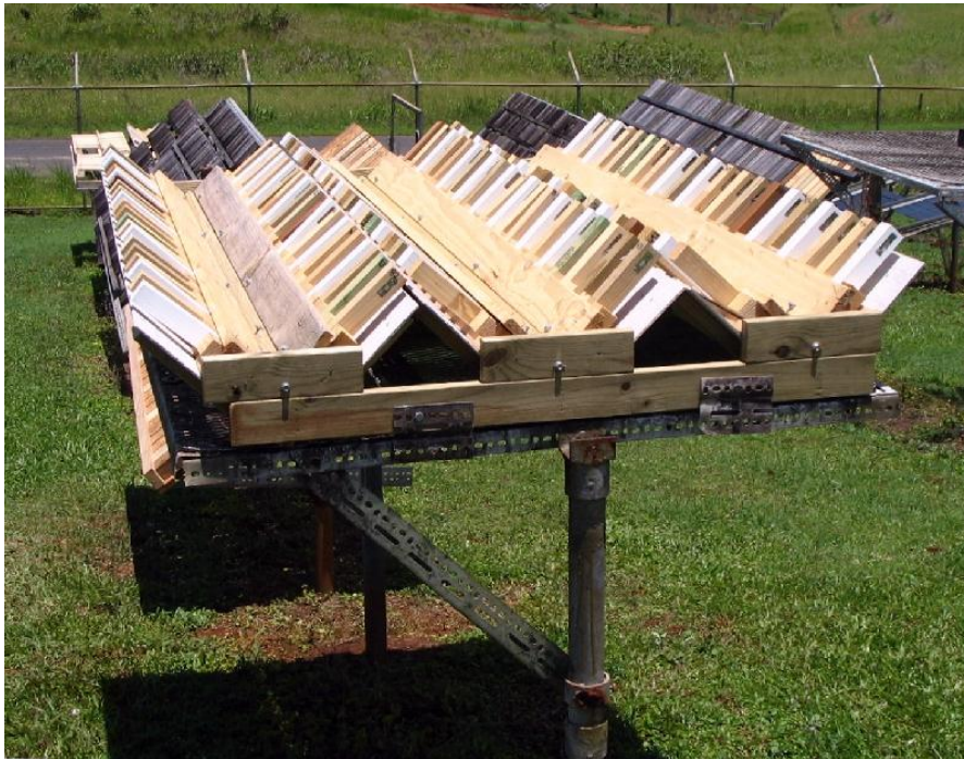
Figure 15. Embedded test installed at Innisfail, painted specimens randomized with A- and B-list test specimens
