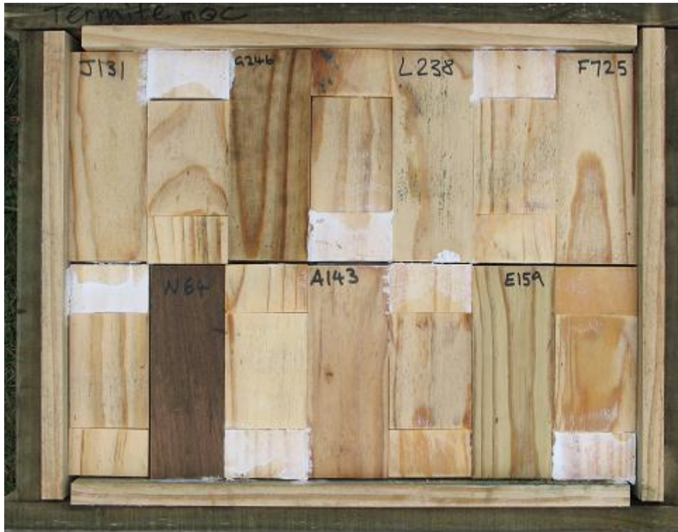
Figure 29. Pre-inoculated rot box from the Rotorua AFS after moving to the graveyard for summer exposure. Mould patches and O. placenta mycelium have developed on untreated separators and some of the test specimens.
