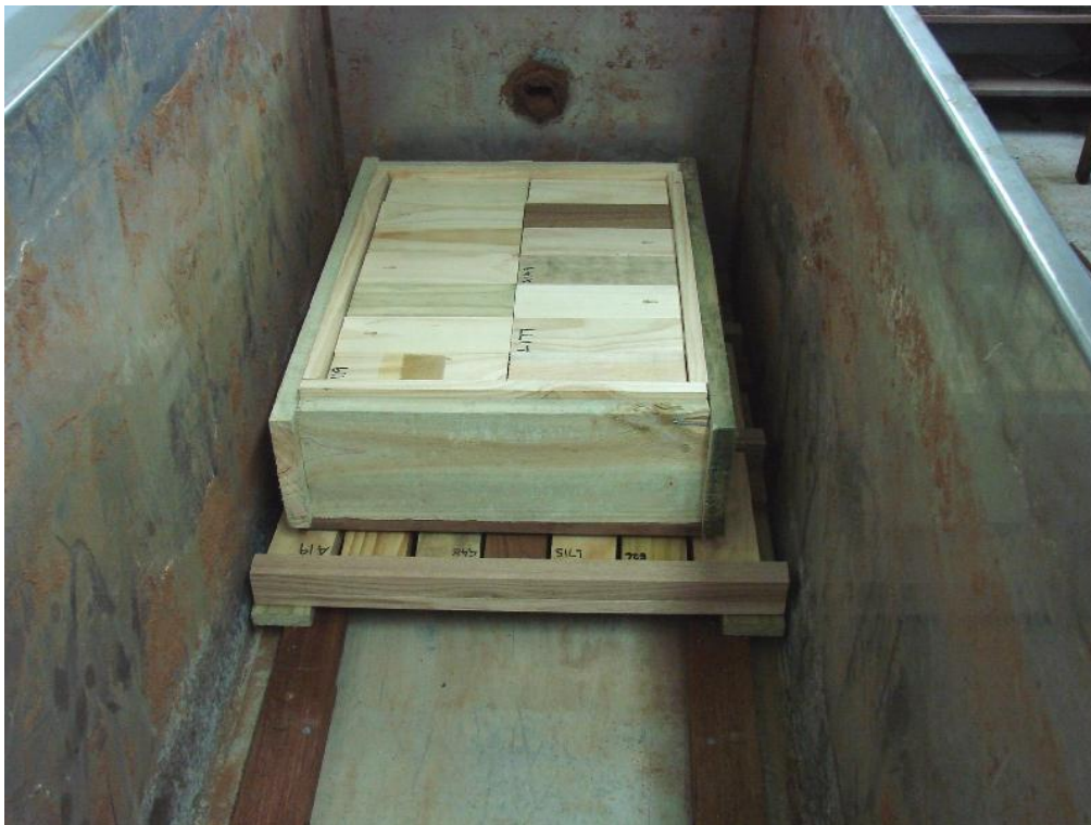
Figure 25. Rot box installed at Clayton AFS, resting upon a flat panel frame. Showing bottom rows in trough upon which other tests will be stacked.
