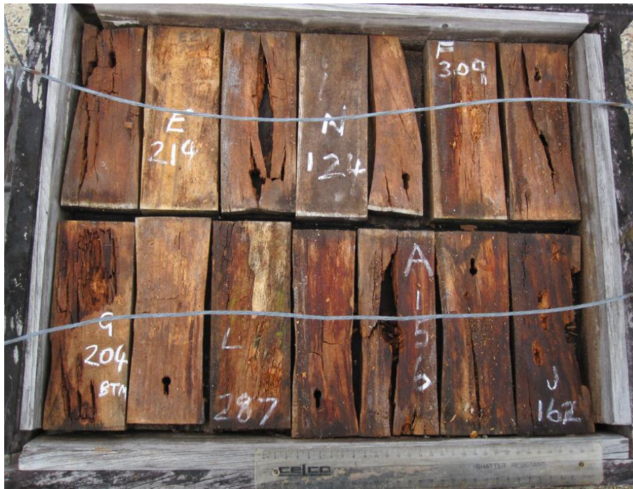
Figure 52. Rot box No 12 at Innisfail after four years, second top row, feeder bait blocks alternate with test specimens. Left to right = E219 ACQ rating 5, N124 C. maculata rating 7, F309 TBTN rating 4, G204 CCA rating 0, L287 azoles rating 3, A156 water rating 0, J162 HFK rating 0.
