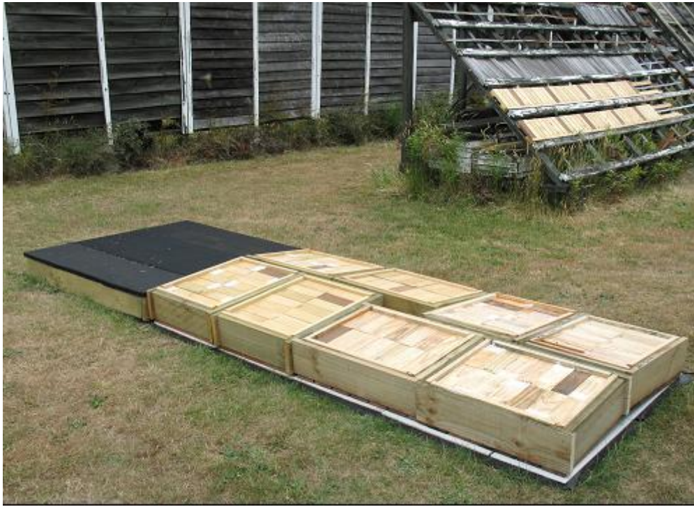
Figure 2. General view at Rotorua of rot boxes, ground proximity (covered with black shade cloth) and flat panel tests (top right) on 5 December 2007, after rot boxes from the termite house were moved to the graveyard test area for summer exposure.
