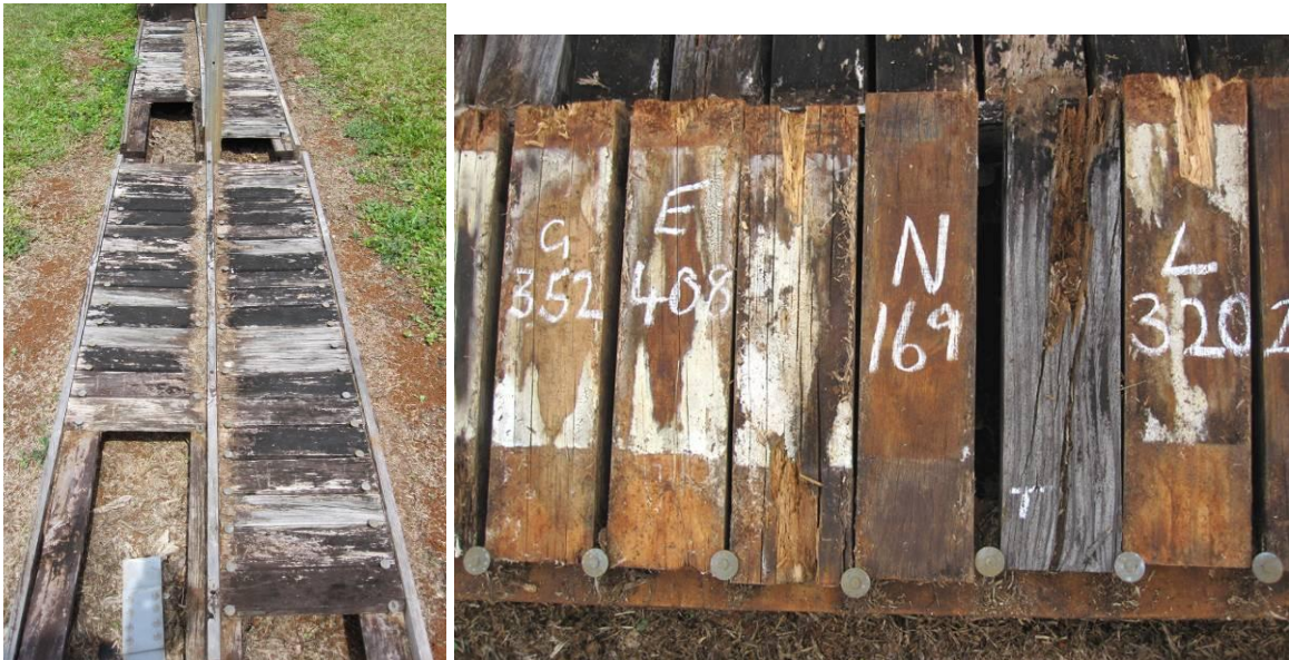
Figure 46. Deck-on-grass at Innisfail after four years. Left photo, note dead grass accumulated along centre board on top of specimens. Right photo, left to right undersides = G352 CCA rating 0, E408 ACQ rating 1, F373 TBTN rating 0, N169 C. maculata rating 8, A230 (top side) rating 0, L320 azoles rating 0.
