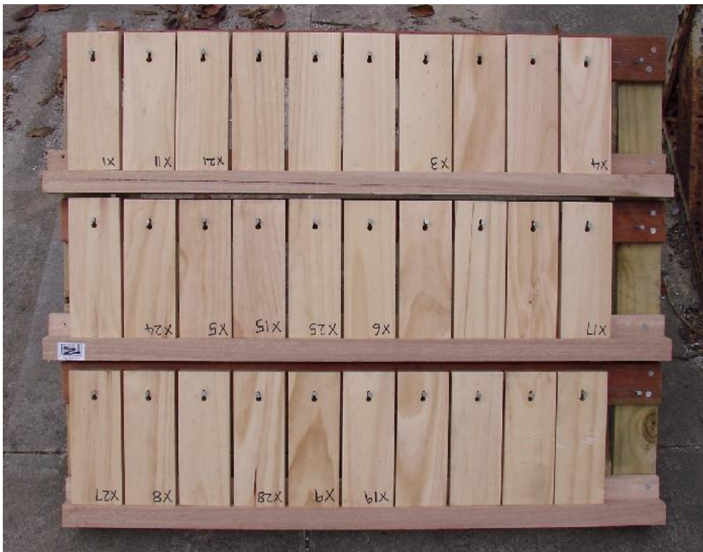
Figure 5. Flat panel test installed of water monitoring specimens at Clayton, on new frame.
