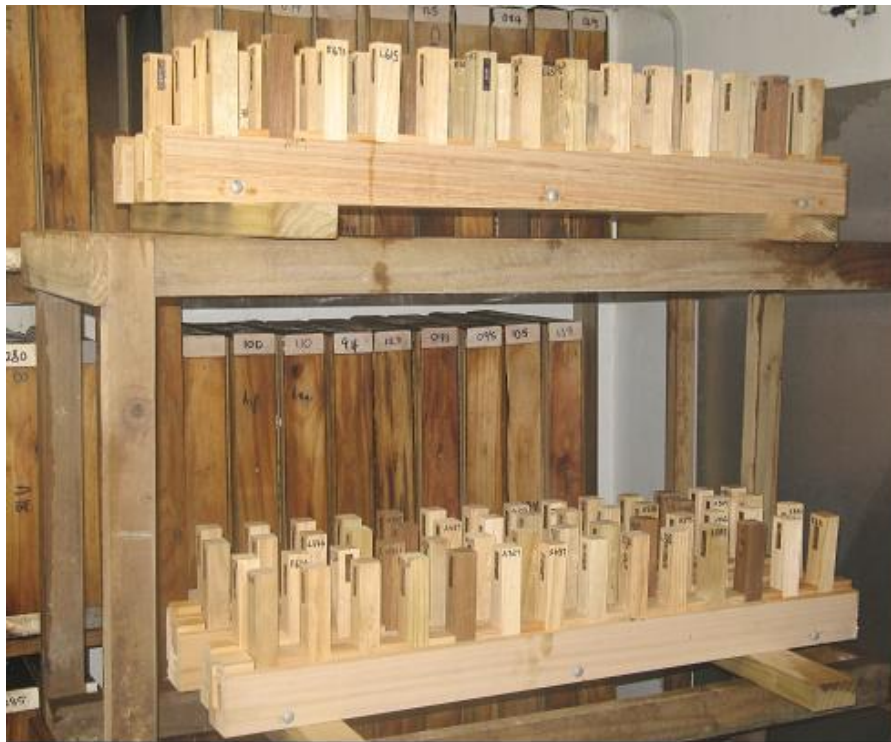
Figure 17. Embedded tests on racks in Rotorua AFS.
