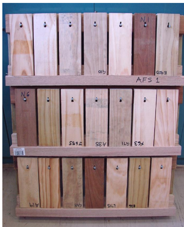
Figure 7. One of the flat panel test frames installed at Clayton AFS.
