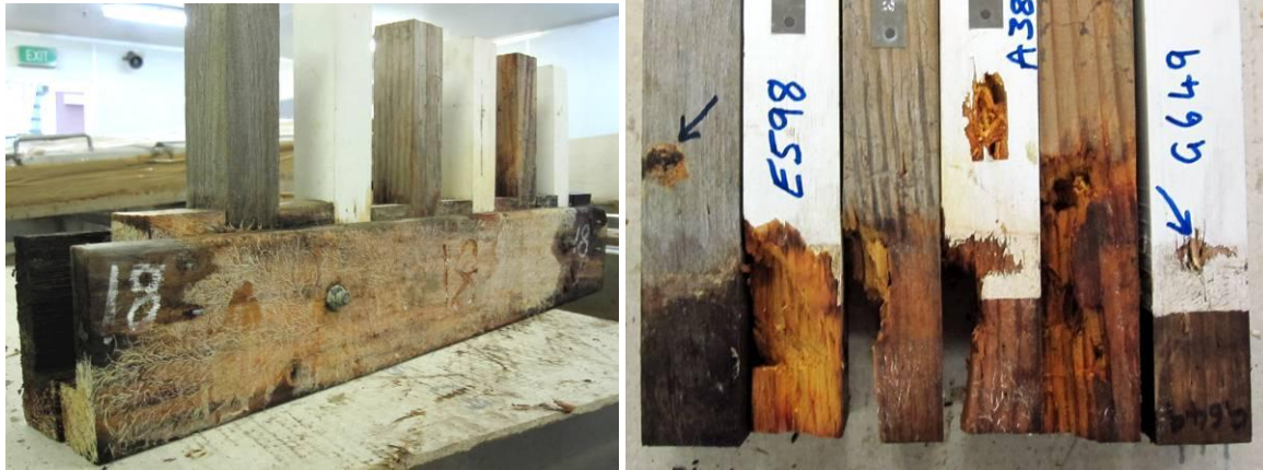
Figure 50. Embedded test in AFS at Clayton after four years, frame 18. Left photo, showing mycelium growing over base holder (white areas). Right photo, left to right = N320 C. maculata rating 8 (with fruiting body on side), E598 ACQ rating 0, A323 water rating 0, A389 water rating 0, E690 ACQ rating 0, G649 CCA rating 6.
