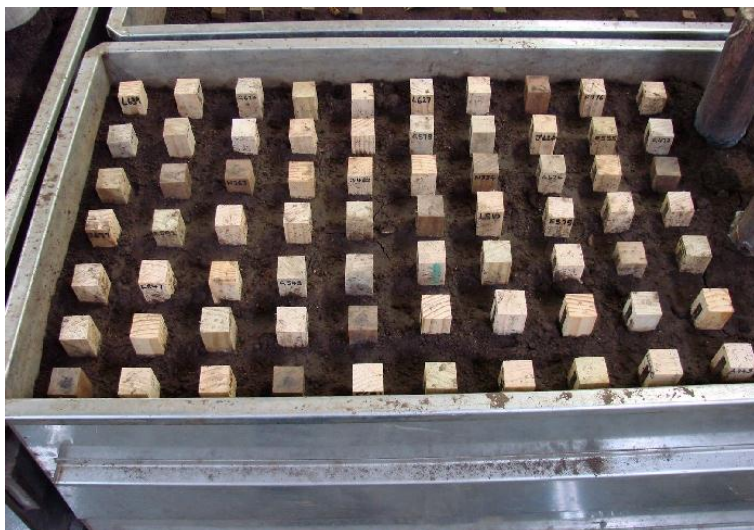
Figure 37. In-ground stakes installed in the Clayton AFS.
