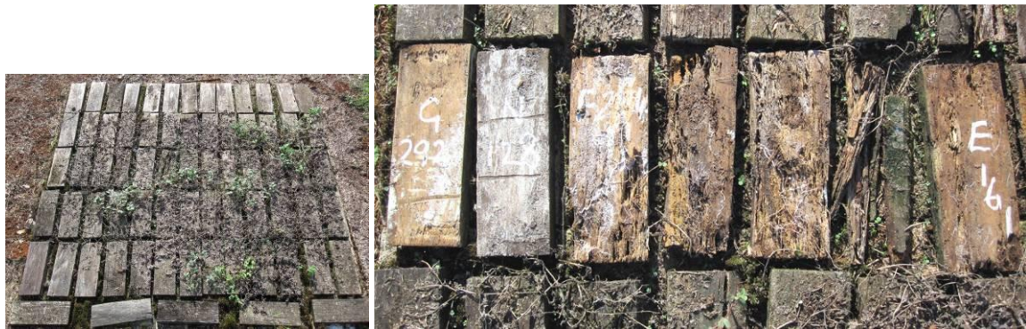
Figure 55. Ground proximity test at Innisfail after four years. Left to right = G292 CCA rating 6, N128 C. maculata rating 7, F224 TBTN rating 0, J224 HFK rating 0, L232 azoles rating 0, A122 water rating 0 (nearly disintegrated), E161 ACQ rating 0.
