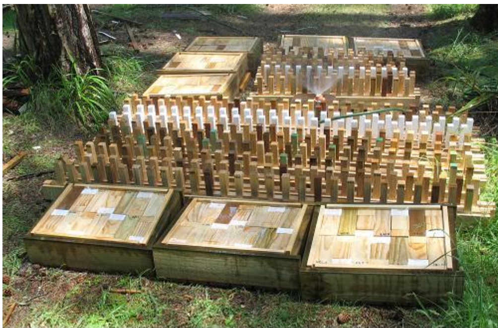
Figure 20. Rot boxes and embedded tests (pre-inoculated or not) at Rotorua under water spray for 1.5 hours prior to placement in the AFS or field.
