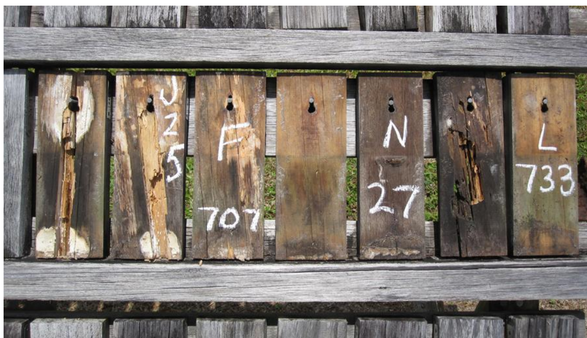
Figure 43. Flat panel test on new frame at Innisfail after four years, underside. Left to right = E32 ACQ rating 0, J25 HFK rating 0, F707 TBTN rating 4, G30 CCA rating 7, N27 C. maculata rating 8, A38 water rating 0, L733 azoles rating 7.
