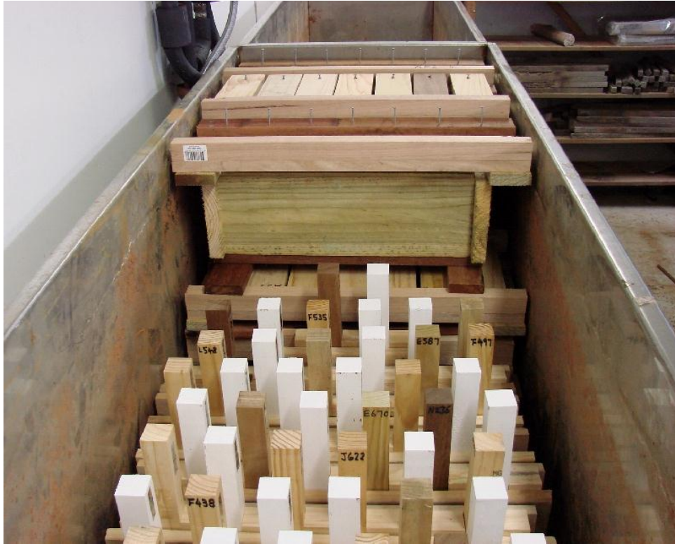
Figure 8. Embedded test (foreground), rot box and flat panel test installed within steel troughs in the Clayton AFS.
