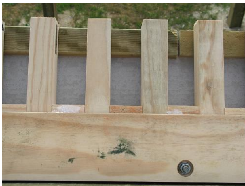
Figure 21. Pre-inoculated embedded test at Rotorua AFS when installed for summer exposure in graveyard on 5 December 2007. Note mycelium from the pre-inoculated blocks spreading up over the surface of the holders.
