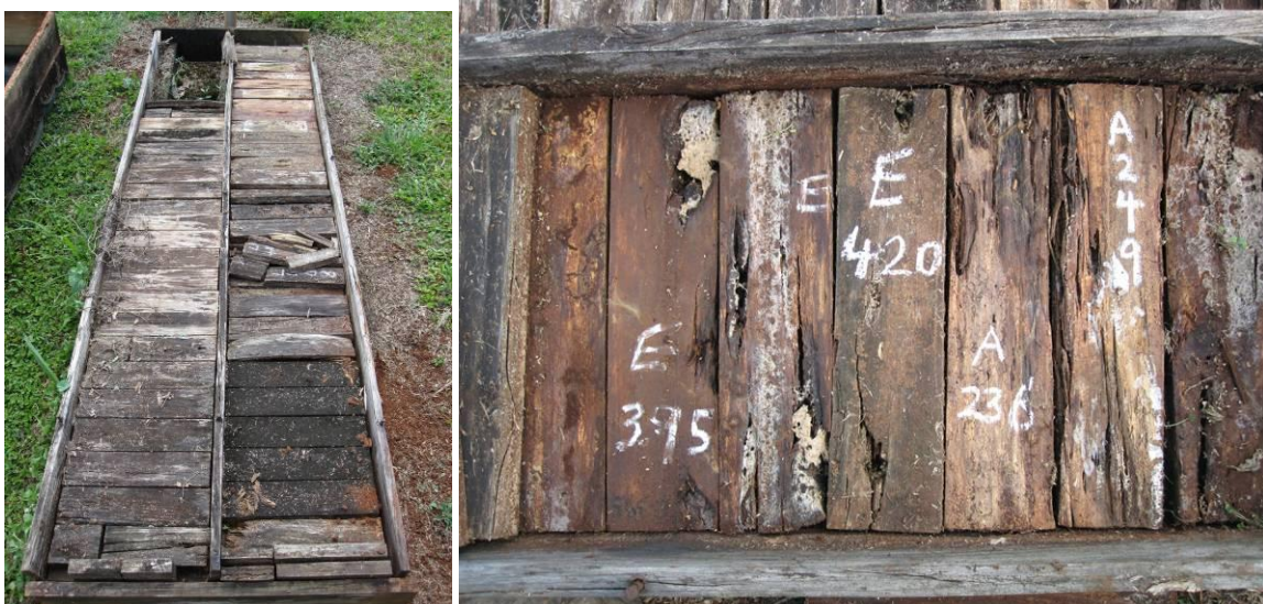
Figure 58. Double layer test at Innisfail after four years. Right, bottom right column shows set of darker C. maculata specimens rating 7 or 8, middle right column azoles (jumbled) all rating 0. Left, bottom layer of E specimens (ACQ) all rating 0, and A specimens (water) all rating 0 (spare blocks separating treatments removed for photo).
