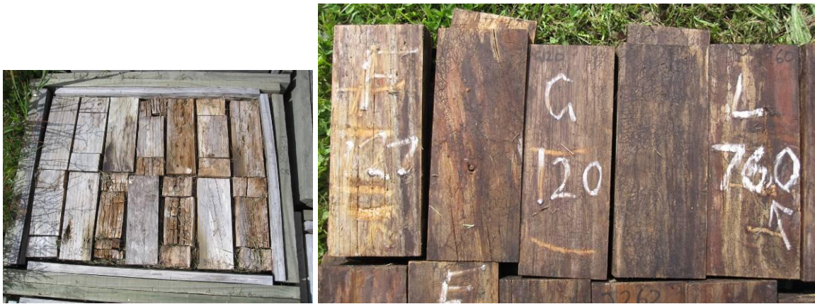
Figure 54. Rot boxes in AFS at Rotorua after four years (during summer exposure outdoors). Right Box No. 8 pre-inoculated showing brown rotted feeder blocks between test specimens. Left Box No. 5 not inoculated, left to right = F127 TBTN rating 7, feeder, G120 CCA sound, feeder, L760 azoles rating 6.
