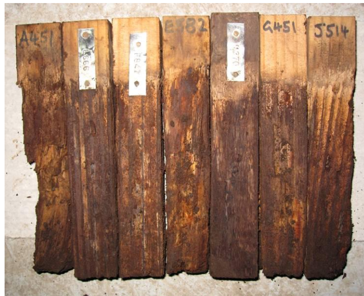
Figure 61. In-ground stake in Clayton AFS after four years. Left to right = A451 water rating 0, L666 azoles rating 5, F847 TBTN rating 3, E582 ACQ rating 3, N370 C. maculata rating 7, G451 CCA rating 3, J514 HFK rating 0.
