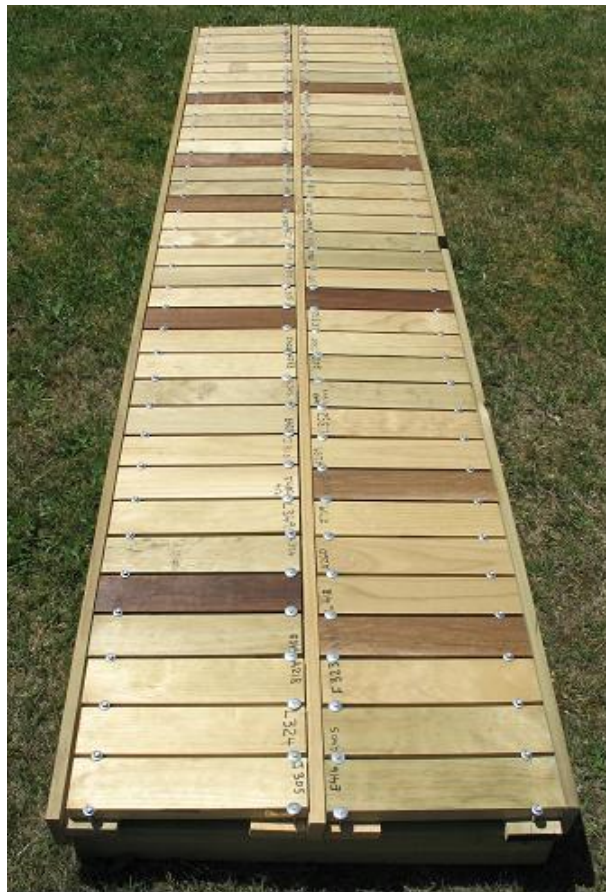
Figure 11. Deck-on-grass installed at Rotorua.
