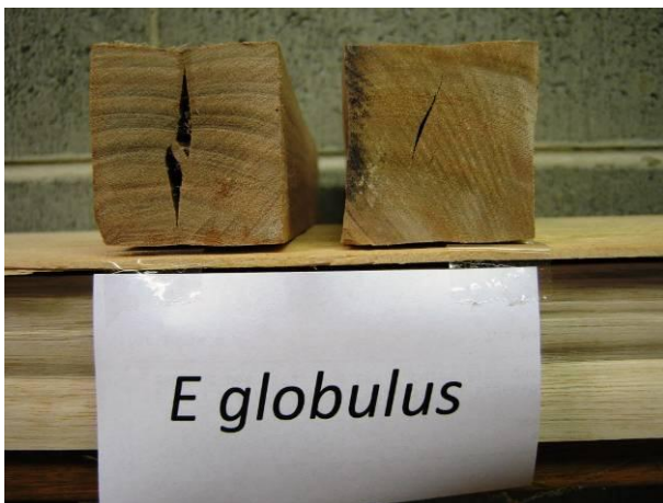
Figure 27 Collapse & distortion in E. globulus
