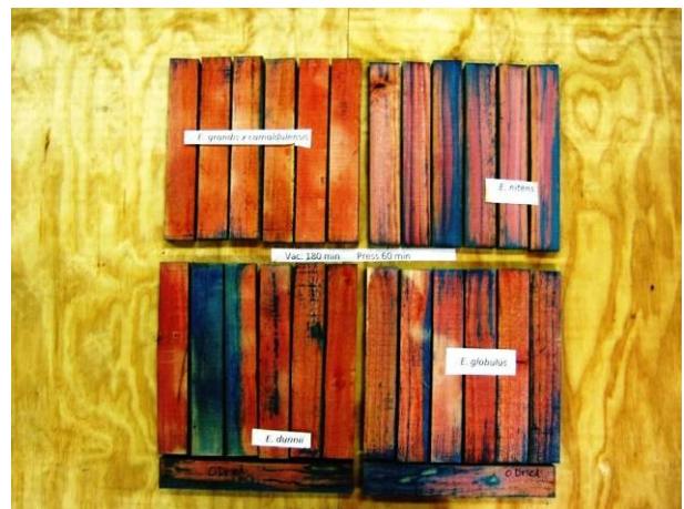
Figure 37 Copper penetration after schedule #6
