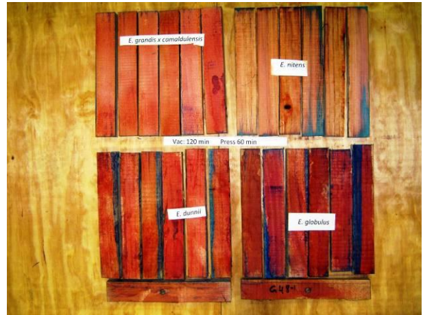
Figure 33 Copper penetration after schedule #2
