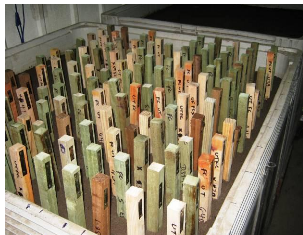
Fungal cellar exposure
