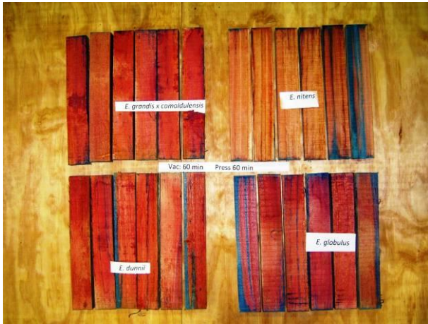
Figure 32 Copper penetration after schedule #1
