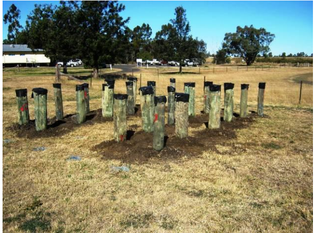
Figure 48 Stub layout Dalby - decay
