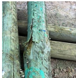
Really bad debarking damage – will need to be addressed if the species is to be used as poles
