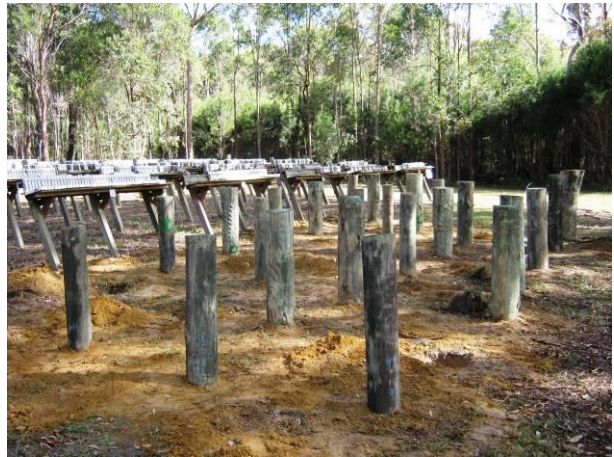
Figure 20 Stub layout Redlands - decay
