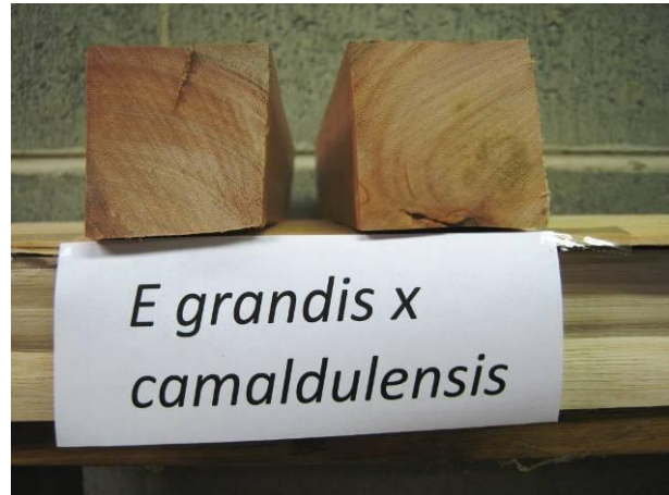
Figure 26 Distortion in E. grandis x camaldulensis
