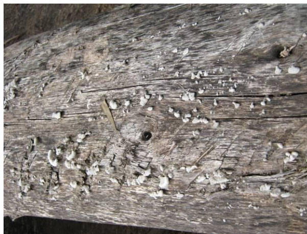
Figure 14 Fruiting bodies on the surface of E. globulus poles before treatment
