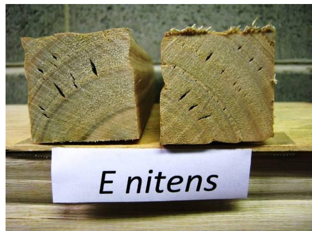
Figure 28 Collapse & distortion in E. nitens
