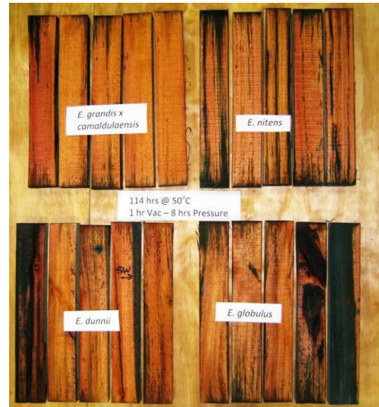
Figure 39 Copper penetration after schedule #8
