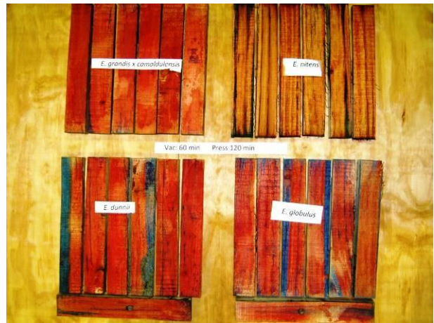
Figure 35 Copper penetration after schedule #4
