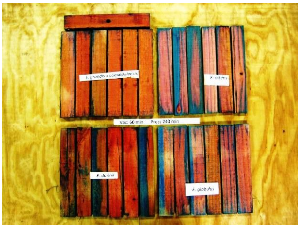
Figure 36 Copper penetration after schedule #5
