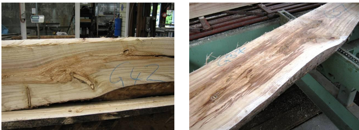
Figure 29 Internal decay in E. globulus
