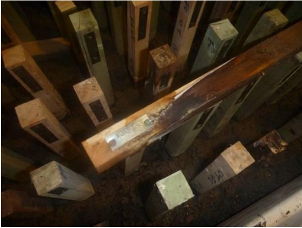
Figure 42 Saturated untreated P. elliotii stake
