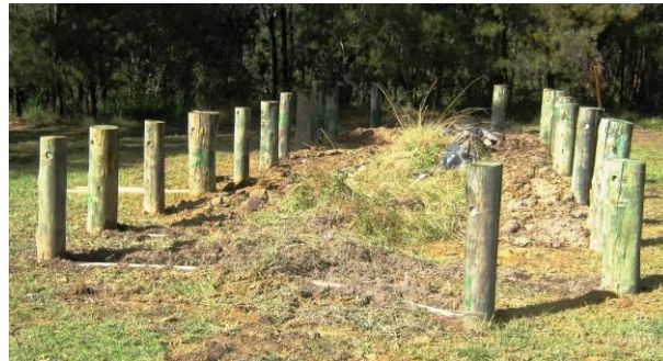
Figure 46 Stub layout Redlands - termites
