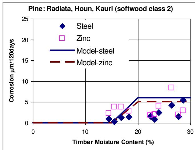
Figures 3.3.1 Check of the model with 120-day corrosion of nails in softwood class 2 timber. Data from Table 3.3.1. Model Equation is (1.5.2).
