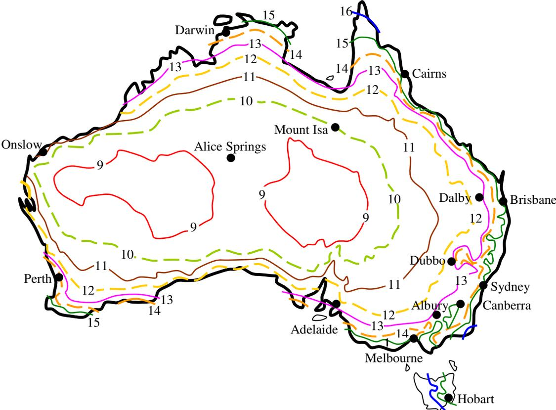
**Figure 1.3.3.** Annual mean surface moisture content of timber outdoors.
