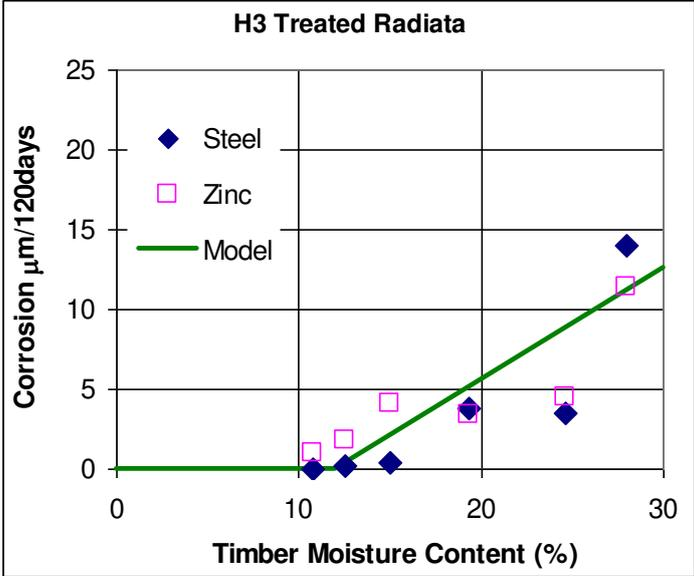
Figures 3.3.5 Check of the model with 120-day corrosion of nails in H3 CCA-treated Radiata pine. Data from Table 3.3.1. Model Equation is (1.6.3).
