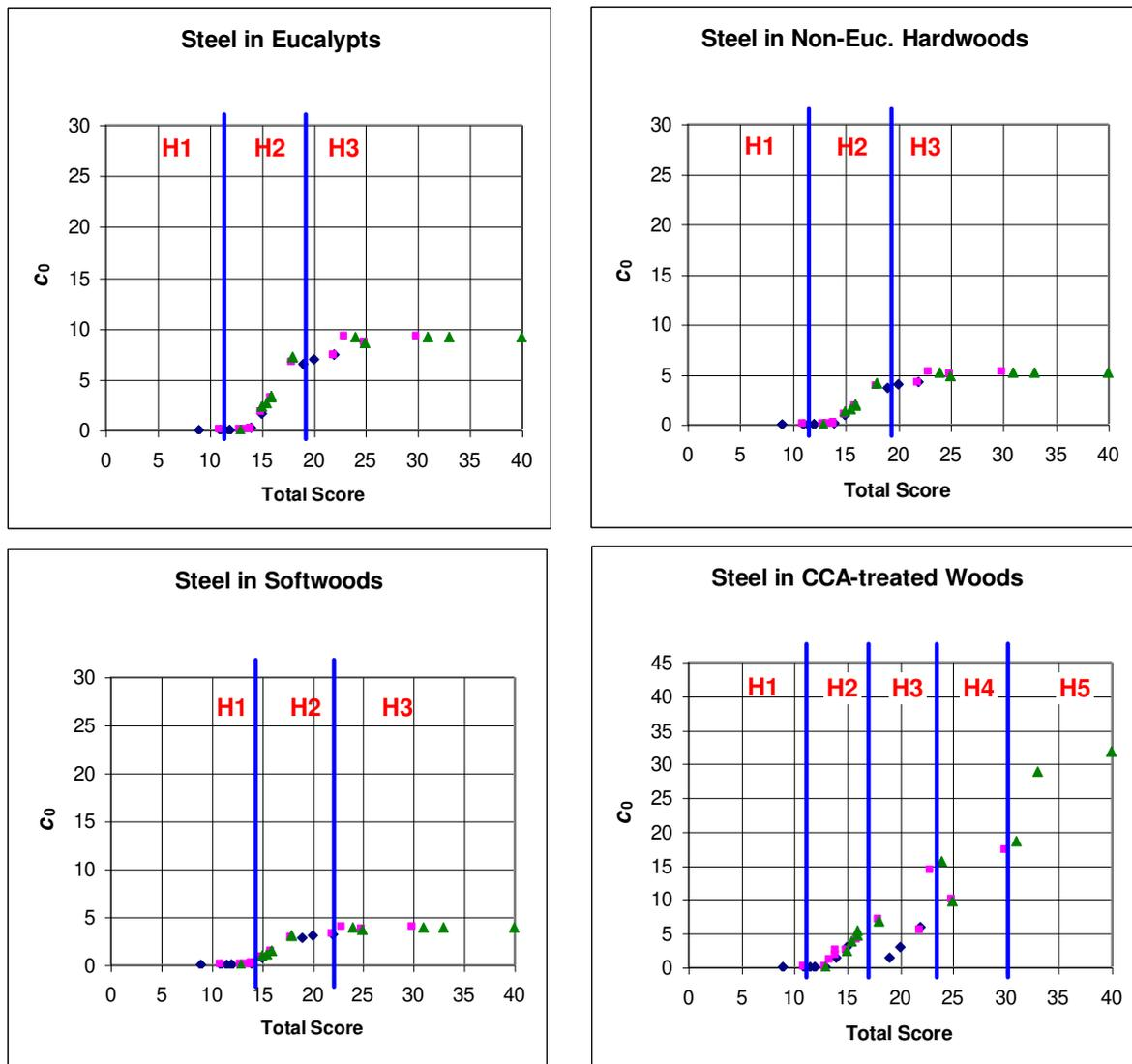
**Figure 4.2.2.** Hazard ratings for steel fasteners embedded in different types of wood (Data from Appendix B)
