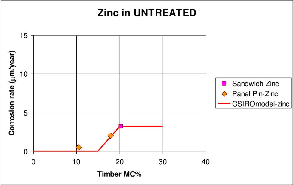
Figures 3.2.1 Comparison of the model prediction of corrosion rate (Eq.(1.5.1)) vs timber MC with BRANZ test data for zinc in untreated Radiata pine (Table 3.2.1)
