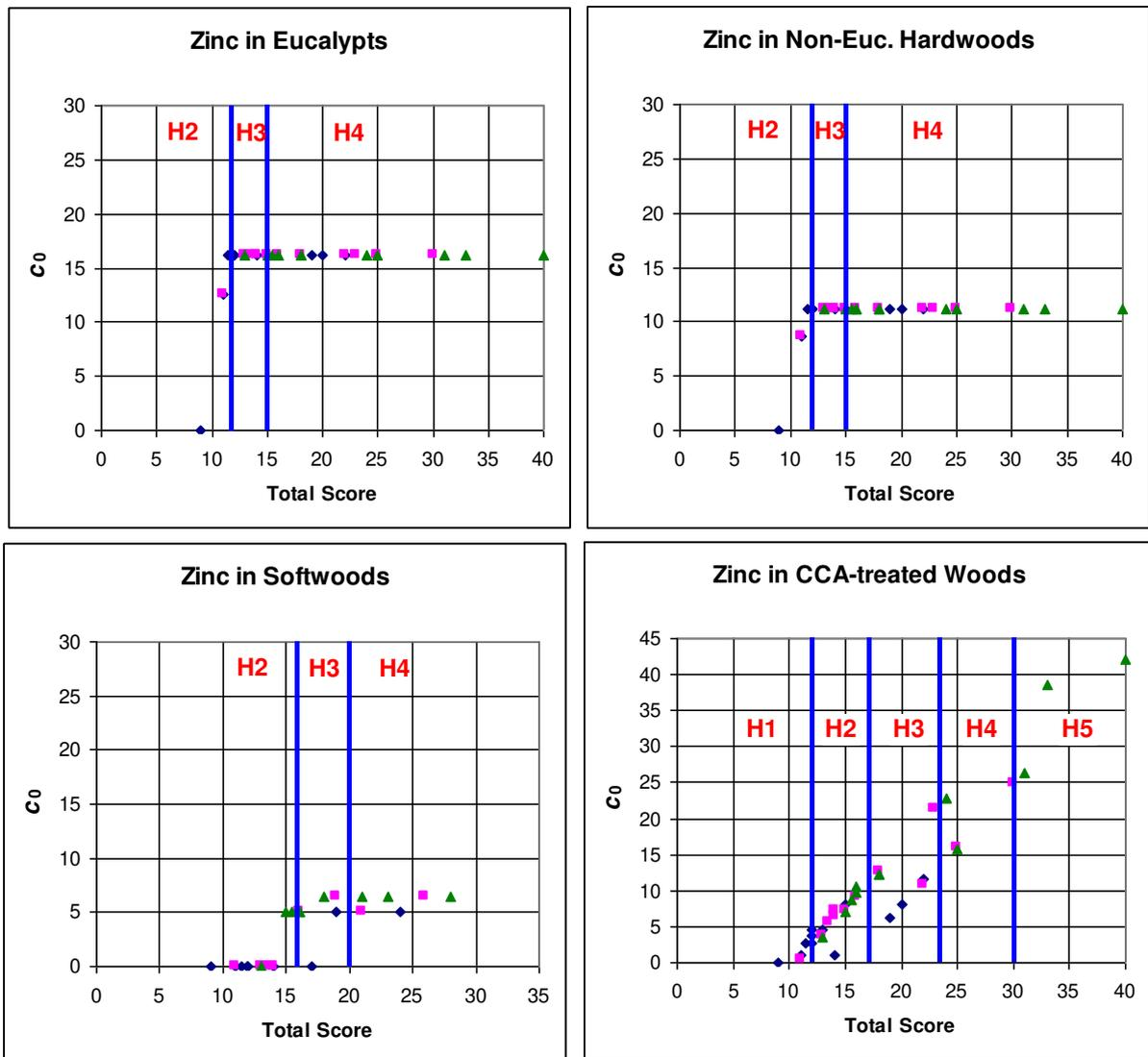
**Figure E.2.1.** Hazard ratings for zinc fasteners embedded in different types of wood
