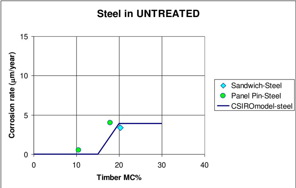
Figures 3.2.2 Comparison of the model prediction of corrosion rate (Eq.(1.5.1)) vs timber MC with BRANZ test data of steel in untreated Radiata pine (Table 3.2.1)
