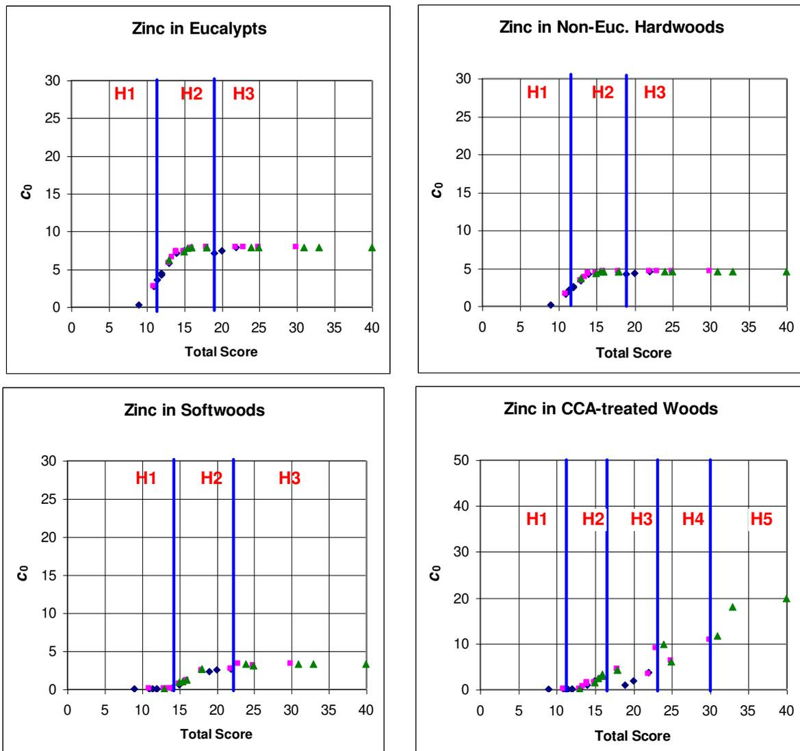
**Figure 4.2.1.** Hazard ratings for zinc fasteners embedded in different types of wood (Data from Appendix B)
