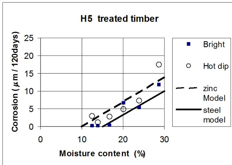
**Figure C.4.3** Comparison of corrosion model for embedded metal, with test data for CCA treated Radiata pine.
