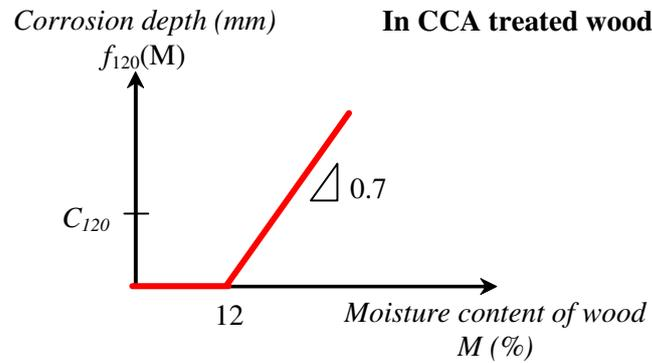
**Figure 5.2.4.1.** Base model of embedded corrosion in CCA-treated wood.
