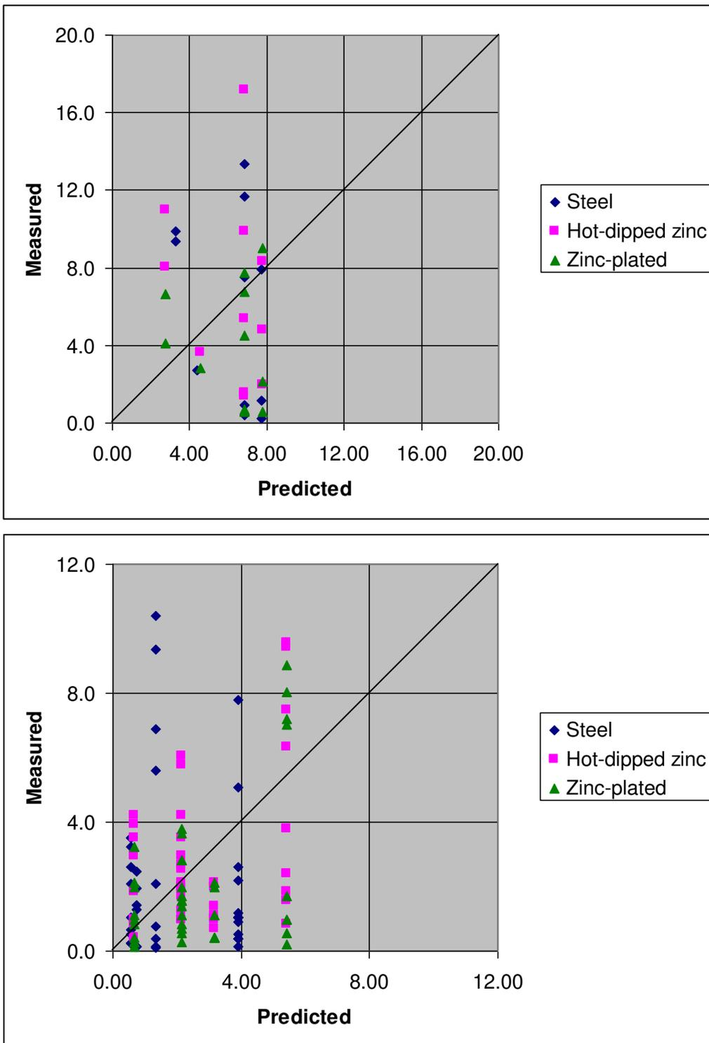
**Figure 3.1.2.2** Checks with *outdoor 2-year embedded nails individual data* using the current model. Top: Marine sites, Bottom: Non-marine sites
