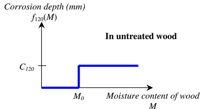
**Figure D.4.1.1.** Base model of embedded corrosion in untreated wood.
