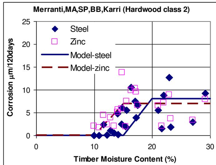
Figures 3.3.3 Check of the model with 120-day corrosion of nails in hardwood class 2 timber. Data from Table 3.3.1. Model Equation is (1.5.2).
