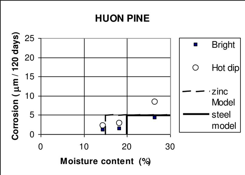
**Figure C.4.2 (cont)** Comparison of corrosion model for embedded metal, with test data for softwood timber.
