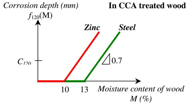
**Figure D.4.2.1.** Base model of embedded corrosion in CCA-treated wood.
