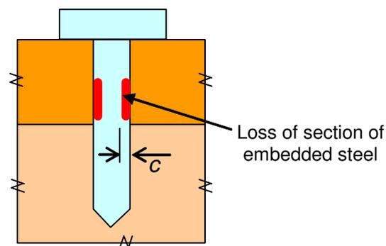
Figure 5.2. 1 Embedded corrosion depth
