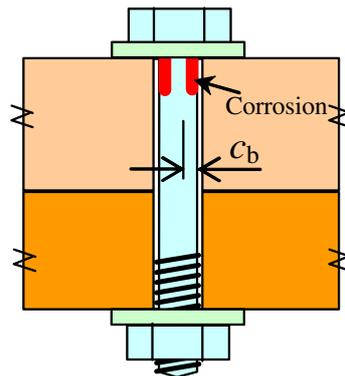
**Figure 5.3.1** Depth of corrosion at the neck of the bolt
