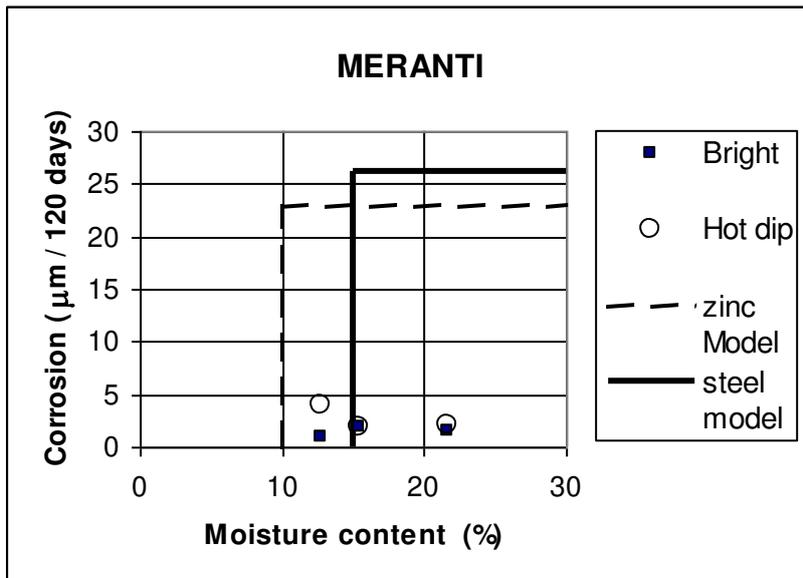
**Figure C.4.1 (cont)** Comparison of corrosion model for embedded metal, with test data for hardwoods.
