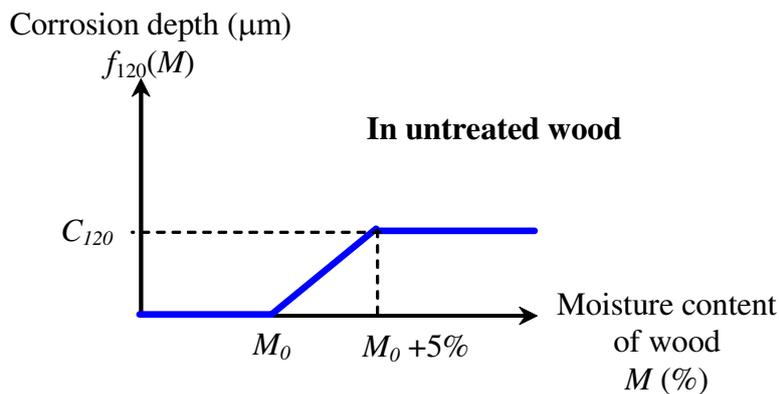
**Figure 1.5.1.** Base model of embedded corrosion in untreated wood.
