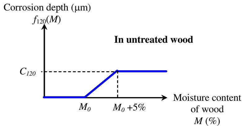
**Figure 5.2.3.1.** Base model of embedded corrosion in untreated wood.
