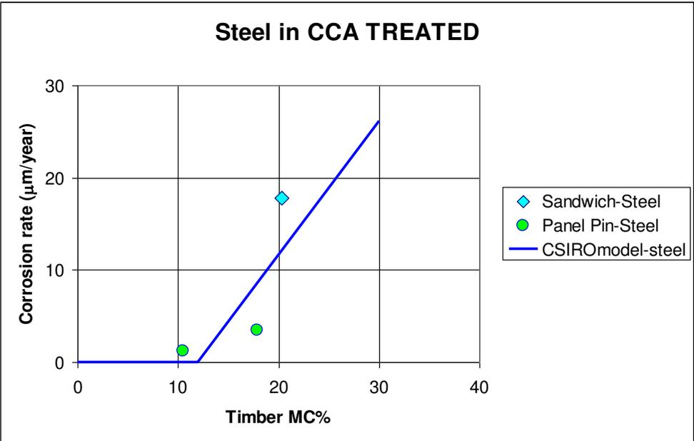
Figures 3.2.4 Comparison of the model prediction of corrosion rate (Eq.(1.6.2)) vs Timber MC with BRANZ test data of steel in treated Radiata pine (Table 3.2.1)
