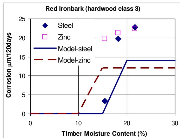
Figures 3.3.4 Check of the model with 120-day corrosion of nails in hardwood class 3 timber. Data from Table 3.3.1. Model Equation is (1.5.2).
