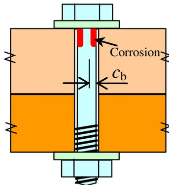
**Figure 1.8.1** Depth of corrosion at the neck of the bolt
