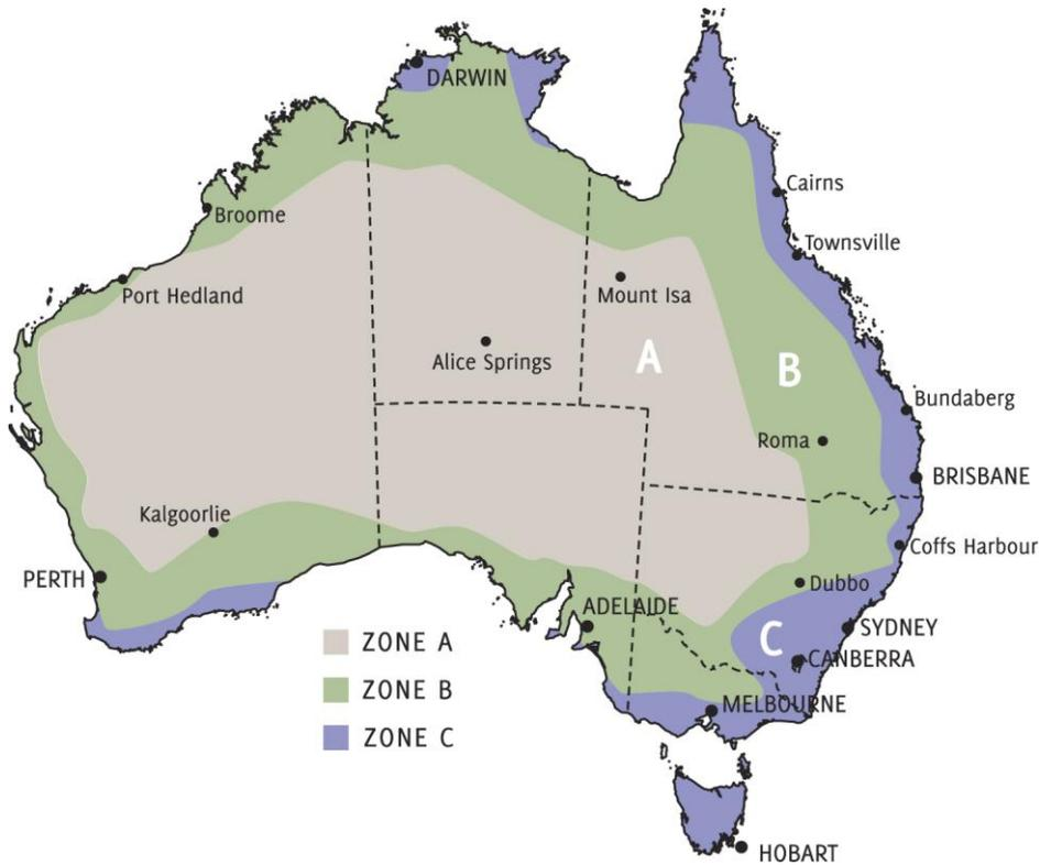
**Figure D.1.2.** Modified Hazard zone map based on effective  $SEMC_{mean}$  - currently used in the Compendium.
