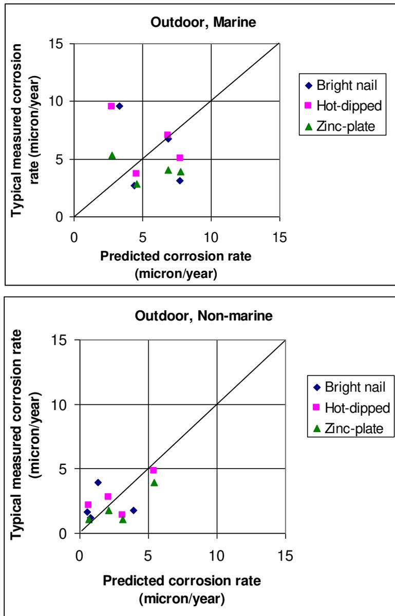
**Figure 3.1.2.1** Checks with outdoor 2-year embedded nails group-averaged data using the current model . Top: Marine sites, Bottom: Non-marine sites
