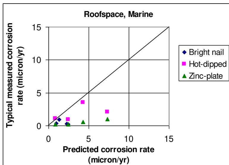
**Figure 3.1.2.1** Checks with 2-year embedded nails in roof-space using the current model
