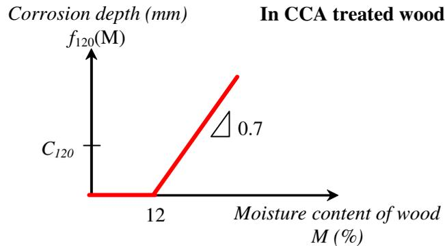
**Figure 2.4.2.1.** Base model of embedded corrosion in CCA-treated wood.
