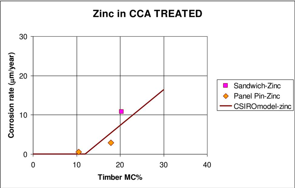
Figures 3.2.3 Comparison of the model prediction of corrosion rate (Eq.(1.6.1)) vs Timber MC with BRANZ test data of zinc in treated Radiata pine (Table 3.2.1)
