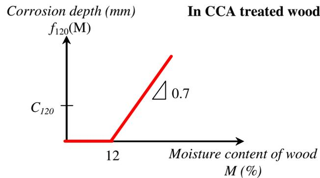
**Figure 1.6.1.** Base model of embedded corrosion in CCA-treated wood.
