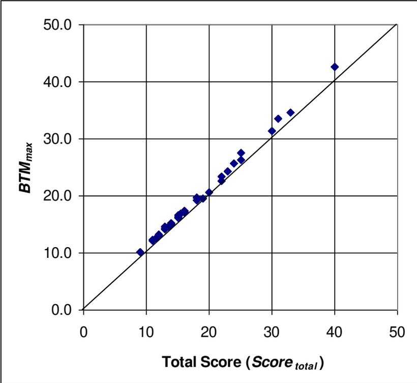
**Figure A.1.** Maximum moisture content of timber in buildings ( $BTM_{max}$ ) versus total score ( $Score_{total}$ ) – Data is from Table B.1, Appendix B.
