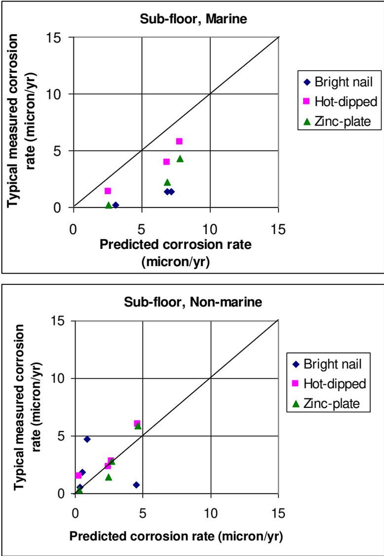
**Figure 3.1.2.1** Checks with outdoor 2-year embedded nails in sub-floor using the current model . Top: Marine sites, Bottom: Non-marine sites
