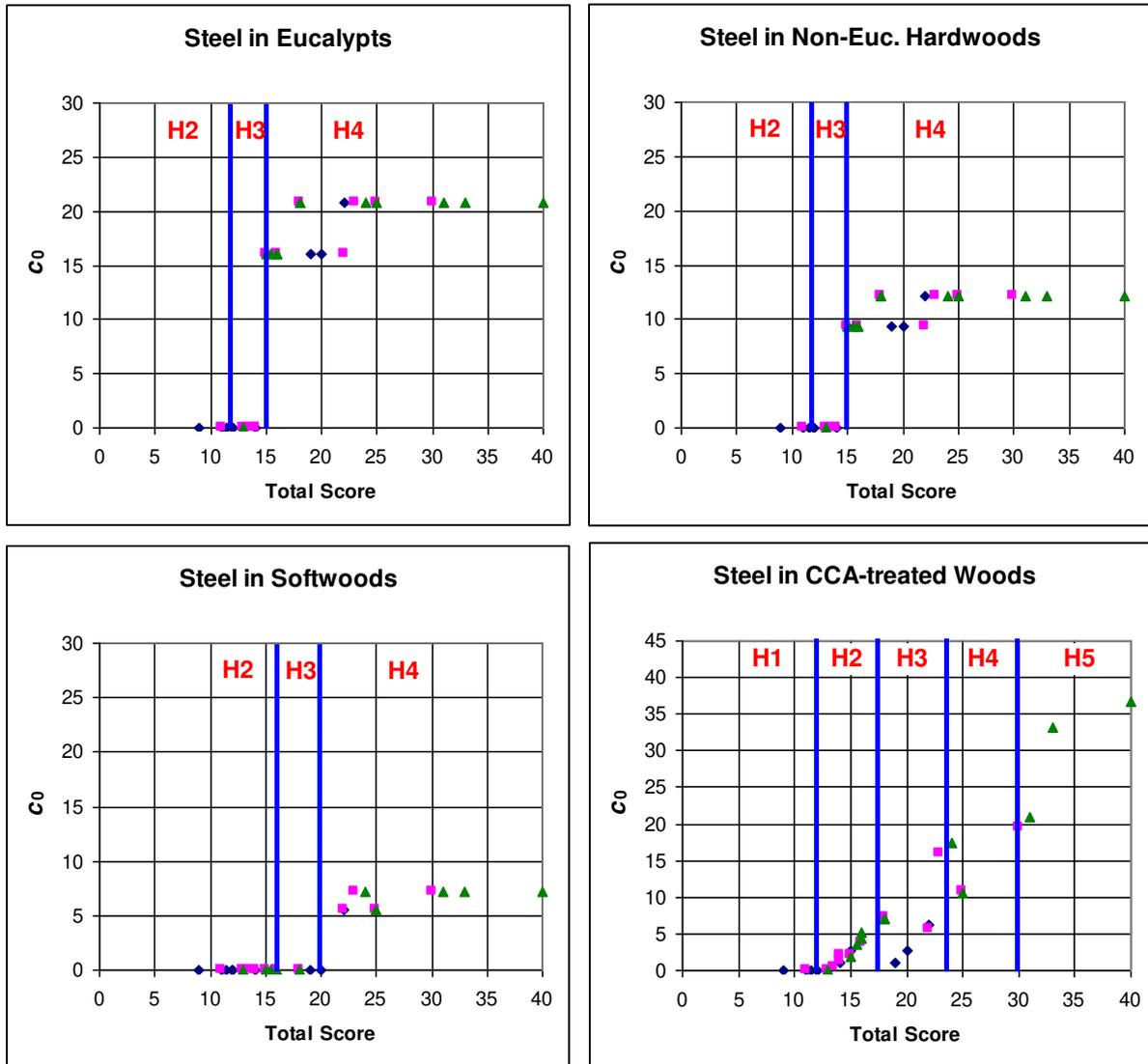
Figure E.2.2. Hazard ratings for steel fasteners embedded in different types of wood
