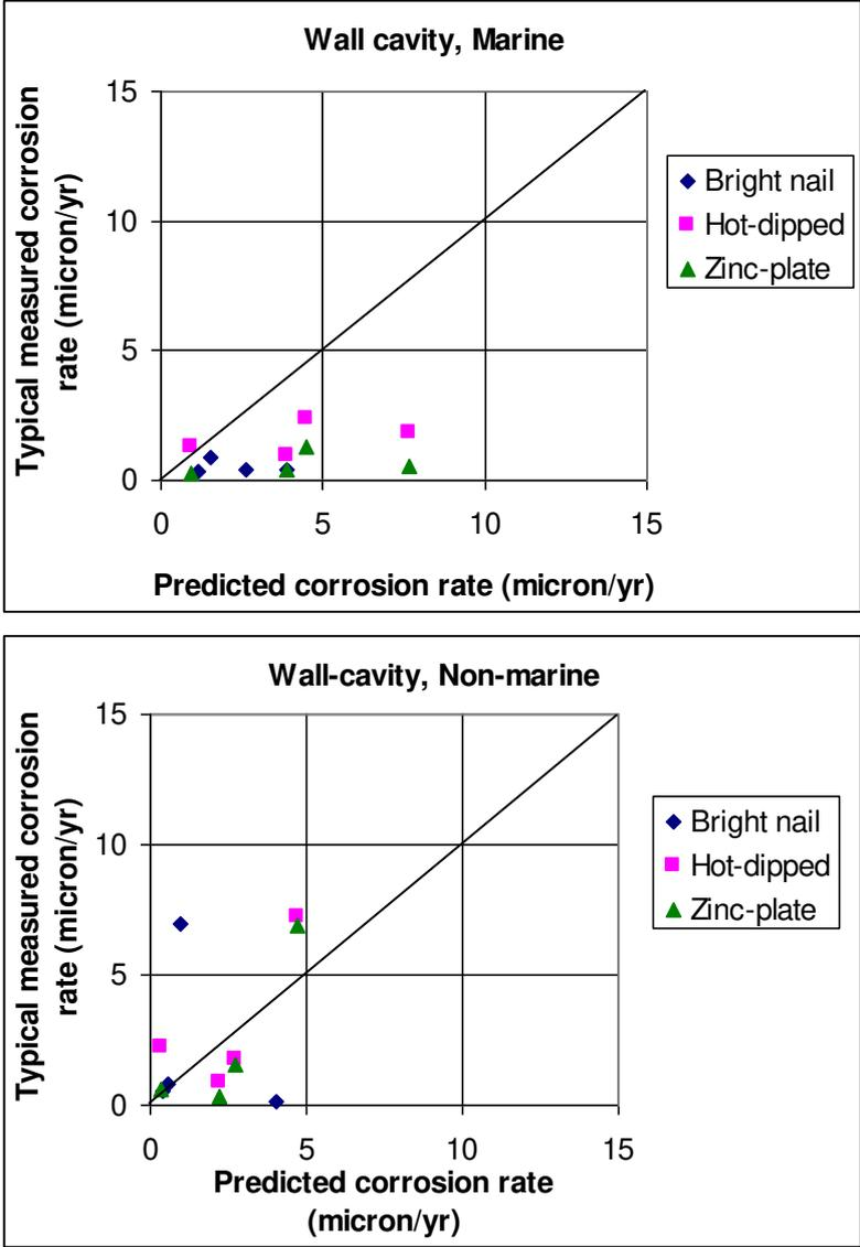
Figure 3.1.2.1 Checks with outdoor 2-year embedded nails in wall cavity using the current model . Top: Marine sites, Bottom: Non-marine sites
