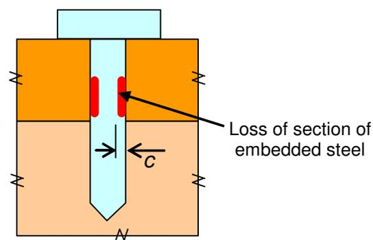
Figure 1.2.1 Embedded corrosion depth
