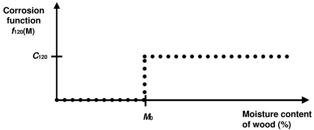
Figure C.3.1. Corrosion function  $f_{120}(M)$  for timber embedded in untreated wood.
