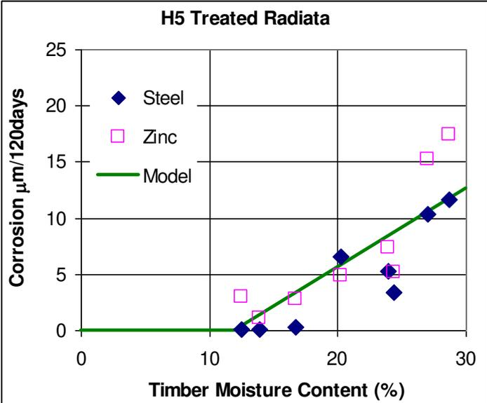
Figures 3.3.6 Check of the model with 120-day corrosion of nails in H5 CCA-treated Radiata pine. Data from Table 3.3.1. Model Equation is (1.6.3).
