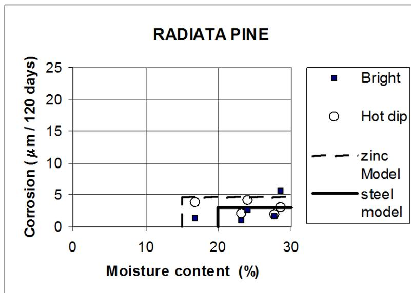
**Figure C.4.2** Comparison of corrosion model for embedded metal, with test data for softwood timber.
