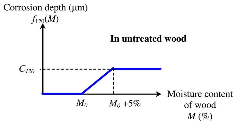
**Figure 2.4.1.1.** Base model of embedded corrosion in untreated wood.
