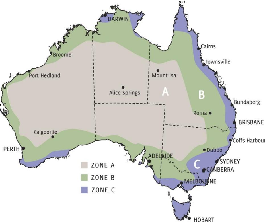
**Figure 1.3.1** Embedded corrosion hazard zone map. Zone C is most hazardous.
