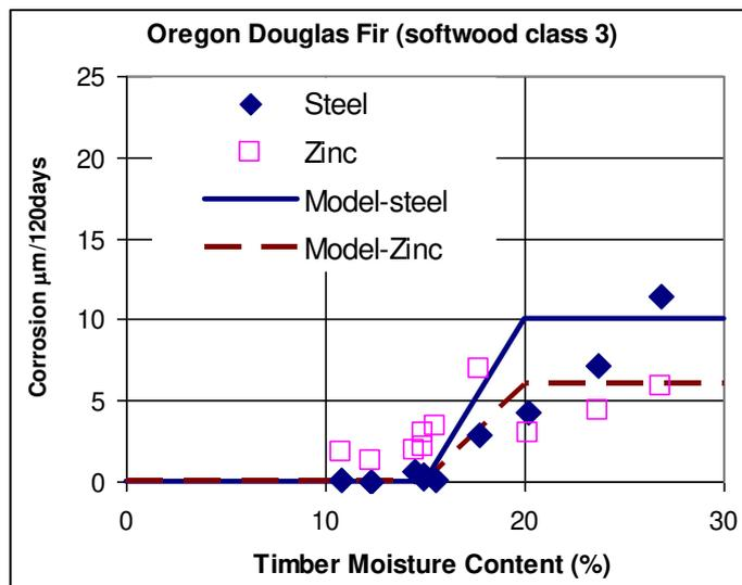
Figures 3.3.2 Check of the model with 120-day corrosion of nails in softwood class 3 timber. Data from Table 3.3.1. Model Equation is (1.5.2).
