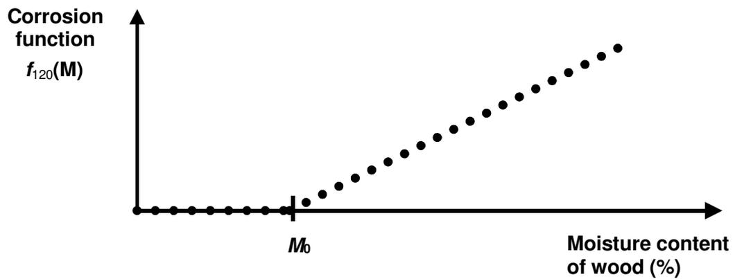
Figure C.3.2. Corrosion function  $f_{120}(M)$  for timber embedded in CCA treated wood.
