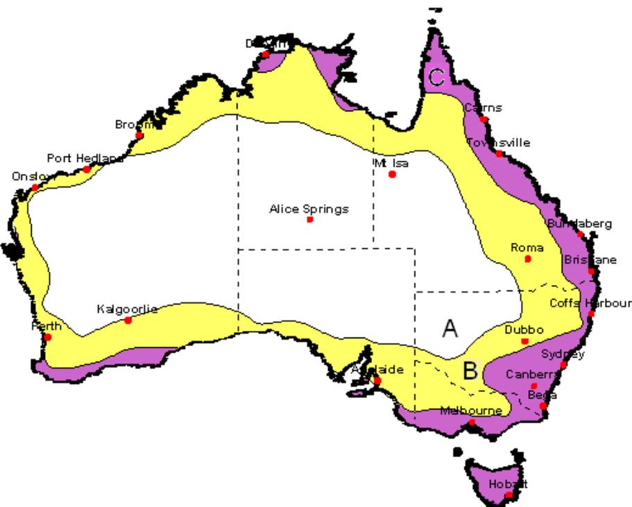
**Figure 5.2.1.1** Embedded corrosion hazard zone map. Zone C is most hazardous.
