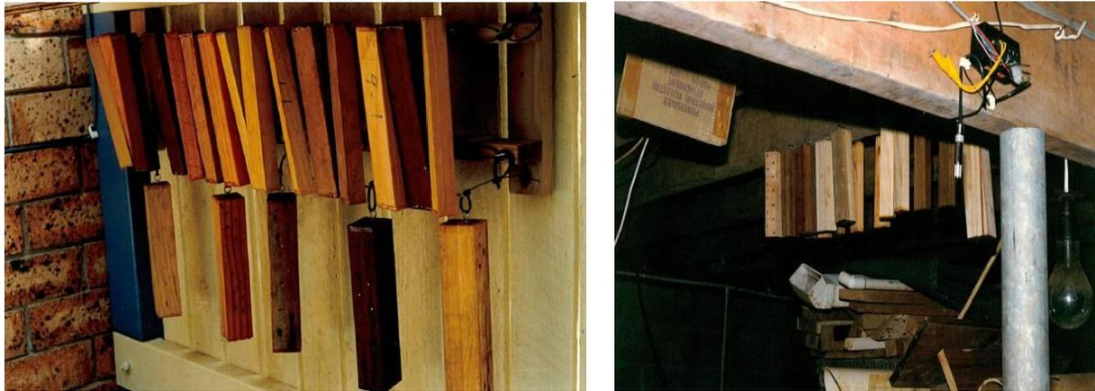
**Figure 3.1.1.** Exposed nail joint specimens on facade (left) and in subfloor (right)
