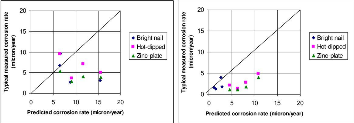
**Figure 3.1.1.1** Checks with 2-year embedded nails data outdoor using 2002’s model . Left: Marine sites, Right: Non-marine sites
