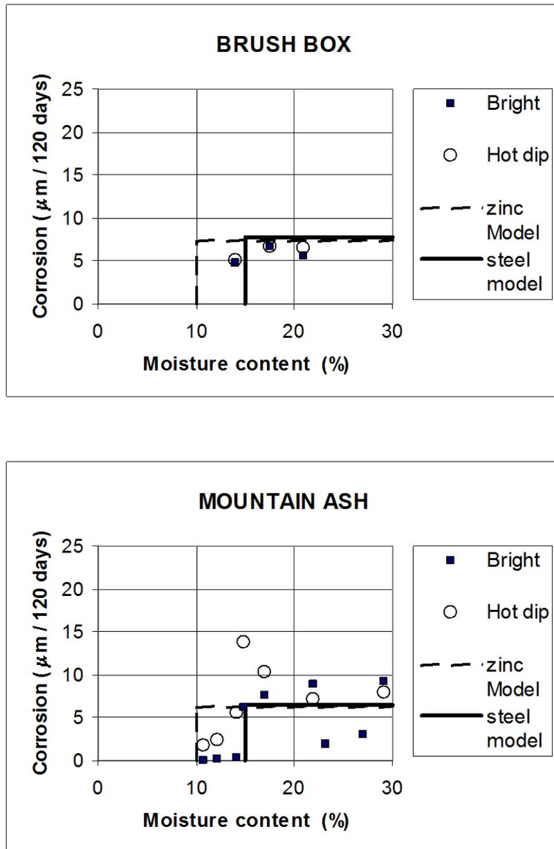
**Figure C.4.1.** Comparison of corrosion model for embedded metal, with test data for hardwoods.
