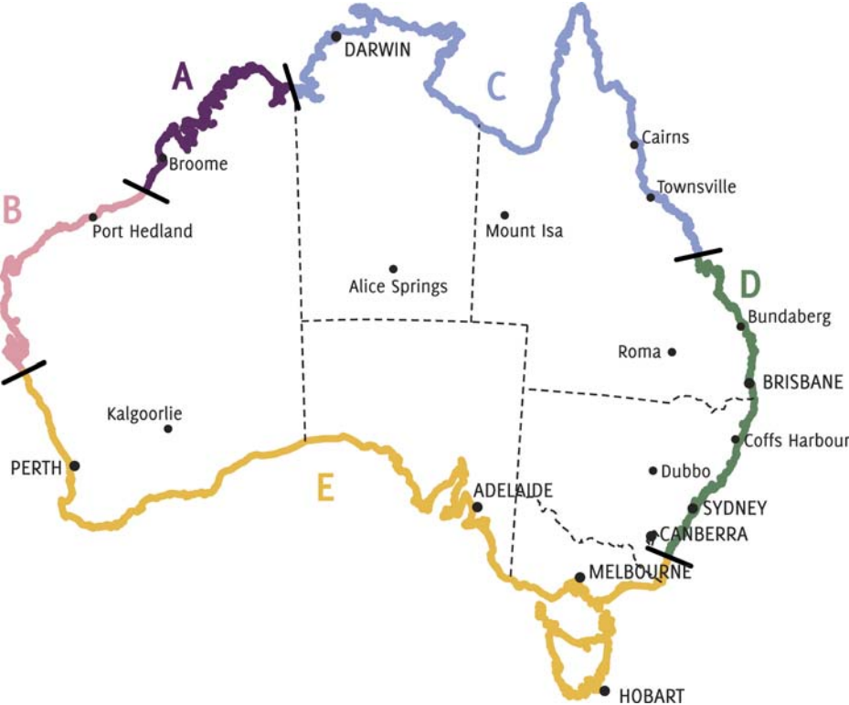
Figure 1.1.5.1. Hazard Zones related to atmospheric corrosion (Zone E has the greatest hazard)
