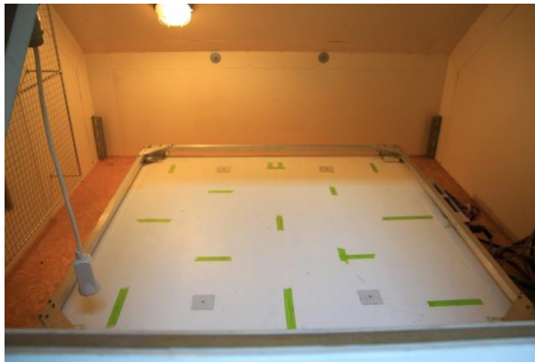
Figure 4. Metering box in upper chamber
