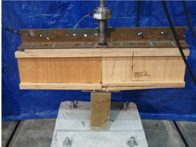
Figure 13. Joist flange delamination
