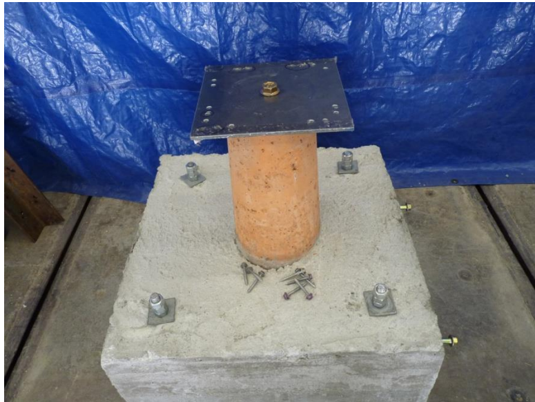
Figure 3 Concrete pile with connector plate attached
