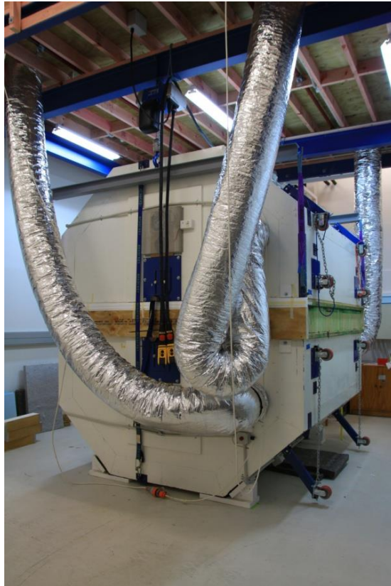
Figure 1. Guarded Hot Box with floor panel installed.
