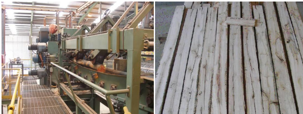
Figure 25: The HewSaw R200 at the former FEA mill site at Bell Bay, Tasmania processing E. pilularis (left) and drying defect associated with the pith in small diameter E. pilularis (right) (source: Washusen et al. 2009d).
