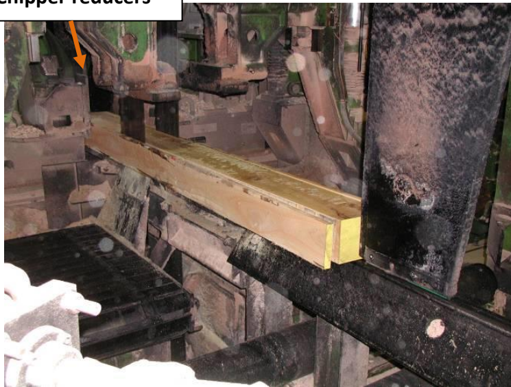
Figure 10. The McKee twin band-saw at Auswest Timbers, Pemberton, equipped with chipper reducers (in this photograph hidden ahead of the saws) that effectively make four cuts with the initial pass. This photograph was taken during a trial back-sawing pruned 22-year-old plantation-grown Eucalyptus globulus grown at Vasse in Western Australia and shows the sawing immediately after the first turn-down (source: Washusen et al. 2004)
