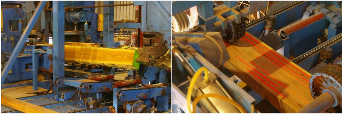
Figure 16. The sawing system at Whittakers Timber Products processing 17-year-old pruned plantation-grown eucalypts. Top: sawing on the twin band-saw; Lower left: the hydraulic turn-down device in operation; Lower right: scanning of the central cant prior to re-sawing on the multi-saw (source: Washusen et al. 2009a)
