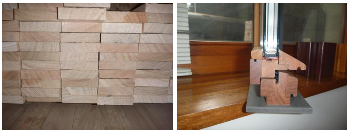
Figure 34: Quarter-sawn dried E. globulus boards at Villapol, cross-cut prior to laminating and showing no visible internal-checking (left); and cross section of moulded window frames (source: Harwood 2012).
