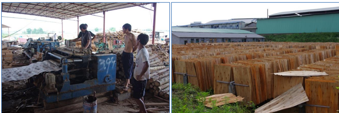
Figure 39: Processing peeled veneer from small diameter eucalypts with a spindle-less lathe (left) and air drying peeled veneer sheets at the Qi Po Veneer mill, Guangxi Province, P.R. China. (Photos: Russell Washusen).
