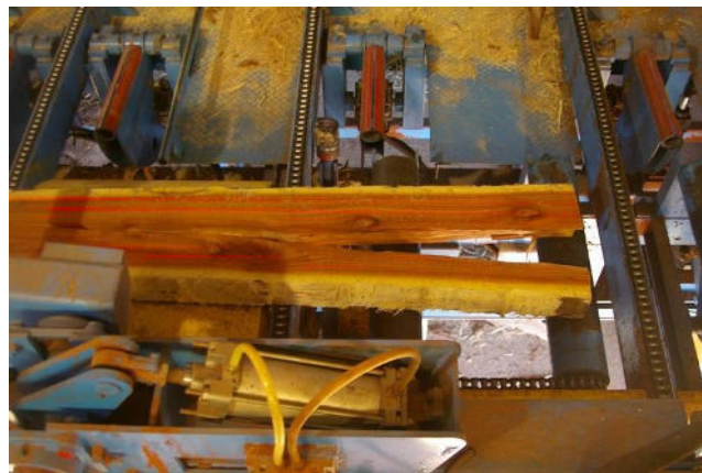
Figure 17. Log end-splitting in 17-year-old Eucalyptus saligna , the consequence of sawing to produce a cant that is too narrow relative to the log diameter (source: Washusen et al. 2009a).
