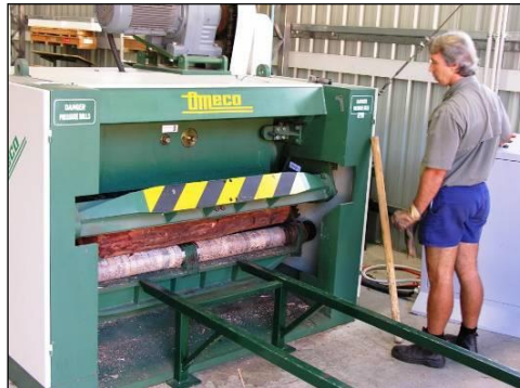
Figure 40: Processing of Corymbia citriodora subsp variegata into veneer sheets using an Omeco spindle-less lathe (source: Zbonak et al. 2012).
