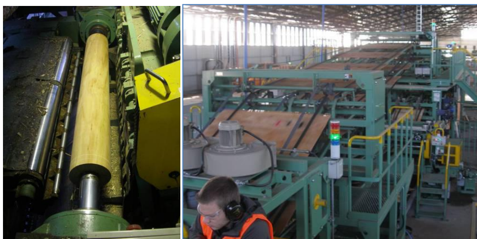
Figure 41: Lathe with partly peeled E. nitens billet (left), the veneer conveyor and veneer stacker at the Ta Ann mill, Smithton, Tasmania (right) (Source: Blakemore et al. 2010b).
