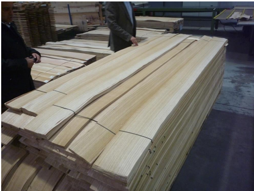
Figure 42: Quarter-sliced veneer produced at Asperal, Spain from E. globulus (Source: Harwood 2012).
