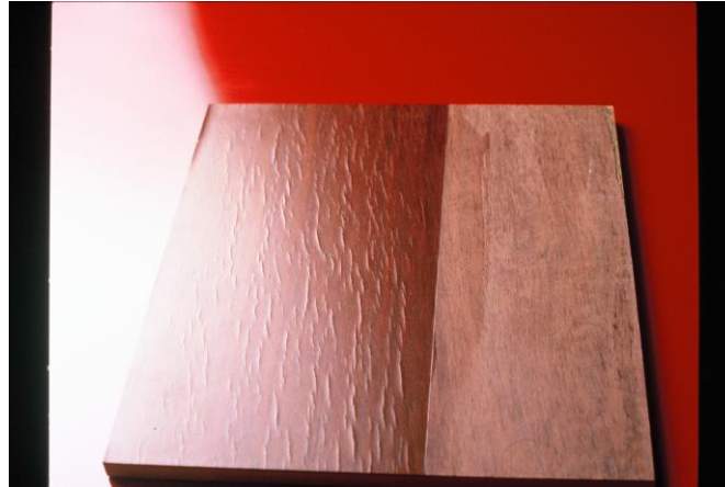
Figure 41: Example of checks developed on veneer surface (Photo: Barbara Ozarska)
