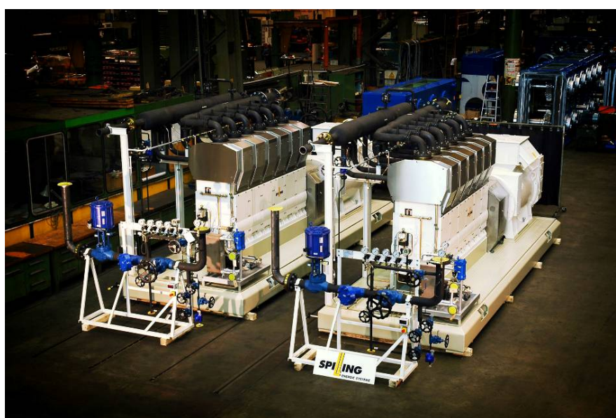
Figure 12: Two Spilling 6 - Cylinder (3/3H12) Engine Sets. 33
