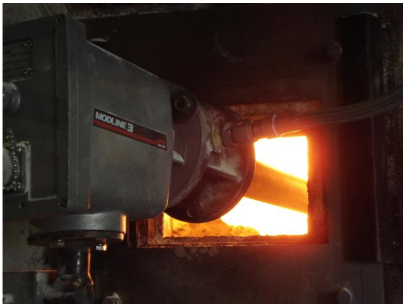
Figure 21: Canadian paper mill firing bio-oil in a lime kiln.
