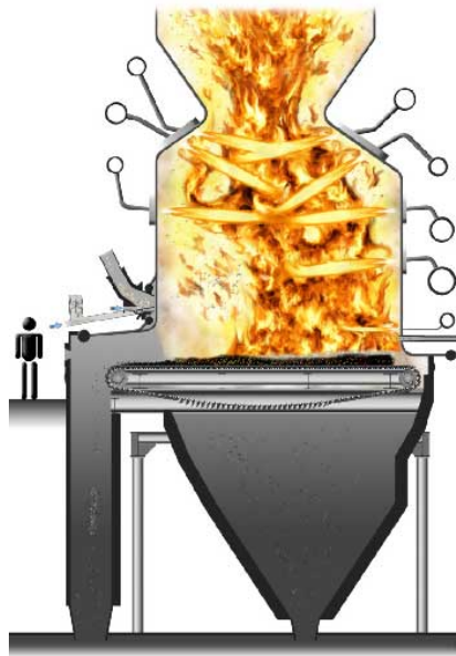
Figure 9: A travelling grate type furnace. (Image courtesy of AET-Biomass)
