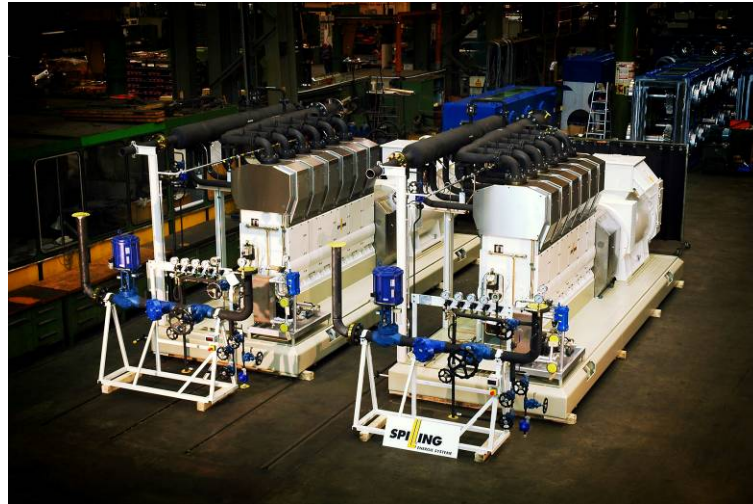
Two 6-cylinder Spilling steam engines
