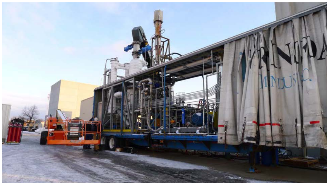
Figure 18: Trailer mounted research gasifier and GTL reactor that converts 100-150kg/hour of wet wood chips into 10-30litres/hour of bio-methanol, which is intended to be converted to electricity in a Direct Methanol Fuel Cell. (Photo courtesy EERC, University of North Dakota)
