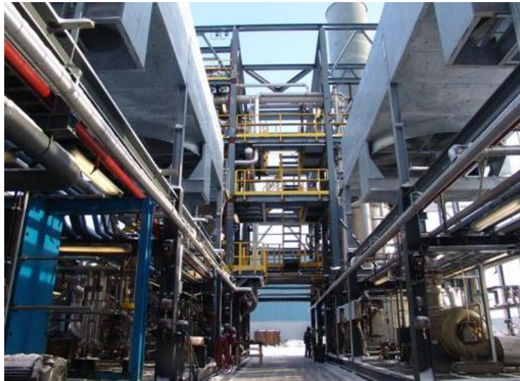
Figure 22: DynaMotive's 200 tonne per day Plant in Guelph, Ontario, has an input of approximately 65,000 dry tonnes per year of biomass from waste construction and demolition wood and produces an energy output equivalent to 130,000 barrels of oil. (Image courtesy DynaMotive)
