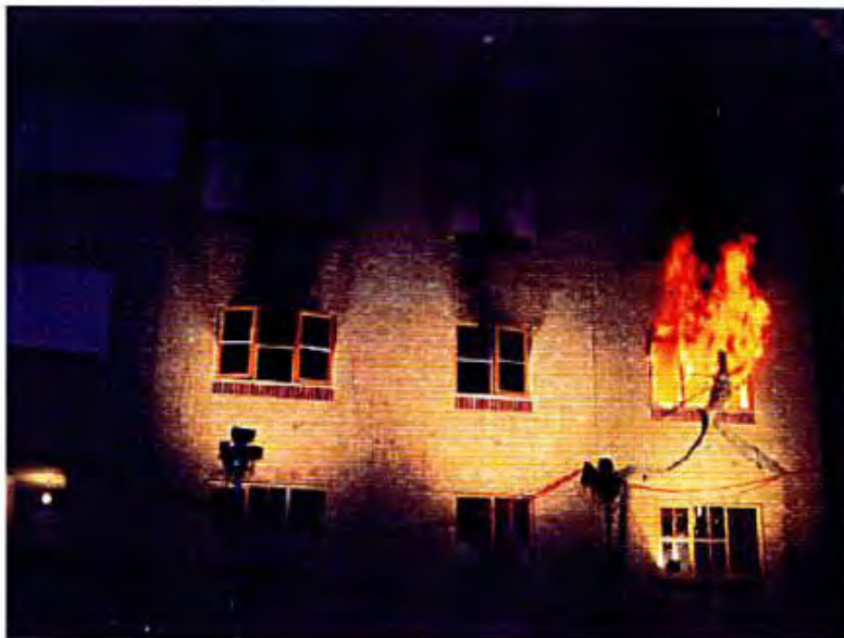
Figure 3: Front elevation of the TF2000 building. Flames can be seen emanating from the living room window of the fire flat.
