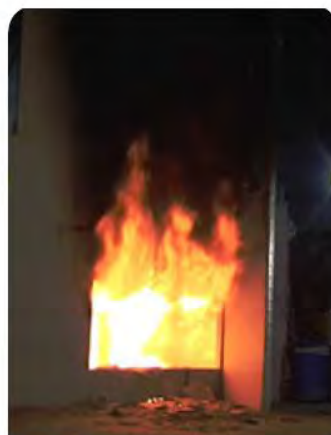
35 mins Transition to fuel controlled phase
