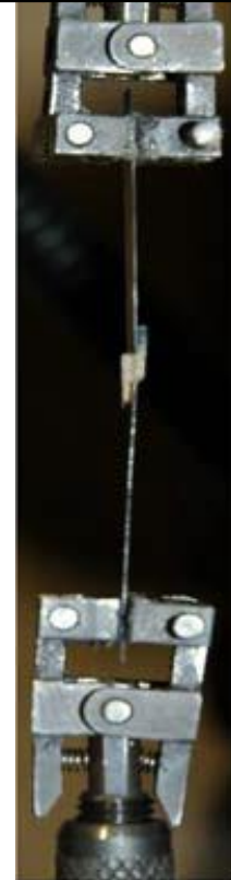
Digital image correlation: 2D strain fields in micro-bonds
