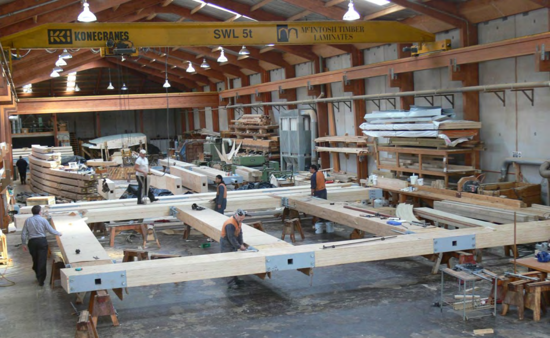
Pre assembled in factory before delivery to site.
