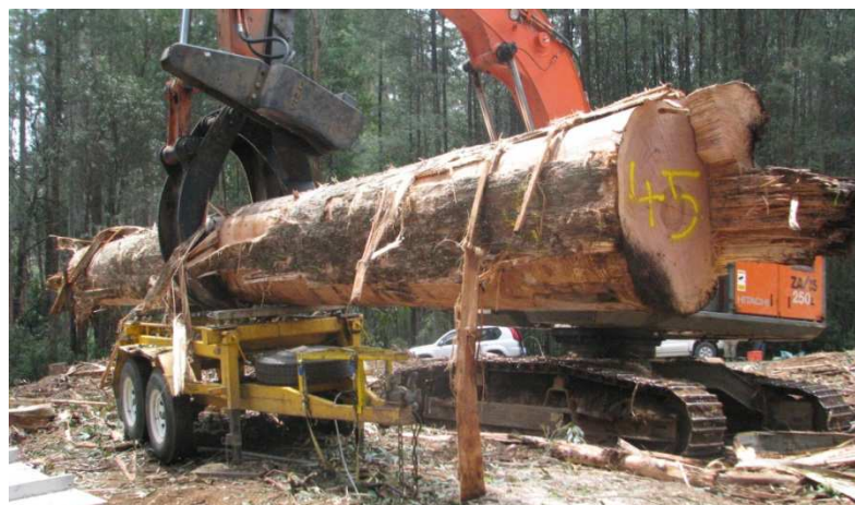
Figure 1.6. A mountain ash “production” site log being weighed on the biomass weighing trailer.
