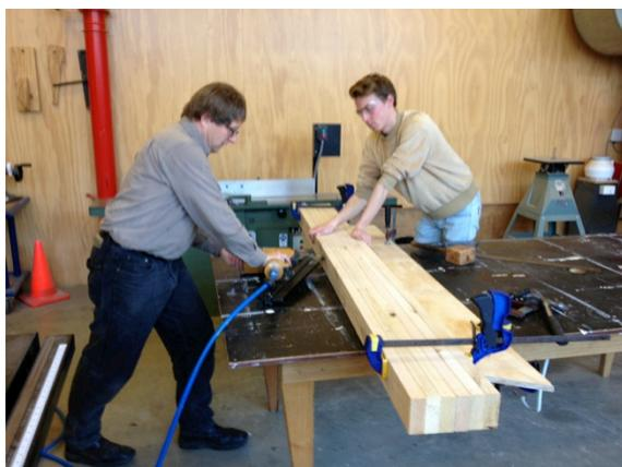
Figure 7: Nail lamination of E. Nitens 90x35 boards
