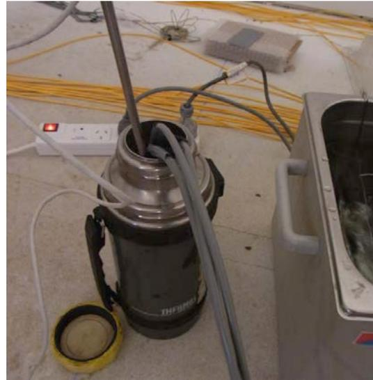
Figure 12: An ice filled thermos for cooled temperature sensor calibration
