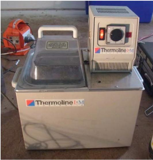
Figure 11: Thermoline calibration equipment for heated temperature sensor calibration
