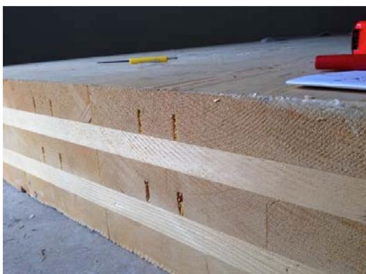
Figure 9: 180mm 5 ply softwood CLT panel
