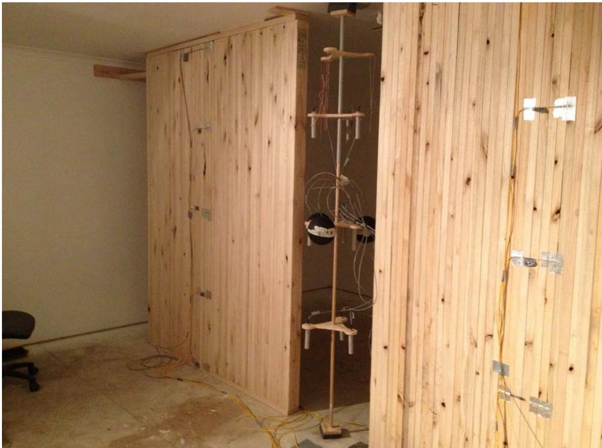
*Figure 1: 90mm plantation Eucalyptus nitens partition wall within test building*
