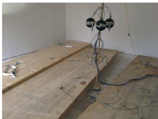
Figure 10: Three softwood CLT panels installed inside test building on top of existing particleboard floor
