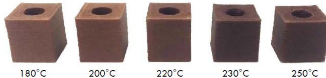
Cubes printed with LAYWOO-D3 at different temperatures
