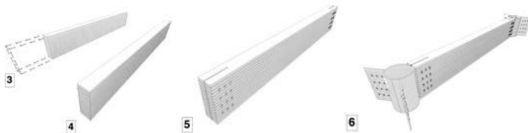
Figure 2. Sawn timber cut to length (No. 3) or engineered timber piece (No. 3 & 4). Machined piece (No. 5). Finished piece with connectors attached (No. 6).
