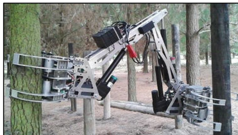
Tree-to-tree 'swinging' forest harvester (Parker et al., 2015)
