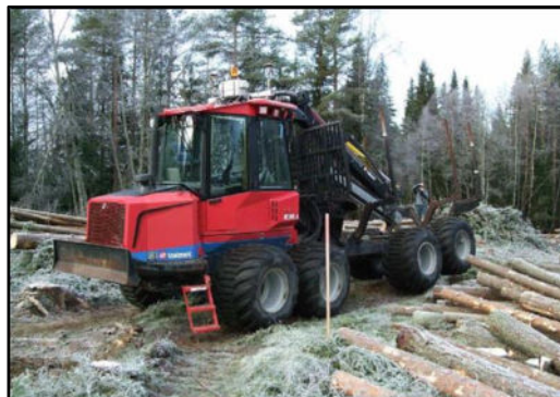
Valmet 830 forwarder tested for path detection in the forest (Image sourced from Ringdahl 2011).
