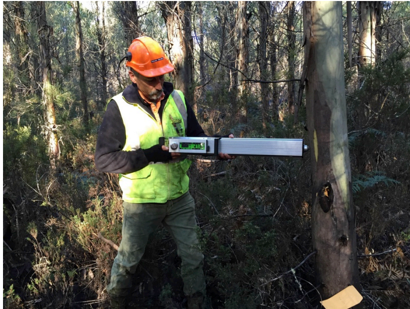
Geoff Downes operating the resistograph on E. nitens trees growing at Blythe Rd
