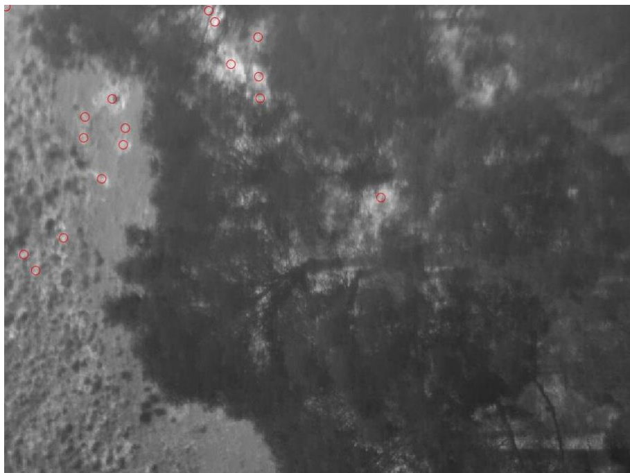
Figure 13: Example of multiple false positive detections. These detections have the same intensity (infrared radiation) as the koala detection shown above
